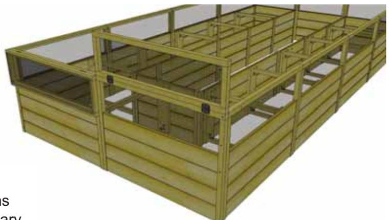
**25.** Complete attachments of both back wall trellis/screens to rear wall framing. Confirm screens can move up and down smoothly. Adjust if necessary.
