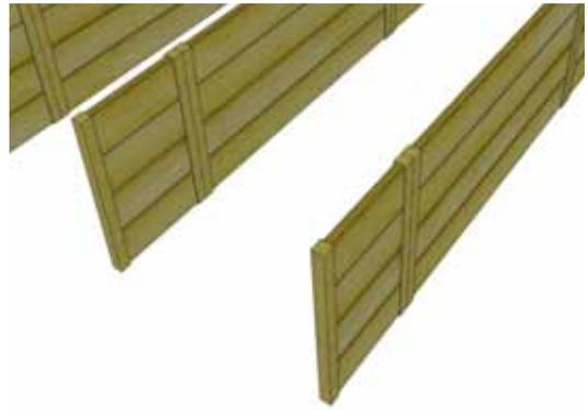
**12.** Align and attach final side **Interior Panels (Part D)** as per **Step 10**. Angle screw panels together with **3 - 2 1/2" Screws** from the inside.
