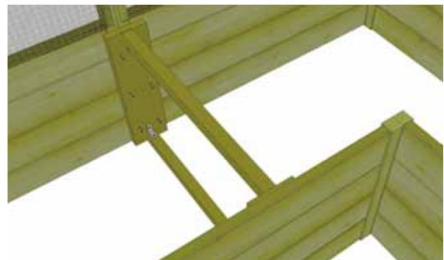
**19.** Lift and center completed longer **Bed Rib Frame** on rear and end interior panels. Align with bottom of panels. Secure with **6 - 2" Screws** per plate. **Important** - Do not over screw!
