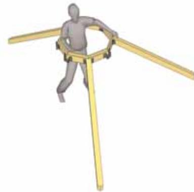
**29.** From underneath, screw bracket and corner rafter together with 2 - 3" screws. With your helper still supporting the Skybox/ Rafter Assembly, position and attach a second and third rafter as illustrated in **Step 28**.
