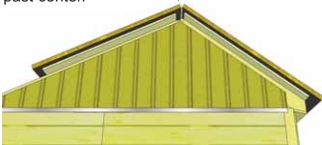
Slight Gap between Roof Panels. Long Side will sit slightly past center.
