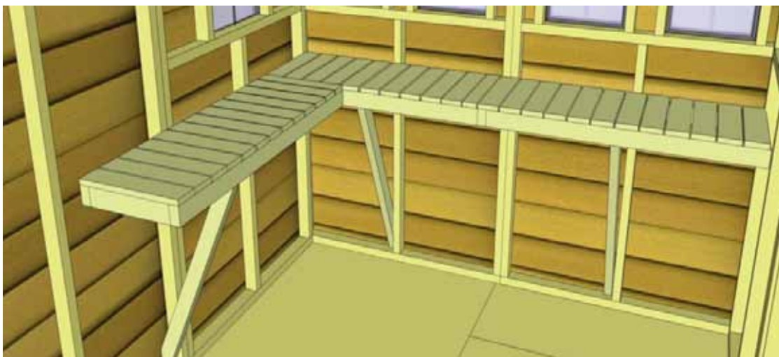
Completed Potting Shelf
