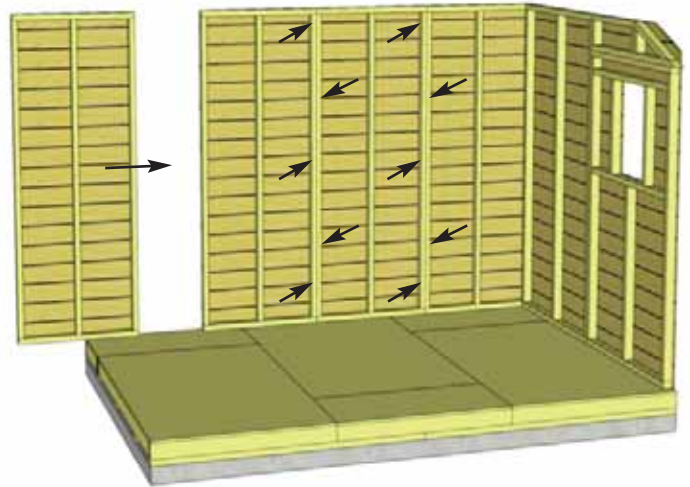
20. Position and secure Wall Panel studs together as per Step 18 .
