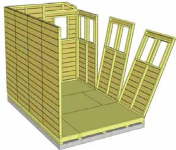
22. Position and secure Wall Panel studs together with 3 - 2 1/2" screws. Locate and position remaining Double Window Walls on floor.
