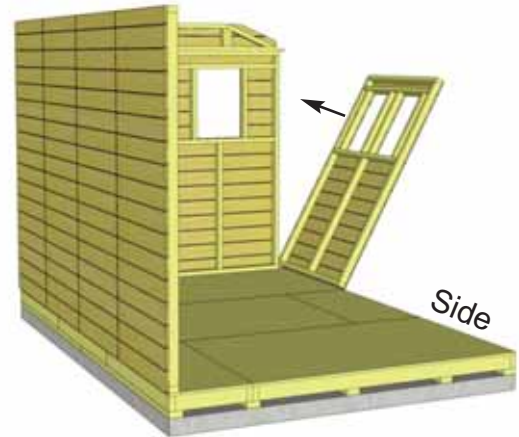
21. Front Side Wall Panel will sit flush with floor framing in corner when positioned correctly. Position Right Side Double Window Wall on floor.
