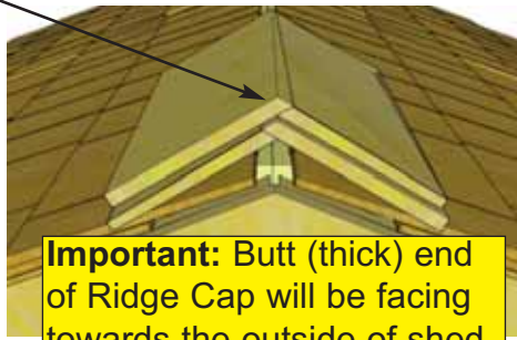
Alternate Ridge Cap seams (offsetting angle cut at peak)
