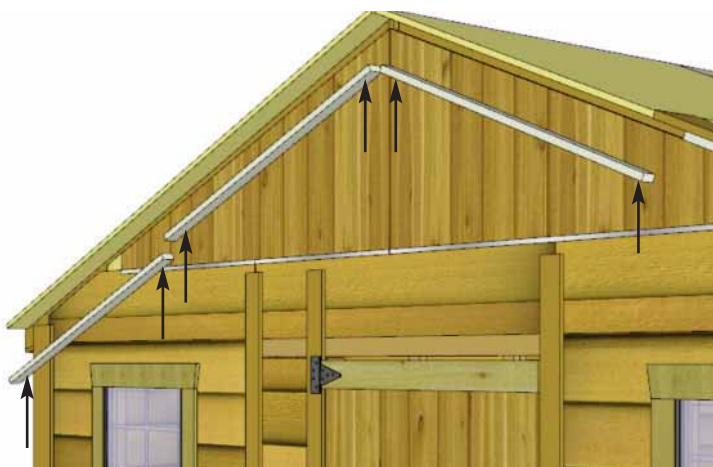
78. Attach Facia Cleat (3/4" x 1 1/2" x 36 1/2") centered on underside of Short Roof plywood, flush to edge. Attach Facia Cleats (3/4" x 1 1/2" x 40") to underside of Long Roof plywood, 1/2" from ends and flush to edge. Repeat this step on the rear side of shed. Fasten with 3 - 1 1/4" screws per piece.
