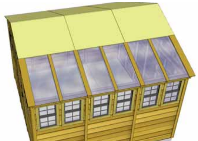
77. Align and attach remaining Ridge Caps (4 1/2" wide) over Double Rafters as per Step 74.
