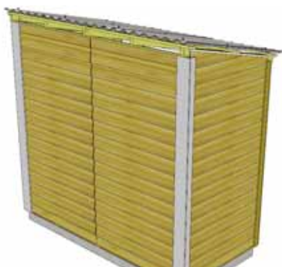
60. To completely trim out rear corners, locate Side Rear Corner Trims (1/2" x 2 1/2" x 88 3/4") and Rear Corner Trims (1/2" x 5 1/2" x 88 3/4"). Align and attach as per Step 59.
