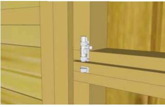
88. Attach Door Handle, Exterior Drop Latch and Interior Barrel Bolt to door. Handle is positioned on top door, Drop Latch on bottom door, and Interior Barrel Bolt (silver) on top door stud. Attach Black Drop Latch as illustrated above with 4 - 3/4" Black Screws. Note how female part of Drop Latch is positioned higher than male part. Do a dry run first to position Drop Latch correctly. Important: Drill pilot holes with 1/8" drill bit prior to securing to prevent wood from splitting.
