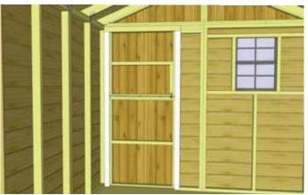
**89.** Attach Horizontal Door Stop and Vertical Door Stops to door jamb and wall framing. Use 4 - 2" screws to secure Horizontal Stop, and 6 - 2" screws per Vertical Stop. Door Stops should overhang the door by approximately 1/2". Start with the Horizontal Stop first.
