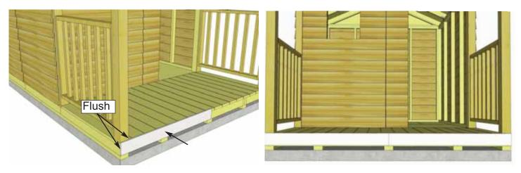
**59.** Attach **Front Bottom Skirting** around the base of the shed. Skirting will hide floor framing. Start with Front Skirting positioned flush with the top of the deck boards and the side of the floor frame. Attach with **6 - 1 1/2" Finishing Nails** per piece.
