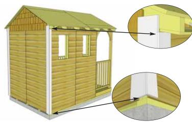
64. Position Corner Trim in rear corner and Wide Corner Trim over Filler Trim. Prior to attaching, do a dry run with Narrow Trim butted up tight underneath the Soffit. Position Wide Trim evenly with Narrow Trim at bottom Narrow Trim will cap Wide Trim. Attach with 8 - 1 1/2" Finishing Nails per (1/2" x 5 1/2" x 81 1/2") x 2 piece. Repeat for other opposite rear corner.
