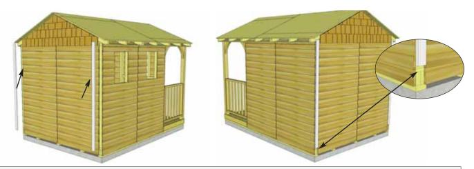
**63.** Attach Rear Filler Trims to rear walls, positioned flush with siding and bottom skirting. Attach with 8 - 1 1/2" Finishing Nails.
