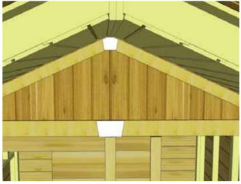
**70.** Position Small Porch Detail Plate and one Facia Detail Plate to cover trim seams. Attach with 4 - 1 1/2" Finishing Nails per piece.
