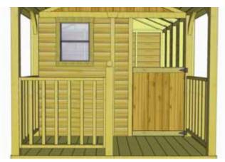
**86.** Place **Bottom Dutch Door** panel into position. Gap 3/8" on bottom, evenly space on sides, and attach hinge to doorway seam trim with **3 - 2" Black Headed Screws**. Use shim to help keep the door evenly spaced on bottom. One of the **Shim Shingles** can be used.
