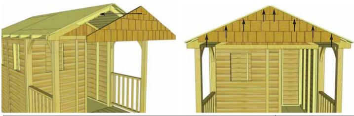
**74.** Position the **Gusset Gable** onto the front of the shed. Push Gable plywood up tight under roof plywood and against Roof Nailing Strip. Screw through the shingles of the Gusset Gable horizontally into the Roof Nailing Strip with 8 - 2 1/2" screws.
