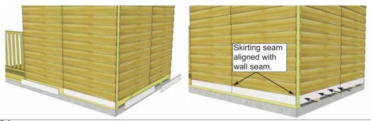
**61.** Position **Rear Bottom Skirting - Bevel** around the base of the shed. Bevel is thicker at butt and thinner at top of board. Skirting will hide floor framing. Gaps on side will be covered by Narrow & Wide Trimpieces later. Start on side walls first and attach with **4 - 1 1/2" Finishing Nails** per piece.
