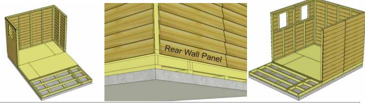
**16.** Be sure to correctly position wall panels so siding overhangs your floor and wall framing is flush with floor framing. Continue to attach walls together as per **Step 15.**
