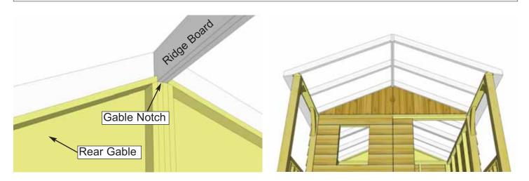
**44.** When both **Rafter** Sections are correctly aligned, **Ridge Boards** will sit in both the rear and middle gable notches. Front **Rafters** will overhang **Porch Posts**.
