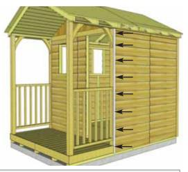
65. Position Narrow Filler Trims in gap between shed and porch. Attach with 8 - 1 1/2" Finishing Nails per piece.
