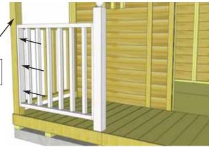
**80.** To complete porch, attach **Short Deck Post** and **Handrail Section** together with **3 - 2" Screws**. Measure 3 1/2" from bottom of post to align rail. Place Post/Handrail section on deck. Attach rail to Porch Post with **3 - 2" Screws**.
