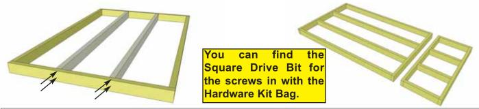
2. When correctly positioned, attach each Joist with 4 - 2 1/2" screws (2 per end). You can find the Square Drive Screw Bit in the Hardware Kit Bag.
