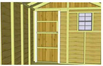
**100.** Attach Horizontal Door Stop and Vertical Door Stops to door jamb and wall framing. Use 4 - 2" screws to secure Horizontal Stop, and 6 - 2" screws per Vertical Stop. Door Stops should overhang the door by approximately 1/2". Start with the Horizontal Stop first.
