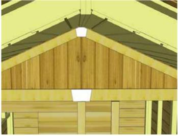
**81.** Position Small Porch Detail Plate and one Facia Detail Plate to cover trim seams. Attach with 4 - 1 1/2" Finishing Nails per piece.
