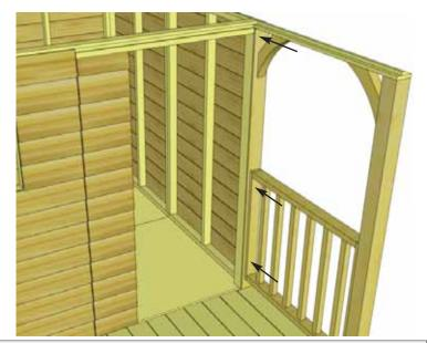
28. Attach Wall Trim/Supports to wall with 3 - 2 1/2" screws per side. Try to conceal screws if possible.
