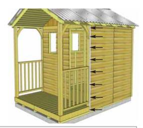
76. Position Narrow Filler Trims in gap between shed and porch. Attach with 8 - 1 1/2" Finishing Nails per piece.
