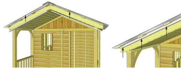
**83.** Attach remaining two **Roof Nailing Strips** to the underside of the roof plywood on front of shed. These strips will be pushed tight against the rafters unlike the Rear Nailing Strips. Fasten with **4 - 1 1/4" Screws** per piece.
