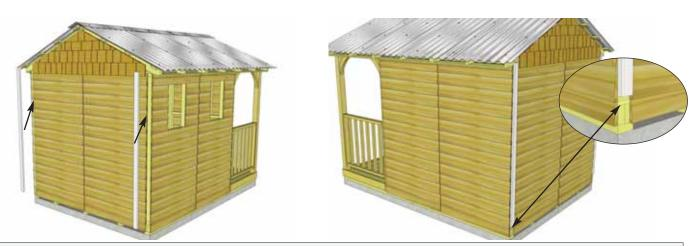
**74.** Attach **Rear Filler Trims** to rear walls, positioned flush with siding and bottom skirting. Attach with 8 - 1 1/2" **Finishing Nails**.
