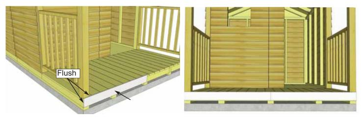
**70.** Attach **Front Bottom Skirting** around the base of the shed. Skirting will hide floor framing. Start with Front Skirting positioned flush with the top of the deck boards and the side of the floor frame. Attach with **6 - 1 1/2" Finishing Nails** per piece.
