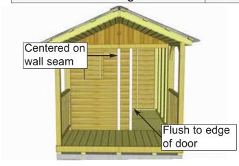
**79.** Attach both Porch & Door Trims to front walls. Secure with **6 - 1 1/2" Finishing Nails**.
