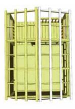
**57.** Repeat **Steps 51 - 56** to complete Batten Section on opposite side of roof with remaining **Battens** and **Batten Spacers**.
