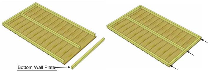
**13.** Starting with All **Solid Wall Panels**, carefully lay panel face down. Position and attach **Bottom Wall Plates** to bottom of wall studs of each wall panel with **3 - 2 1/2" screws**. Position so Wall Plates are flush with framing.
