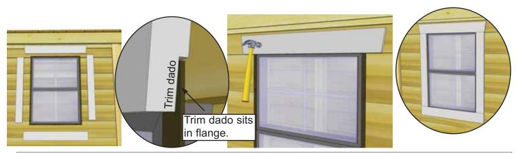
**95.** Position **Window Trim** around window doing a dry run first and attach with **4 - 1 1/2**" **Finishing Nails** per piece. Window trim has a small dado on reverse face. Outside flange of window will roughly sit in the dado to give a better fit.
