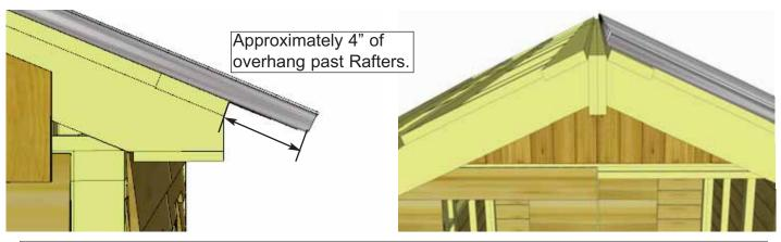
**59.** Overhang the **Metal Roof Panels** past the **Battens** on front and rear of shed by approximately 1". Adjust panels side-to-side to achieve desired width. Overall width past the **Battens** can vary from 1" - 3" depending on your preference. The overhang over the side of the shed will be set by the **Metal Roof Hangars**, but should be approximately 4" on side of shed.
