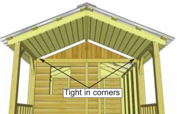
**80.** Position **Porch Roof Seam Trim** so the sharp angle of each piece is tight into the corner between Porch Ceiling and Horizontal Above Door Trim. Attach with **4 - 1 1/2**" **Finishing Nails** per piece.
