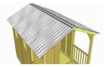
**65.** Locate remaining **Foam Enclosures**. Place **Foam Enclosures** at the top of roof panels. **Foam Enclosures** prevent moisture from coming in through the top of your shed.
