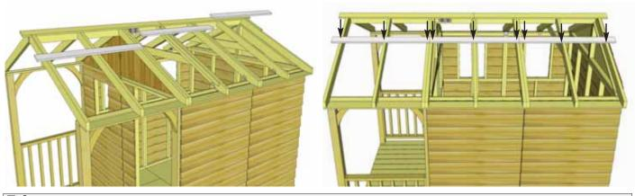
**54.** Locate **2 Outside Roof Battens** and **1 Inside Roof Batten**. Place outside Battens flush with Batten Spacers and overhanging outside Rafter by 3 3/4". Secure row of Battens to Rafters with **9 - 1 1/4**" **screws** (3 screws per Batten).
