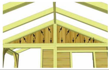
47. With both Ridge Boards connected, completely secure Rafters to Front Gable framing of both rear and middle Gable Walls. Use 8 - 2" screws.
