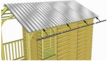
**62.** Before fully fastening **Metal Roof Panels** down, remove the **Metal Roof Hangars** and insert **Foam Enclosures** between **Metal Roof Panels** and **Battens** at the bottom of the roof. Enclosures will prevent moisture and unwanted bugs, etc from entering your shed through here.
