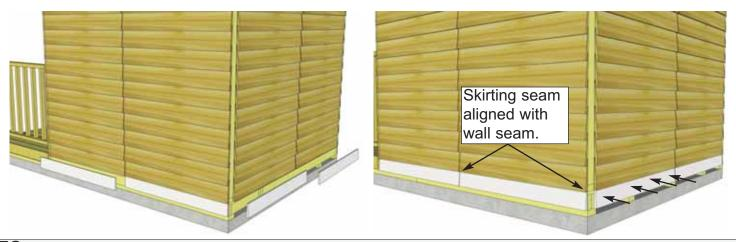
**72.** Position **Rear Bottom Skirting - Bevel** around the base of the shed. Bevel is thicker at butt and thinner at top of board. Skirting will hide floor framing. Gaps on side will be covered by Narrow & Wide Trimpieces later. Start on side walls first and attach with **4 - 1 1/2" Finishing Nails** per piece.
