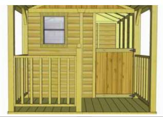
**97.** Place **Bottom Dutch Door** panel into position. Gap 3/8" on bottom, evenly space on sides, and attach hinge to doorway seam trim with **3 - 2" Black Headed Screws**. Use shim to help keep the door evenly spaced on bottom. One of the **Shim Shingles** can be used.
