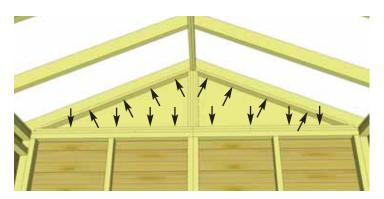
**46.** With both Ridge Boards connected, completely secure Rafters to Rear Gable framing of both rear and middle Gable Walls. Use 8 - 2" screws.
