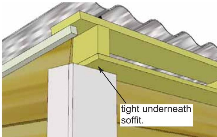
59. Place both trims in front corner and align as illustrated above. Do a dry run prior to attaching to achieve best fit. Start with 5 1/2" wide Front Corner Trim and align tight underneath soffit to determine vertical height. Attach with 8 - 1 1/2" finishing nails per piece. Position and attach Side Front Corner Trim (2 1/2" wide) using 8 - 1 1/2" finishing nails, aligning at bottom with wide trim.
