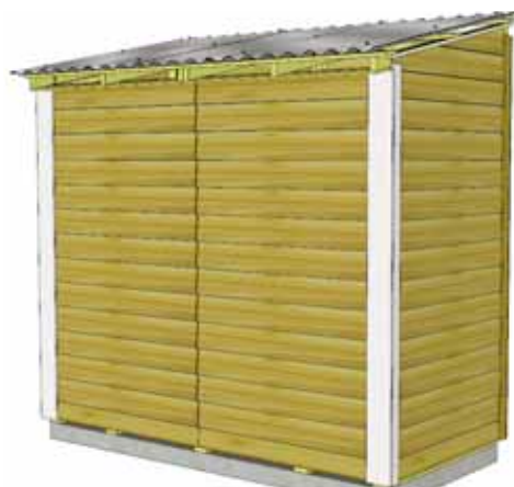
60. To completely trim out rear corners, locate Side Rear Corner Trims (1/2" x 2 1/2" x 80") and Rear Corner Trims (1/2" x 5 1/2" x 79"). Align and attach as per Step 59.
