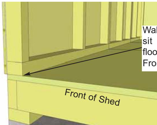
Wall panel will sit flush with floor framing at Front of shed.
