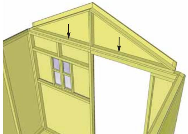
**34.** Complete positioning and attachment of front gable as per **Step 32-33.**
