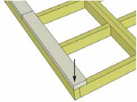
**8.** Make sure Runners are flush with outside and front and rear floor framing but not overhanging.
