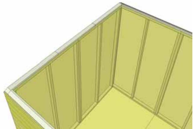
**30.** Position the **Rear Top Plates** on back wall to complete as per **Step 28**. Use 4 - 2" screws per piece.
