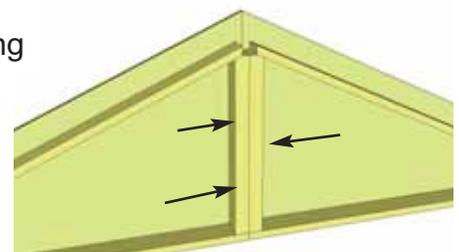
**31.** Locate **Gable 1/2 Walls** for both sides of the shed. Align framing and wall lapp siding together. Screw center wall framing of each piece together with 3 - 2 1/2" screws.
