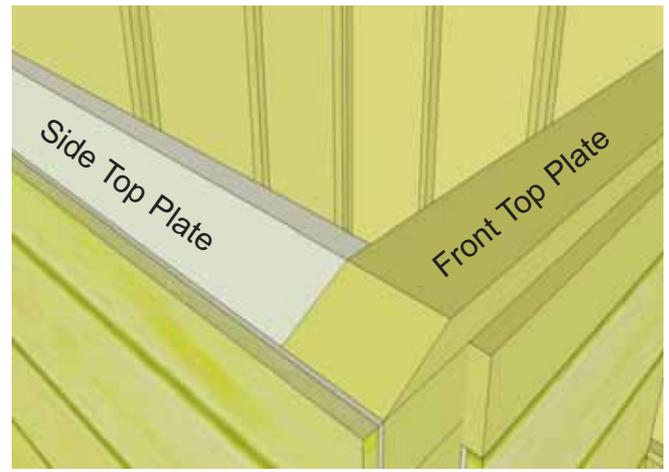
**29.** Next, attach the 2 **Side Top Plates** (1 per side). The side top plates are angle cut down the Edge. Once again, position top plate on wall plate so it is flush with inside of wall framing. Side plate should also be flush with Front Top Plate. Secure with 4 - 2" screws per piece.
