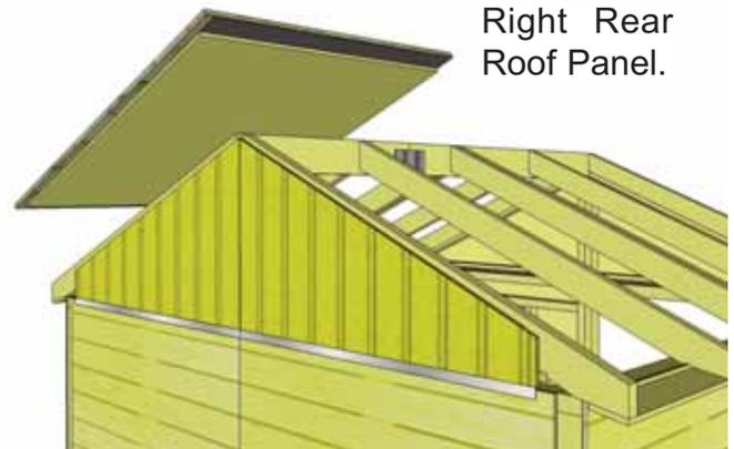
**47.** Identify Roof Panels. There are 2 Rear and 2 Front Roof Panels. Starting with a **Right Rear Roof Panel**, lift up and place on rafters.
