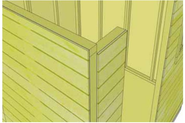
**24.** Position and attach **Narrow Wall Panel** to left side wall stud with 3 - 2 1/2" screws as per **Step 17.** **Note:** Narrow Wall is 73" high (2" shorter than wide walls). Siding overhangs adjacent wall stud and floor.
