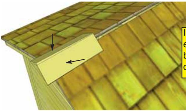
**Important:** Butt (thick) end of Ridge Cap will be facing towards the outside of shed.
