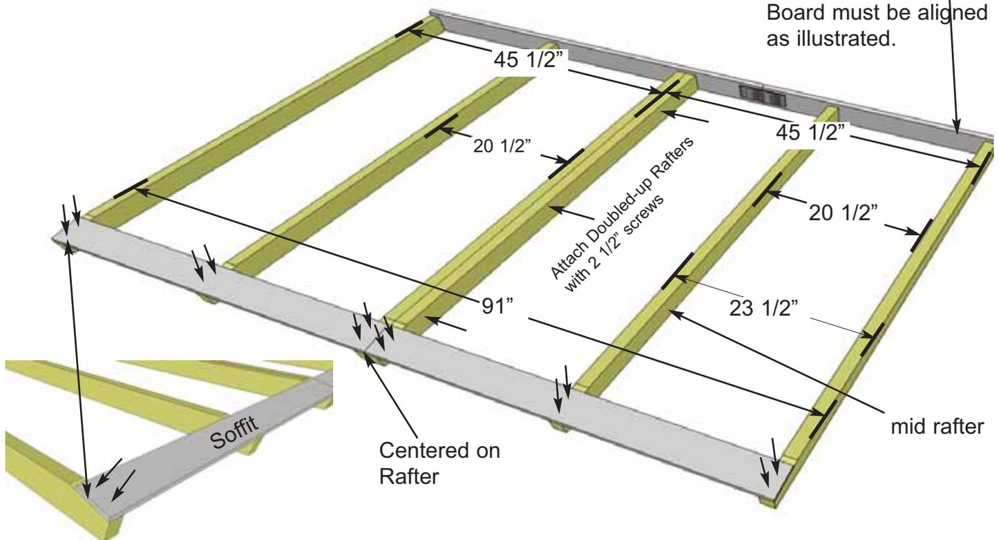
**38.** Measure, position and attach mid rafters as illustrated above as per **Step 36**.
