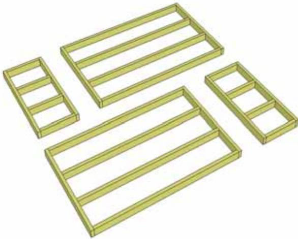
**3.** Lay out **Floor Joist Frames** as illustrated at left. There are 2 larger and 2 smaller Frame Sections. The Footprint for the floor when attached together will be 96" wide x 91" deep.
