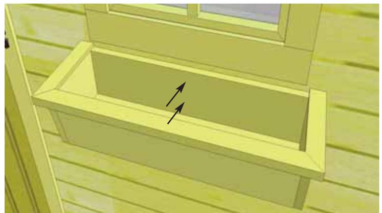
**74.** Assemble **Flower Box** with Assembly Instructions included. Position completed Flower Box below bottom of window trim and secure with 2 - 2" screws. Screw from inside of box into the center wall stud. Attach second screw 2" underneath first screw and once again into the wall stud.
