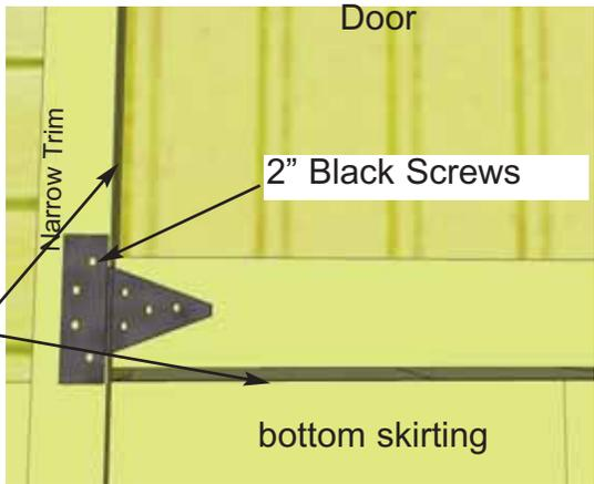
**70.** Place Door panel into position, gap 3/8" on bottom and evenly spaced on sides and attach hinges to Narrow Trim with 1 1/2" black screws. Use shim to help keep the door evenly spaced on bottom. See **Step 71** for gap at top.
