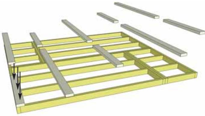
**7.** Attach **Floor Runners** to completed floor frame. There are 2 floor runners per 91" side and 5 completed runners in total. Use 3 - 2 1/2" screws per Runner.
