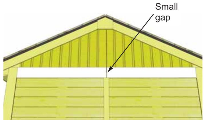
**65.** Attach **Horizontal Gable Trim** (4 - 1/2" x 4 1/2" x 44 1/2") to Front and Rear of shed. Position so flush with top and edge of wide trim. Use 4 - 1 1/2" finishing nails per piece to secure (2 pieces per side).
