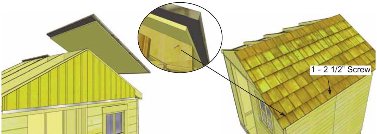
**49.** Locate **Right Front Roof Panel** (roof plywood flush with shingles on inside, shingles overhanging plywood on outside) and place on rafters. Align panels as per **Step 48** and screw panel down to rafter with 1 - 2 1/2" screw in the bottom row of shingles. Angle a 2 1/2" screw from outside rafter into roof plywood.
