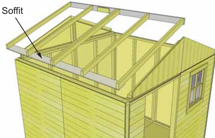
**39.** Flip Rafter Section over so Soffit is facing down. Starting with the left side, lift completed rafter section up and place on gable framing.
