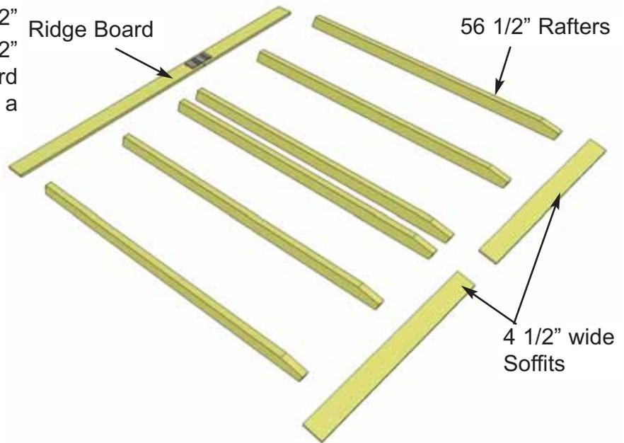
**37.** Attach end of a 45 1/2" long Soffit Board flush to ends of outside rafter with 2 - 1 1/4" screws per rafter end. **Drill pilot hole in Soffit ends to prevent splitting.** Attach Ridge Board to opposite rafter end aligning to bottom of rafter with 2 - 2" screws. Center Soffit on Doubled-up Rafters and secure with 2 - 2" screws. Measure 45 1/2" from outside rafter and secure Ridge Board to rafter with 2 - 2" screws. Attach Doubled-up Rafters together with 3 - 2 1/2" screws.
