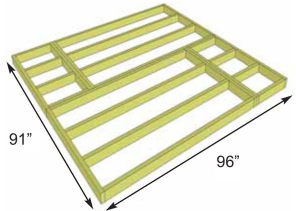
**5.** Complete all large and small frame attachments. Screw each completed section together with 8 - 2 1/2" screws.
