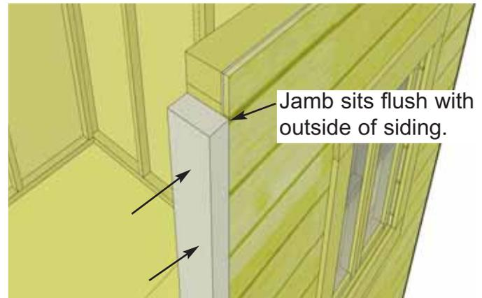
**25.** Locate **Vertical Door Jamb** and position flush against right wall panel stud. The Jamb is 3" wide and will sit flush to outside of wall siding. When positioned correctly, secure Jamb using 4 - 2 1/2" screws.
