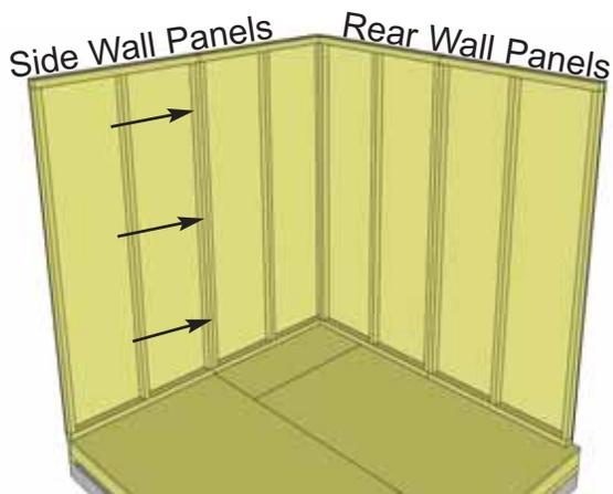
**19.** Continue positioning and securing wall panels around your floor. Attach wall studs together as per **Step 17**. Be sure that rear wall panels fit between the side wall panels (sandwiched).
