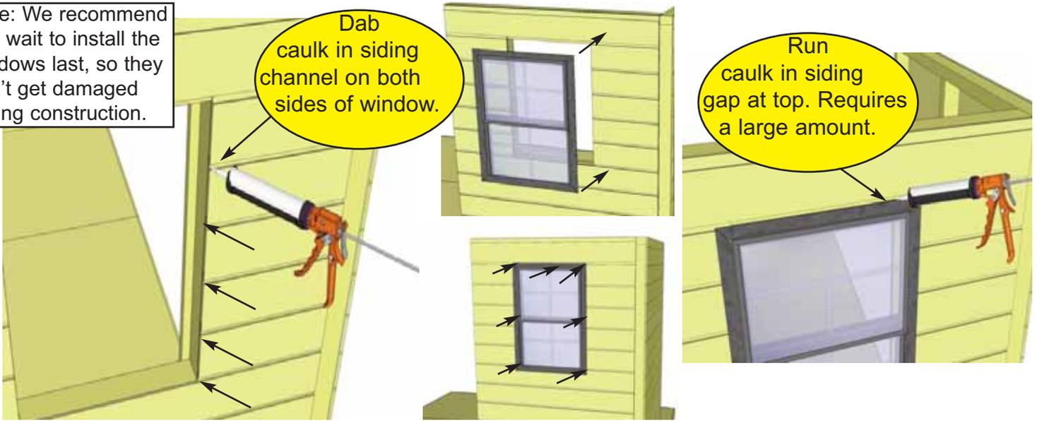
**21. Locate Window Inserts for Regular Window Walls.** Before installing, dab caulk in siding channel on both sides of window opening. This will prevent water from getting in behind window. Position window in cavity and secure with 8 - 1 1/4" screws. Caulk gap between siding and window at top. This requires a large amount of caulking but is important to fill. Later, Window Trims will be installed to hide caulking.
