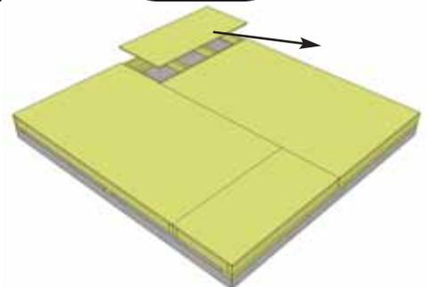
**11.** Position **Plywood Floor** pieces (4) on top of completed floor joists. Plywood is cut slightly smaller than floor framing. Keep plywood seams tight.
