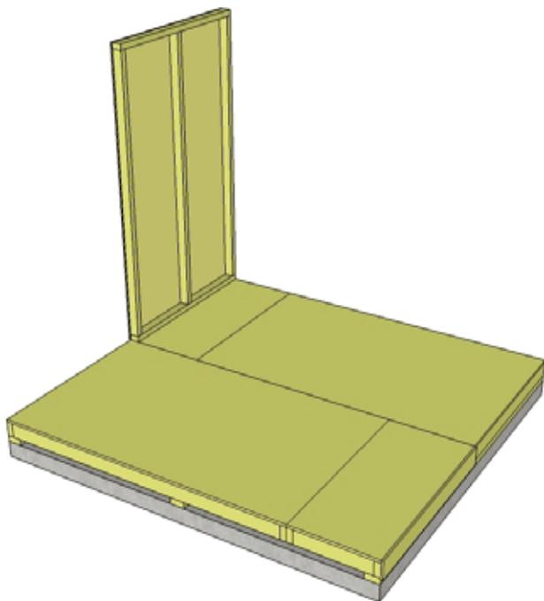
**Important:** Make sure all walls are aligned in their upright position. If not, water may leak into your shed. Unsure if panel is facing up or down? check siding on window wall panel to match alignment.
