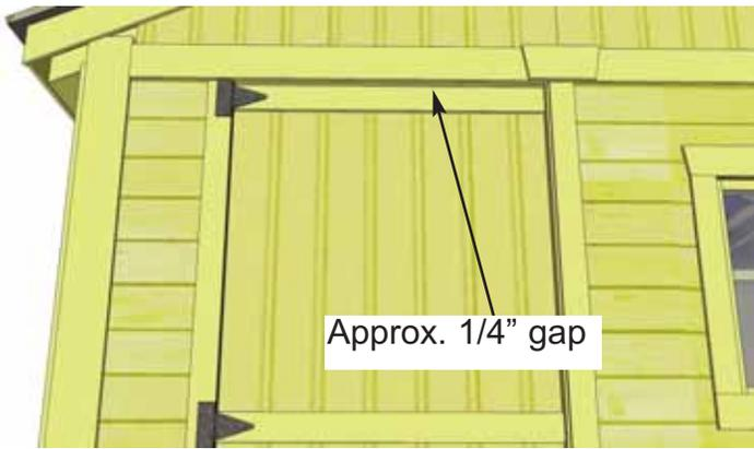
**71.** Door Panel should be positioned so there is 1/4" gap at top. Use a shim once again to help you position door correctly. Attach top and middle hinge to narrow trim with hinge hardware provided.
