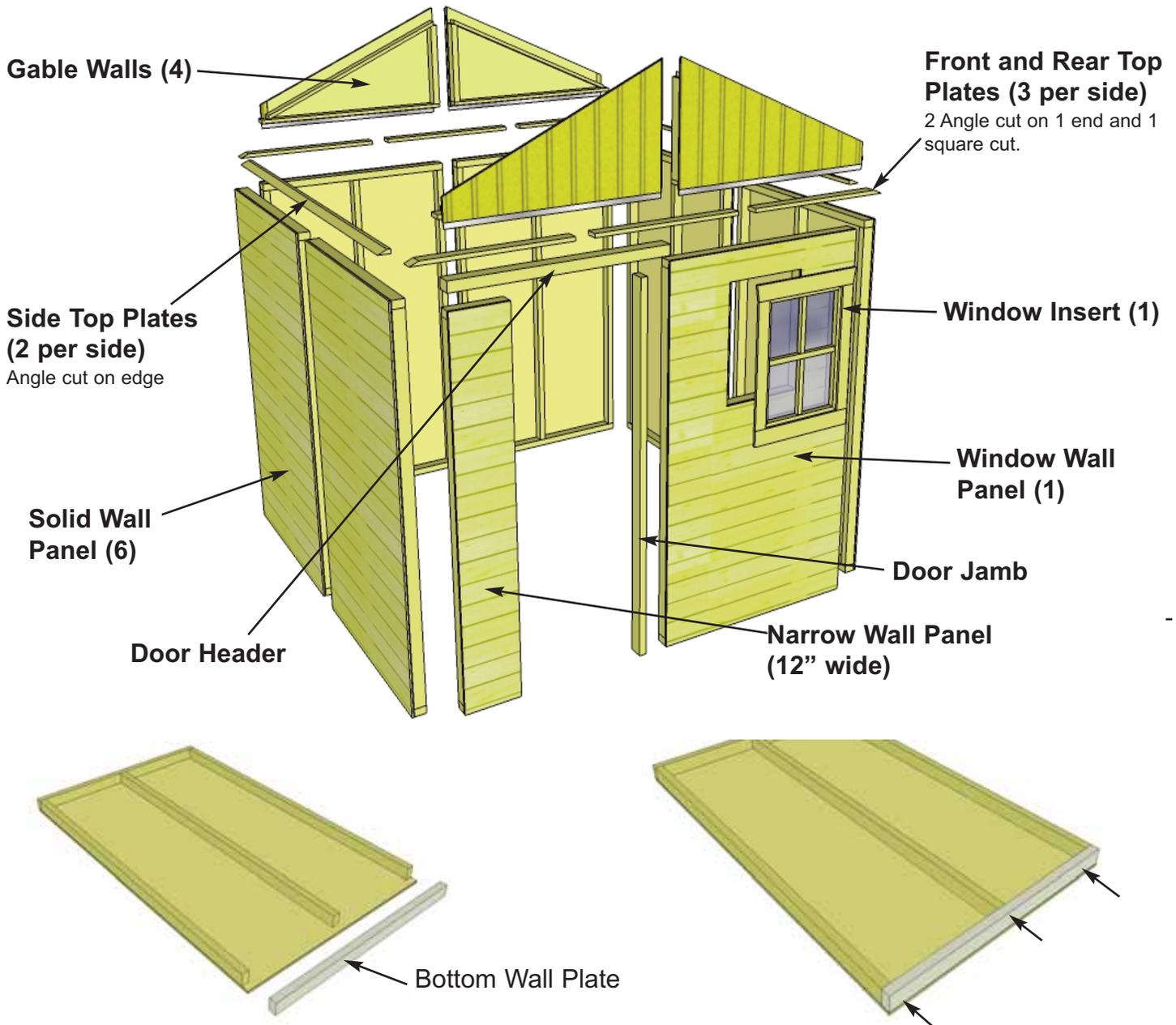
**13.** Starting with **Solid Wall Panels**, carefully lay panel face down. Position and attach **Wall Plate** to bottom of wall studs of each wall panel with 3 - 2 1/2" screws. Position so plates are flush with framing. **Note:** some Bottom Wall Plates may already be attached to some Solid Walls.
