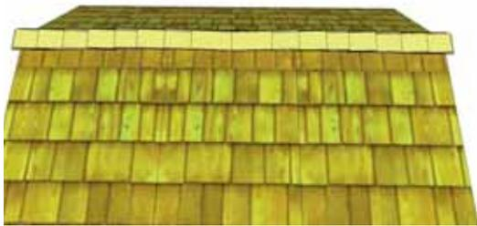
**68.** Place 3rd Ridge Cap 8" back from 2nd (enough to cover shingle nails). Attach 3rd Ridge Cap down as per **Step 67**. Continue to position and attach Ridge Caps until half roof is complete. From opposite side, position and attach Ridge Caps as described above. Score/cut 1 Ridge Cap to 12" or to fit in the center of roof. Attach center cap with 4 - 1 1/2" Shingle Nails.
