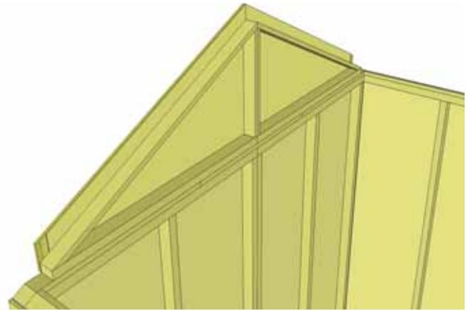
**32.** Lift up a completed gable section and place on top of Rear Top Plate on wall. The rear gable framing should sit flush with the inside of the top plate.
