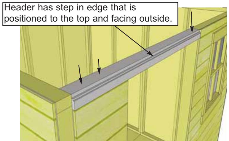
**26.** Position and attach the **Door Header** to Door Jamb and Narrow Wall Panel top framing. Header should sit flush with Door Jamb and Outside of Narrow Wall Panel Siding. Attach with 4 - 2 1/2" screws.
