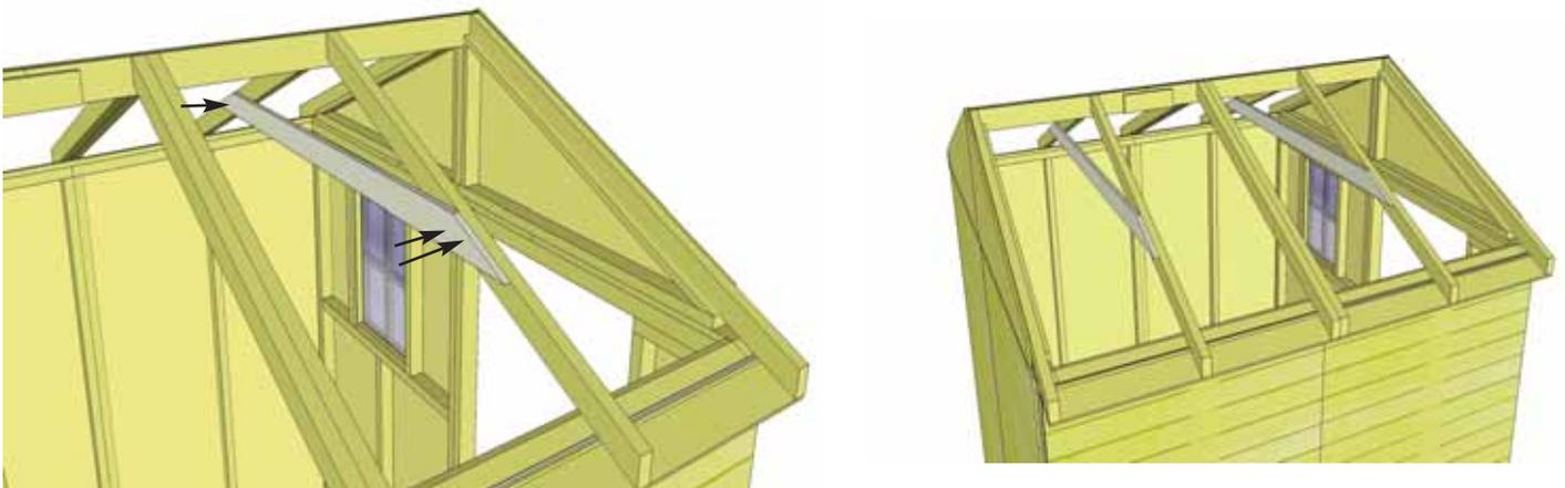
**46.** **Roof Gussets** are positioned on both mid rafters. Slide gusset up, use level to square gusset and attach to rafters with 4 - 2" screws. Pilot hole each Gusset end with 1/8" drill bit. Complete remaining Gusset.
