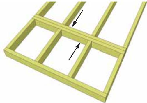
**4.** Attach each large and small floor joist frame together with 6 - 2 1/2" screws per section.
