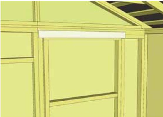
**73.** Attach Interior **Door Stops** to door framing from inside of shed. Start with Horizontal piece first. Use 4 - 2" screws to secure each Stop. Stops should overlap door by approx. 1/2".
