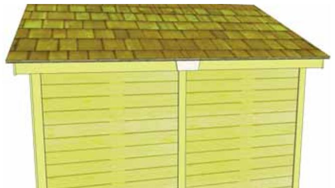
**66.** Attach **Horizontal Gable Trim Detail and Facia Trim Detail Plates** to cover seams where facia and horizontal trim pieces come together. Horizontal Gable Trim Detail Plates are 4 1/2" high while Facia Trim Detail Plates are 3 1/2" high. Secure each with 4 - 1 1/2" finishing nails per piece.
