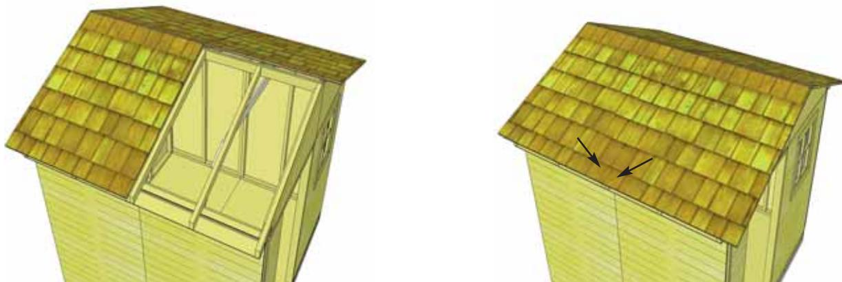
**50.** Position and attach Left Side Roof Panels as per **Steps 47-49.**
