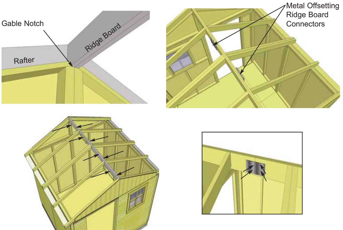
**43.** At the peak, align Ridge Boards so they are flush together and secure them with 8 - 1 1/4" screws. To completely secure Ridge Boards, place 4 - 1 1/4" screws into any of the remaining Metal Ridge Board Connector holes. Complete both sides. **Important:** if there is a gap between Ridge Boards, try pushing side walls closer together from outside. Walls should be 91" apart at top from inside of wall plate to wall plate.
