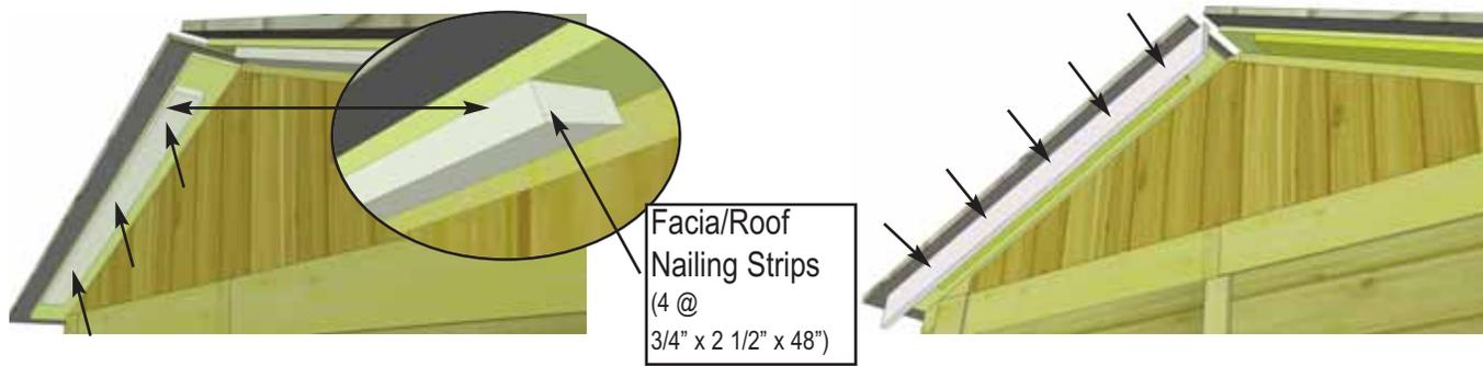
**60.** Attach **Facia/Roof Nailing Strips** (3/4" x 2 1/2" x 48") to the underside edge of the plywood roof with 3 - 1 1/4" Screws per piece. Nailing Strip will make it easier to attach Front and Rear Facia in **Step 61**. **Complete Front and Rear Strips (4 pieces total)**.
