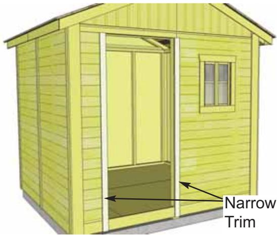
**64.** Position the 2 remaining **Narrow Trim** (2 - 1/2" x 2 1/2" x 77 1/2") pieces flush with inside of door jamb. To determine vertical height of trim, do a dry run with Horizontal Gable Trim in **Step 65**. Make sure Gable Trim covers flashing and mark. Attach Trim with 8 - 1 1/2" finishing nails.
