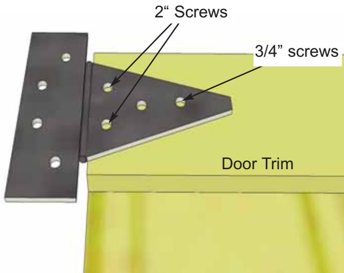
**69.** Attach **Door Hinges** to **Door Panel**. At this stage, door can swing open on the left or right. Decide on your preference and attach hinges to door. (3 hinges per door centered on door trim.) Use 3/4" and 2" long black screws on hinge / door attachment as illustrated above.
