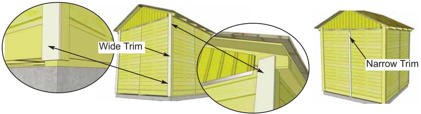
**59.** Position **Wide Trim** (1/2" x 4 1/2" x 82") over Filler Trim and to cap Narrow Trim. Align Wide Trim at bottom with Narrow Trim so flush with each other. Secure trim with 8 - 1 1/2" finishing nails. Complete remaining corner trims. Attach **Narrow Rear Wall Trim** (1 - 1/2" x 2 1/2" x 77 1/2"), where rear wall panels come together and leave a seam, with 8 - 1 1/2" finishing nails. Align Trim at bottom with the corner trims.
