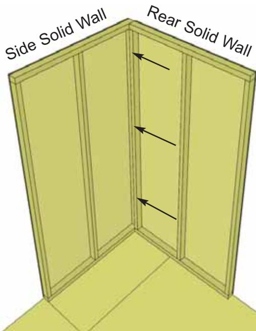
**Do Not Attach Walls To Floor Until Step 23.**
