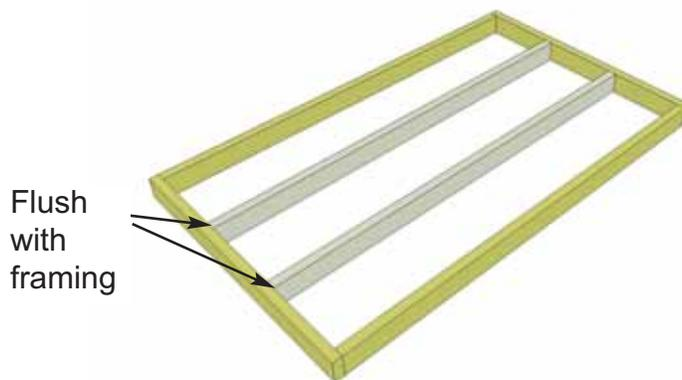
**1.** Lay out **Large Floor Joist Frame** and **2 Floor Joists** as illustrated above. Position Joists equally in Floor Joist Frame. Use **Small Floor Joist Frame** as a template to determine joist position. Position Joist so flush with framing.
