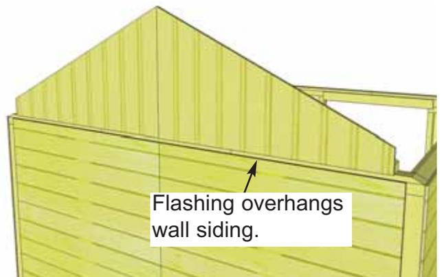
**33.** The gable should be centered sideways (left to right) on the top plate. **Hint:** use a straight edge to check the angle of the gable framing and top plate. Both angles should line up. Adjust gable accordingly. Temporarily attach Gable to walls and top plate with 2 - 2" screws. Screw from the bottom of gable framing down into Top Plate and Wall. Gables may need slight adjustment in **Step 44** and then will be completely attached with an additional 6 - 2" screws.
