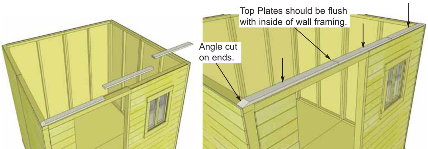
**28.** Position **Front Top Plates** on top of wall studs so they are flush on the inside with 2x3 wall framing. There are 3 pieces of Front Top Plates (2 angle cut on one end and one straight cut on both ends). Together, the plates should be centered evenly on the wall left to right. Attach by screwing down into top wall framing with 4 - 2" screws.
