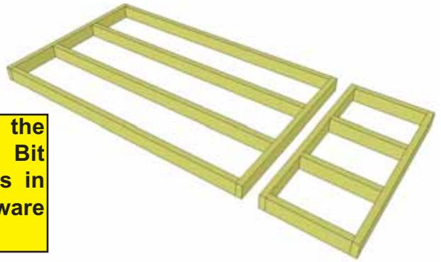
**2.** When correctly positioned, attach each Joist with 4 - 2 1/2" screws (2 per end).
