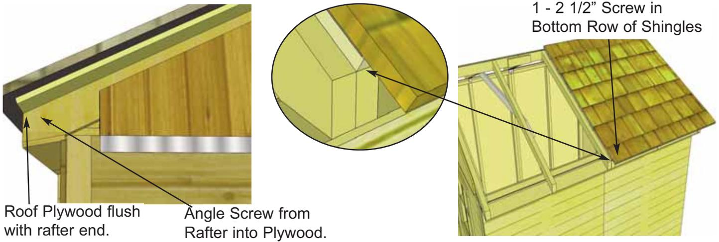
**48.** Place Roof Panel so it sits flush on 3rd rafter from the outside (doubled up rafter). Plywood on roof should be flush with end of rafter at bottom. From the outside, screw down through bottom row of shingles into rafter with 1 - 2 1/2" screw. Angle a 2 1/2" screw from outside rafter into roof plywood.
