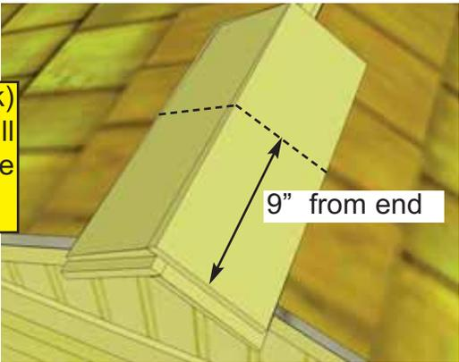
**67.** Place First Roof Ridge Cap on roof peak overhanging shingles by approximately 2". Attach with 2- 1 1/2" Shingle Nails 9" from end. Place 2nd Ridge Cap 1" back from 1st cap. Attach with 2- 1 1/2" Shingle Nails 9" from end.
