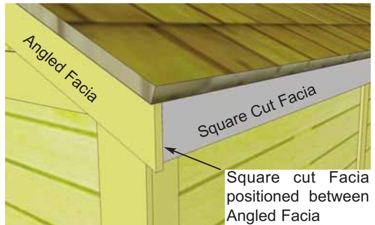
**61.** Position **Front and Rear Facia** (angle cut on ends) and **Side Facia** (square cut on ends) in corner. Line Fascia up so square cut Facia is positioned between angled cut facia. Attach angled facia to plywood end with 6 - 1 1/2" finishing nails per piece. Gap where facia boards come together at peak will be covered in **Step 63**. Do a dry run using Fascia to help you correctly position before attaching.
