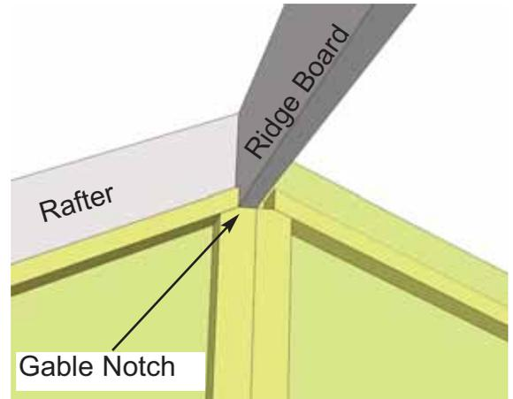
**40.** Slide Rafter Section up on gable framing until bottom of Ridge Board slips into gable notch.
