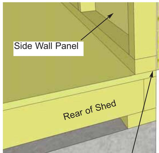
Outside 2x3 framing of wall panel is flush with outside of floor frame when properly aligned.
