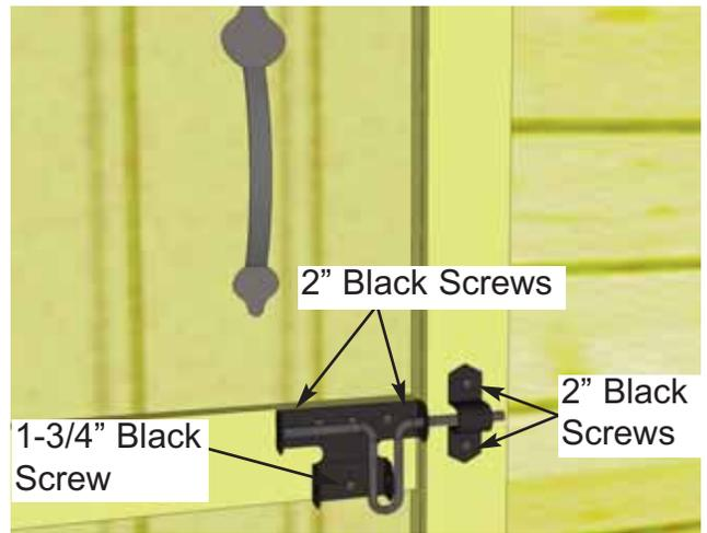
**72.** Attach **Black Barrel Bolt** as illustrated above with 2" & 3/4" Black Screws. Note how female part of Barrel Bolt is positioned higher than male. Do a dry run first to position Barrel Bolt correctly. **Important:** Drill pilot holes with 1/8" drill bit prior to securing with screws to prevent wood splitting. On 3/4" screw, drill shallow pilot hole only.
