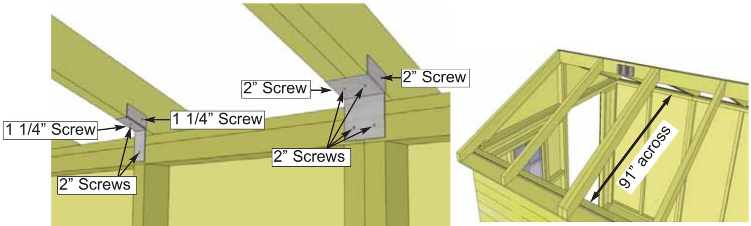
**45.** Attach all **Single and Double Rafter Brackets** where rafters meet Top Wall Plates inside of shed. Attach with 2 - 1 1/4" screws and 2 - 2" screws per Single Bracket and 6 - 2" screws per Double Bracket.
