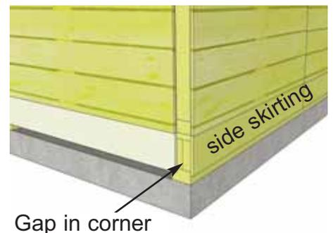
**56.** Attach **Bottom Skirting** around the base of the shed. Skirting will hide floor framing. The side skirting pieces will meet together in the center. Gaps on outside will be covered by Wide Trim pieces later. Start with front and rear skirting pieces first and attach with 4 - 1 1/2" finishing nails per piece.
