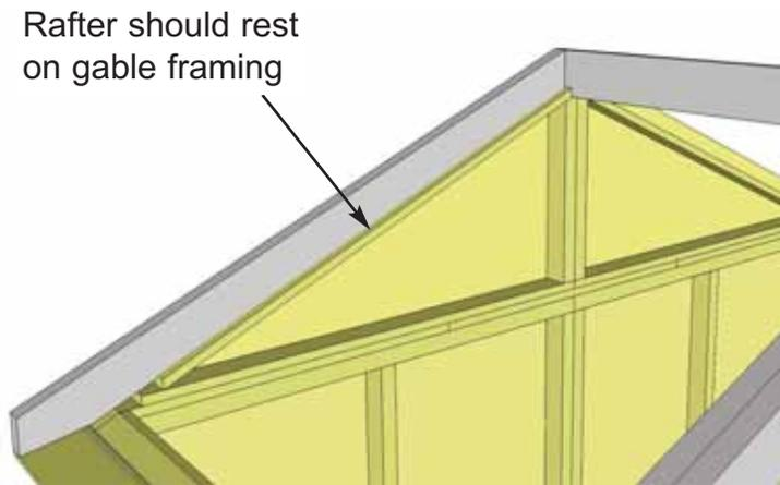
**41.** When Rafter Section is correctly positioned, outside rafters will sit equally on gable framing and Soffit will sit approximately 1/8" away from wall panels.
