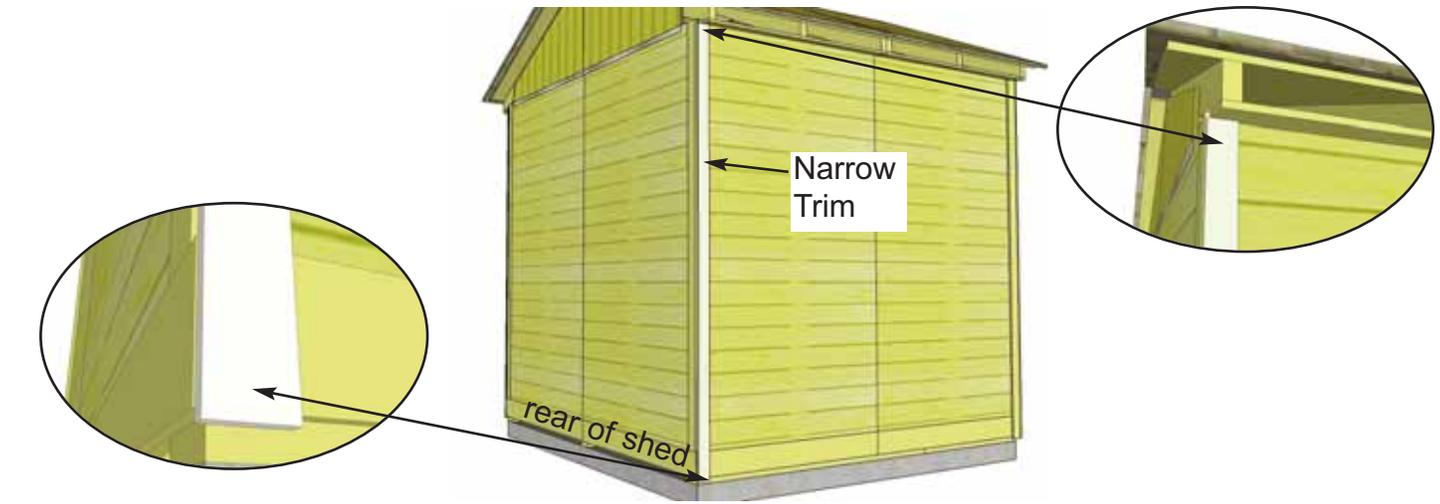
**58.** Align and attach both **Narrow and Wide Trims** in each corner. Starting with a Narrow Trim (1/2" x 2 1/2" x 79" long), align tight underneath Soffit and Rafter. Position flush with Filler Trim so Wide Trim will cap it when attached in **Step 59**. Use 8 - 1 1/2" finishing nails to secure. Note that Narrow Trim will sit slightly below Bottom Skirting when correctly aligned.
