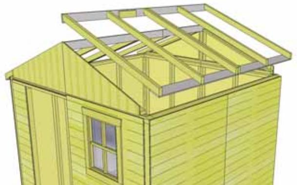
**42.** Place 2nd completed Rafter Section on gable wall framing. Position as per **Steps 39 & 40.**
