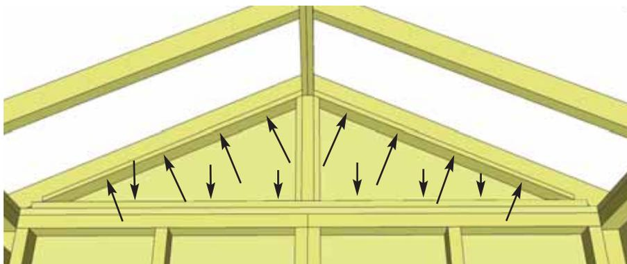
**44.** With both Ridge Boards connected, completely secure Gable framing to walls and rafters. Use 4 - 2" screws per Rafter. Use an additional 6 - 2" screws to secure Gable to wall. **Note: you may have to remove the 2 temporary screws in Gable from Step 33 and reposition Gable for best fit prior to completing gable attachment.**
