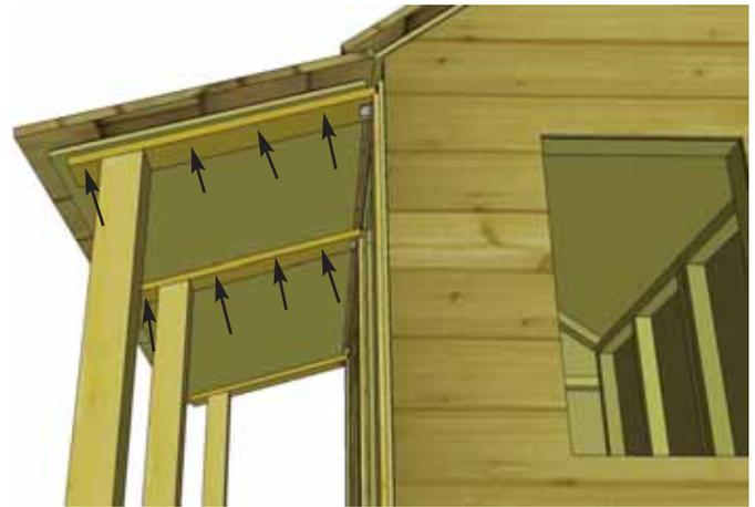
**41.** Using 2" screws, secure Porch Roof Panel to each Porch Rafter from underneath.
