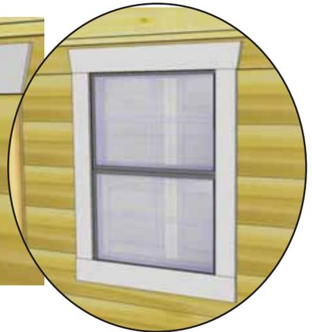
**61.** Position **Window Trim** around window doing a dry run first and attach with **4 - 1 1/2” Finishing Nails** per piece. Window trim has a small dado on reverse face. Outside flange of window will roughly sit in the dado to give a better fit.
