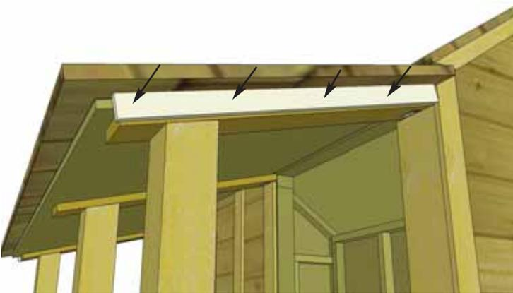
**47.** Position **Porch Facia Trims** on ends of Porch roof plywood. Align tight against shingles. Attach with 4 finishing nails per piece.
