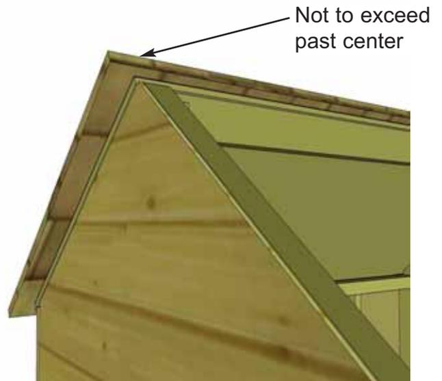
**36.** Starting at the rear, locate one of the **Roof Panels** (Roof Panels are all identical). Place on Gable Wall framing evenly from left to right. At top, Roof Panel should not exceed past the center of apex.
