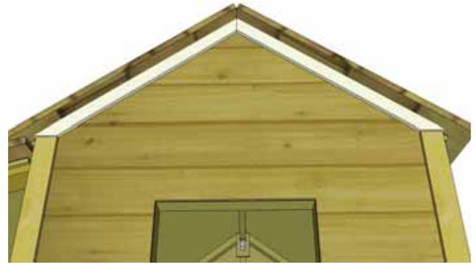
**46.** Position **Side Facia Trims** on ends of roof plywood. Align tight against underside of shingles so both Side Facia Trims meet evenly at the peak. Attach to end of plywood with 4 finishing nails per piece.
