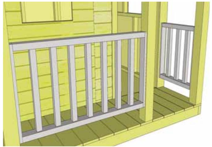
**35.** Position and attach **Front and Left Side Porch Railing** as in **Step 34**. Use a level to confirm both Railing and Porch Posts are square. If building a Little Squirt Playhouse with Elevated Platform for Sandbox, **DO NOT INSTALL Left Side Porch Railing**.
