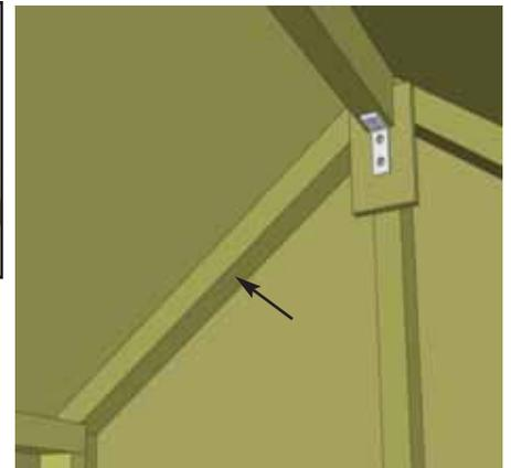
**38.** Position second Roof Panel evenly on front Gable Framing. Tack down with only 2 - 2 1/2" screws. Porch Roof may need to slide under Roof Panel and some play is required before completely securing.
