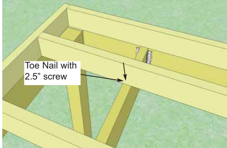
**18.** Align Floor Joist Frames so they sit flush with outside of Upper Girders of Elevated Platform. When positioned correctly, secure Floor Joist Frames with 18 - 2.5" screws, toe nailing on angle into Interior Joists. **IMPORTANT: Be careful that no screw tips are exposed after toe nailing. Run hand down Joists and visually inspect before proceeding. Remove and reposition screws if necessary.**
