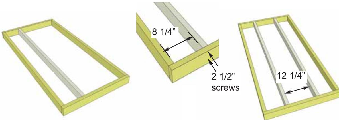
**16.** Next, attach **Floor Joist Frames**. Frames require two interior Floor Joist attachments. Measure Joist (8 1/4") from inside of Floor Joist Frame to inside of Floor Joist and attach with 2 - 2.5" screws per end. Complete attachments of both Floor Joists and both Floor Joist Frames.
