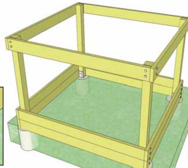
**13.** Locate **Upper Side Girder** (70" long and Pre-Drilled) and attach with Lag Bolts to Support Posts as per **Step 12**. Complete all Upper Girders as Per **Steps 12 & 13**.
