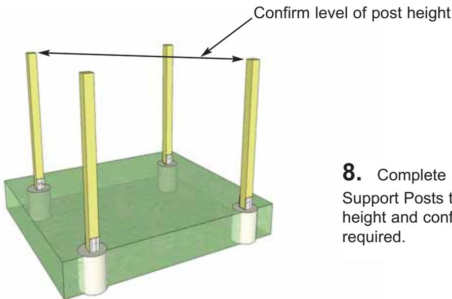
**8.** Complete positioning and attaching all Support Posts to Post Mounts. Measure post height and confirm that it is level. Adjust as required.
