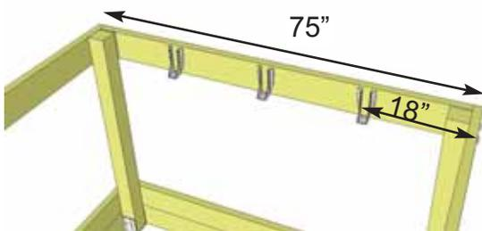
**14.** Locate **Interior Joist Holders (6)** found in hardware kit. Measure 18" on center on both Front and Rear Girder and attach Joist Holders with 1 1/4" screws. Place 67" long Interior Joists in Holders and attach with 1 1/4" screws.
