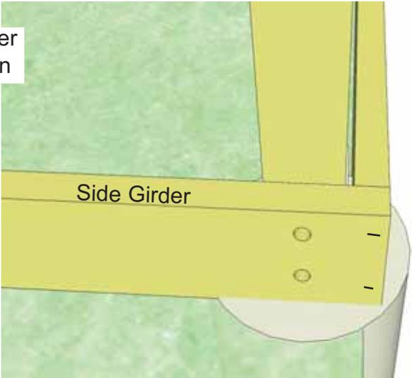
**9.** Carefully lift and re-position Lower Girder Section around Support Posts with your helper. Align Girders as per **Step 4**.
