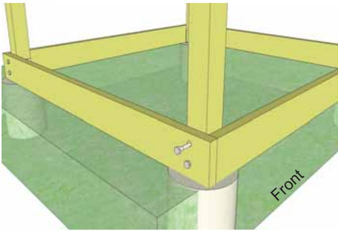
**10.** When correctly leveled and positioned, place **Lag Bolts with Washers** through Pre-Drilled holes of Lower Side Girders and tighten with 9/16th wrench. Complete both Side Girder attachments.
