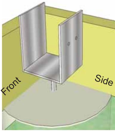
**4.** Place Post Mount in wet Concrete Form and position as illustrated.
