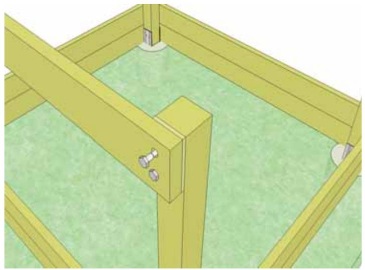
**12.** Locate **Upper Rear Girder** (Pre-Drilled and with a 3/8" Cleat on inside ends). Attach to Support Posts with 4 Lag Bolts. Make sure Girder is flush with top and sides of Posts with Cleat to the inside.
