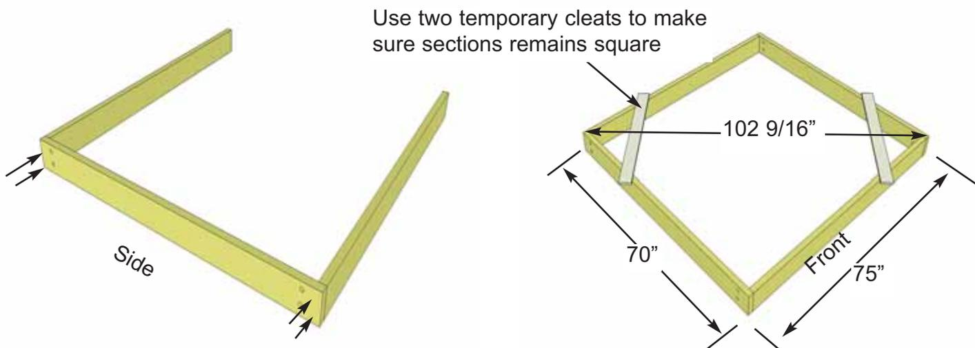
**2.** After the Playhouse is unpacked, to help determine correct placement of **Post Mounts**, use the assembled Lower Girder Section. Locate **(A) Lower Front** and **Rear Girders** and **(B) Lower Side Girders**. Screw Side Girder into both Front and Rear Girders with 2 - 2.5" screws per side. When completed your Lower Girder Section should be 75" wide x 70" deep.
