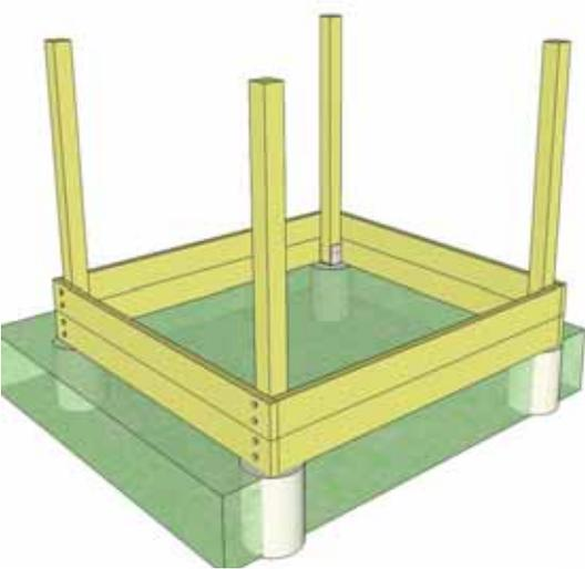
**11.** Place second Left Side Girder between Support Posts directly on top of Lower Girder and attach as per Lower Girder. Attach Front and Rear Girders with 2 - 2.5" screws per side. Complete Right Side Girder to complete as per left side.
