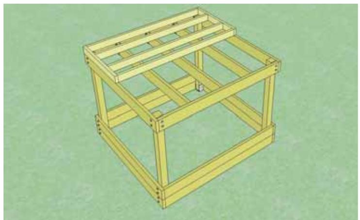
**17.** Carefully lift completed Floor Joist Frames and position on Elevated Platform so long floor joists run perpendicular with interior floor joists of platform.
