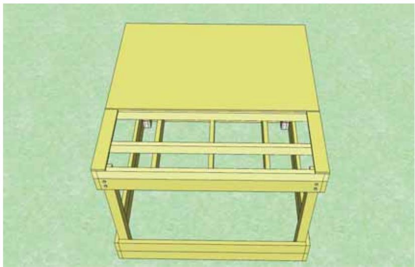
**21.** Position Outside Deck Board so that it is flush to front with 1/2" gap in the rear. When correctly positioned, attach both outside boards with 3 - 1 1/4" Screws.
