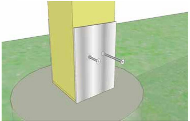
**7.** Locate 3 1/2" x 3 1/2" **Support Posts**. Position and attach bottom to Post Mount. Use Hardware recommended by Post Mount Manufacturer.
