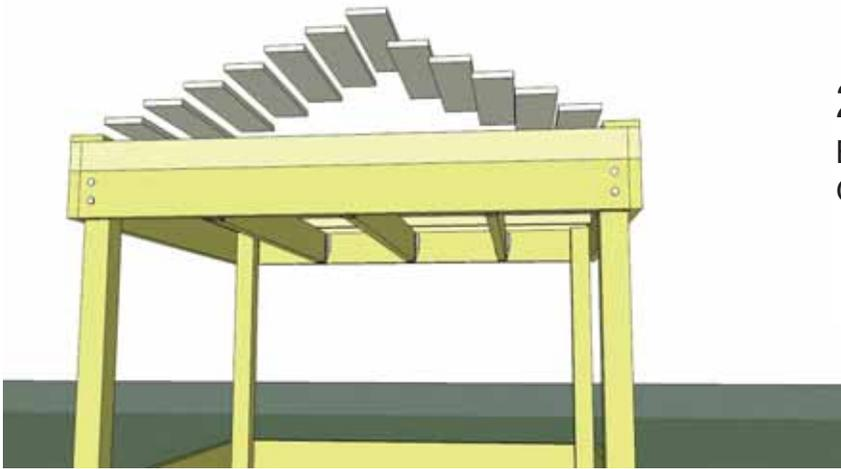
**22.** Position remaining Interior Deck Boards (12 @ 5 3/8" wide) between Outside Deck Boards.
