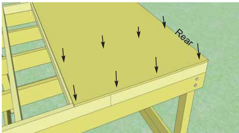
**19.** Locate **Plywood Floor** and position flush with outside of rear Floor Joist Frame. When in correct position, attach with 1 1/4" screws. Use screws every 16". **IMPORTANT: Be careful that no screw tips are exposed after the Floor is attached. Visually inspect before proceeding. Remove and reposition screws if necessary.**
