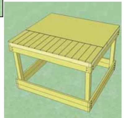
**23.** Space Deck Boards so there is approximately an 1/8" gap between boards and attach with 3 - 1 1/4" screws per piece.
