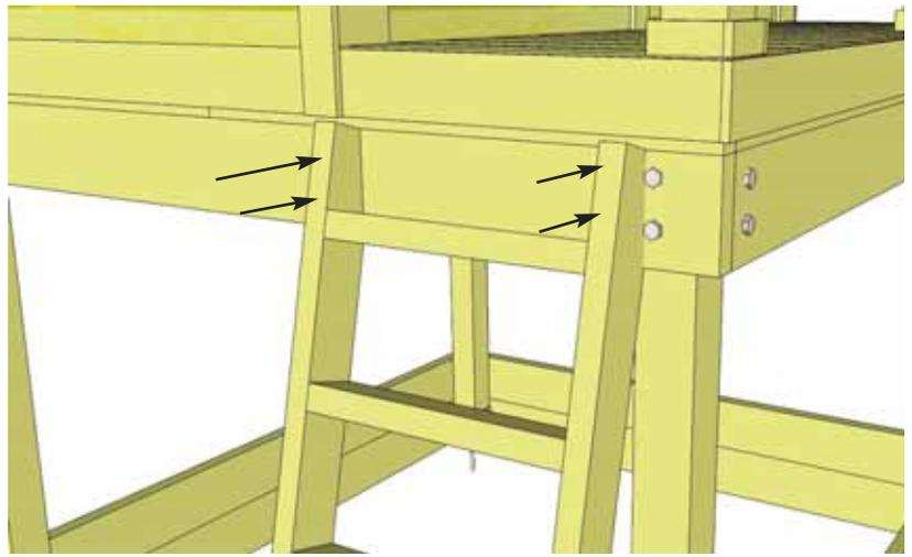
**24.** Attach **Ladder** to Upper Girder with 4 - 2.5" screws. Pilot Hole Ladder to prevent wood from splitting.
