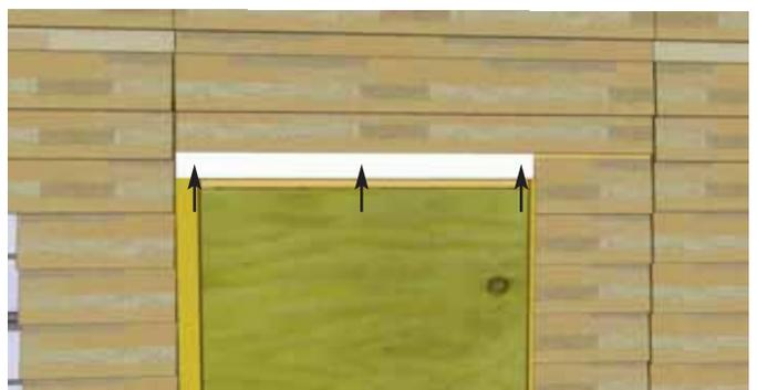
**33.** To complete the door stops, attach the Horizontal Door Stop against Door Header and attach with **3 - 1 1/4" screws**.
