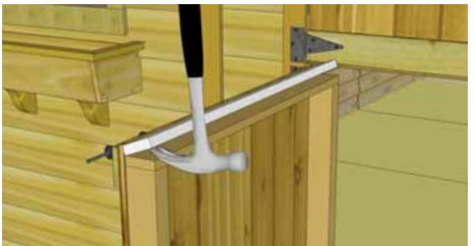
**27.** To accommodate Interior Door Plywood, the existing top plate on bottom door must be removed first. Using a hammer, carefully pry off the top plate and remove any hardware.
