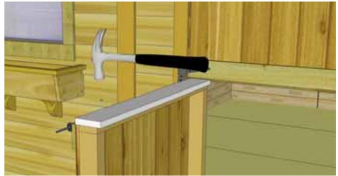
**28.** Position replacement top plate on bottom door and attach with **6 - 1 1/2" Finishing Nails**. Replacement Top Plate will cap door siding.
