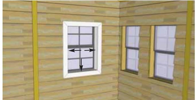
**42.** Locate the 4 large Window Inserts and position in window cavity. Nail to window wall framing with **9 - 1 1/2" Finishing Nails** from the bottom and sides. Complete the smaller window inserts in the same fashion.
