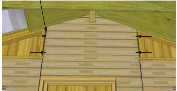
**23.** Lift up Front Center Gable Panels and slide notch up against roof Ridge Board. Once Gable Panel is aligned correctly, attach to gable framing with **4 - 1 1/4" screws**.
