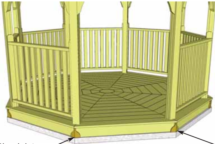
Rim Joist Corner Detail Plates
