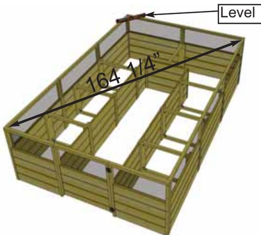
**1.** Prior to installing your Deer Fence Option Kit, confirm your 8x12 Raised Bed is level and square. Measure diagonally inside corner to corner (approximately 164 1/4") in both directions. Adjust as required. Use a level to determine if the tops of the bed frames are sloped and adjust if necessary.
