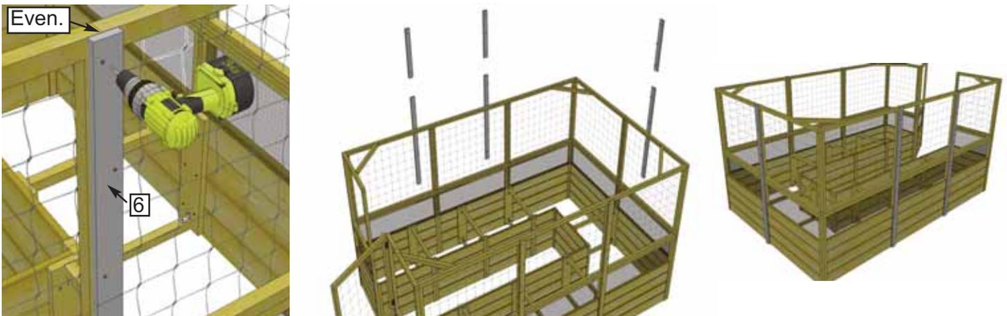
**9.** Position and attach short Vertical Panel Support using **3 - 2" screws** as per Step 7. Complete remaining rear and side walls.
