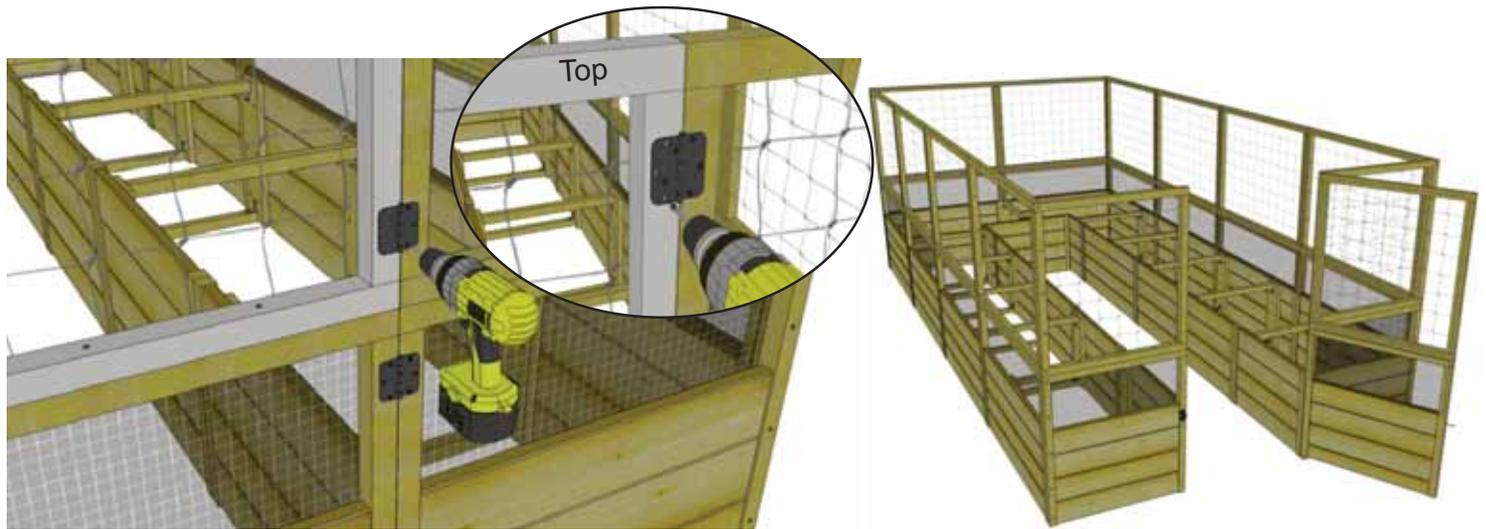
**6.** Locate both **Black Plastic Hinges (3)** and attach to deer fence frame with **6 - 3/4" black screws per hinge** as shown above. Use 1/8" drill bit to pilot hole shallow holes before attaching to avoid splitting deer fence framing. Open and close door to check door aligned correctly. Adjust as required.
