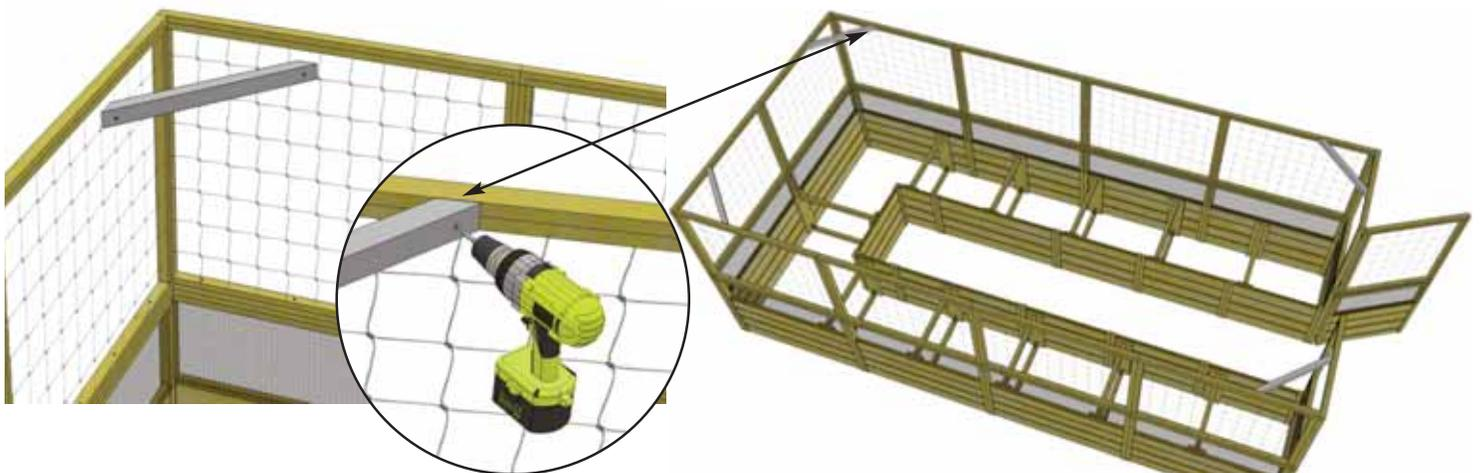
**7.** Attach **Corner Brackets with angle cut ends - (4)** on the inside frames at the top. Use **2 - 2 1/2" screws** per bracket. Screw on an angle. Pre-drill ends with 1/8" drill bit to prevent wood splitting.
