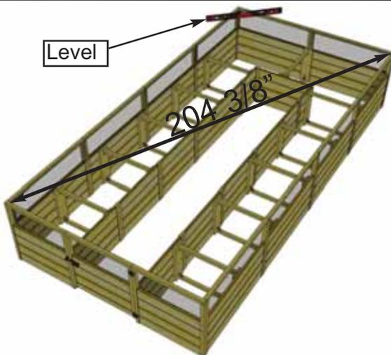
**1.** Prior to installing your Deer Fence Option Kit, confirm your 8x16 Raised Bed is level and square. Measure diagonally inside corner to corner (approximately 204 3/8") in both directions. Adjust as required. Use a level to determine if the tops of the bed frames are sloped and adjust if necessary.
