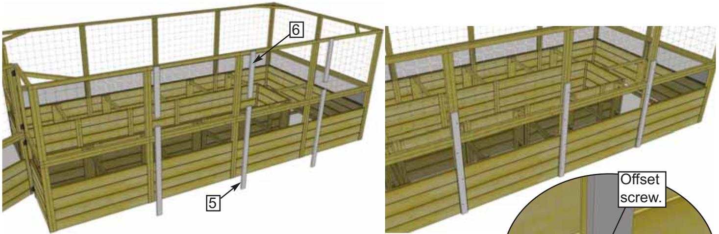
**8.** Locate **Vertical Panel Supports - Long (5) - 3/4" x 2 1/2" x 45"** and **Vertical Panel Supports - Short (6) - 3/4" x 2 1/2" x 22"**. Starting with 45" long support first, center on panel frames, flush at bottom and attach with **4 - 2" screws**. Offset the screw to either side of the support to ensure you contact the heart of the bed frame.
