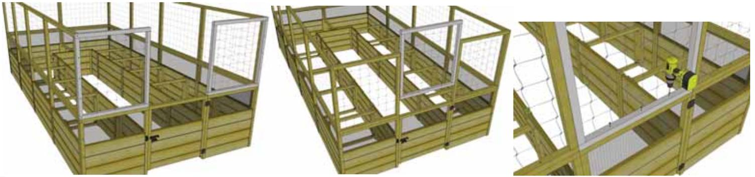
**5.** Locate all three **Front Deer Fence Panels (2) - 30 5/8" wide x 33 1/2" high**. Designate one to be a door panel and leave to the side. Attach both outside panels as per **Steps 1 - 3** except use only **3 - 2 1/2" screws** to attach bottom frame. Position and install designated door panel between front panels and screw only from bottom frame into top of raised bed door frame with **3 - 2 1/2" screws** as shown above.
