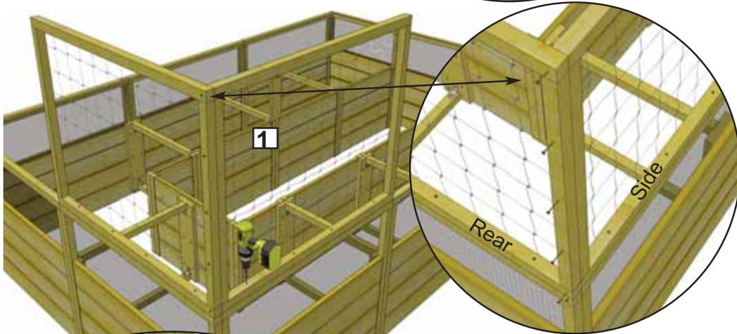
**3.** Position a **Side Panel (1) - 46" wide x 33 5/8" high** directly on top of the side raised bed frame. Hold both deer fence frames together and starting at the top, screw together with **5 - 2 1/2" screws** as shown on the left. Screw bottom of frame down to raised bed frame with **4 - 2 1/2" screws**.
