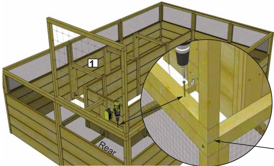
**2.** Starting in rear corner, position the frame of a **Rear Panel (1) - 46" wide x 33 5/8" high** directly on top of the raised bed frame. Screw frames together with **4 - 2 1/2" screws** as shown on the left.
