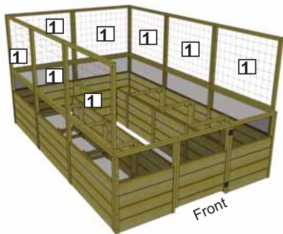
**4.** Position a second **Rear Panel (1) - 46" wide x 33 5/8" high** on top of the rear raised bed frame. Hold both rear deer fence frames together and starting at the top, screw together with **4 - 2 1/2" screws** as shown above. Screw bottom of frame down to raised bed frame with **4 - 2 1/2" screws**. Complete remaining side and rear panels attachments following **Steps 2 and 3**.
