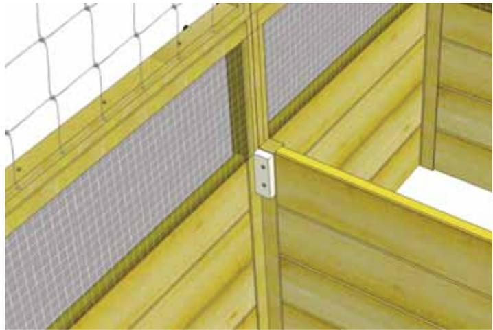
**11.** The **Door Stop (I)** and screws were included with your 8x12 Raised Garden Bed Kit. See **Step 21** of that manual. Install the Door Stop at the top of interior panel frame as shown above.
