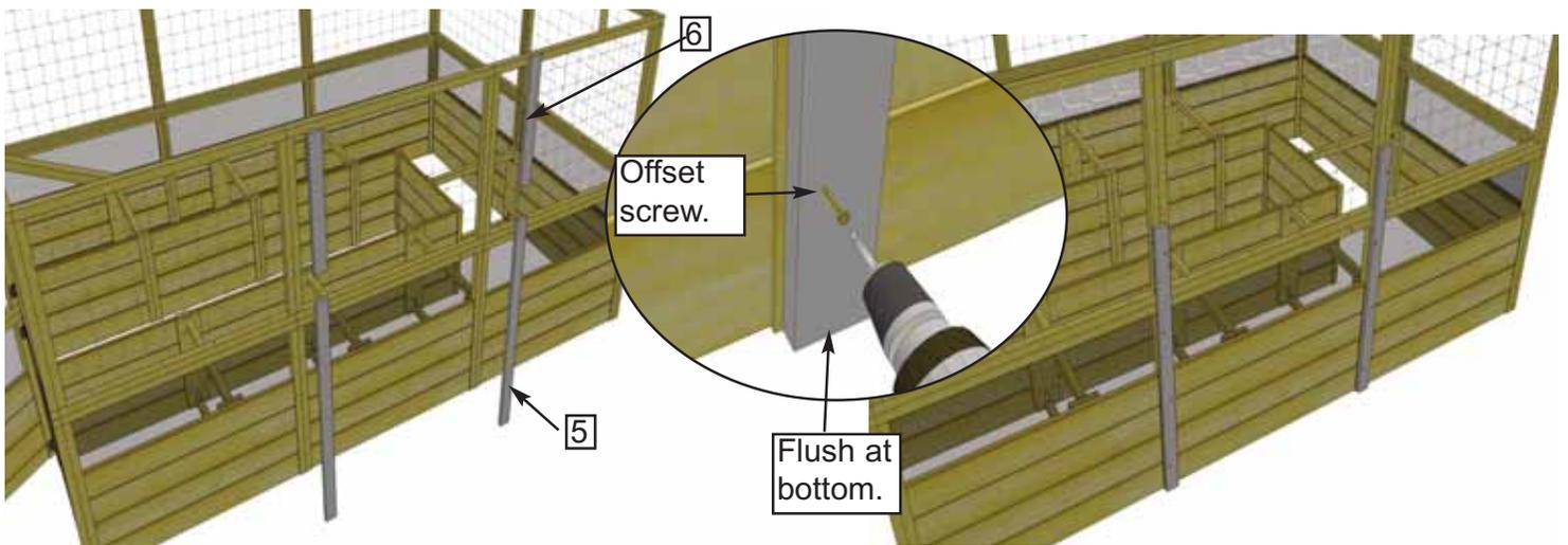
**8.** Locate **Vertical Panel Supports - Long (5) - 3/4" x 2 1/2" x 45"** and **Vertical Panel Supports - Short (6) - 3/4" x 2 1/2" x 22"**. Starting with 45" long support first, center on panel frames, flush at bottom and attach with **4 - 2" screws**. Offset the screw to either side of the support to ensure you contact the heart of the bed frame.
