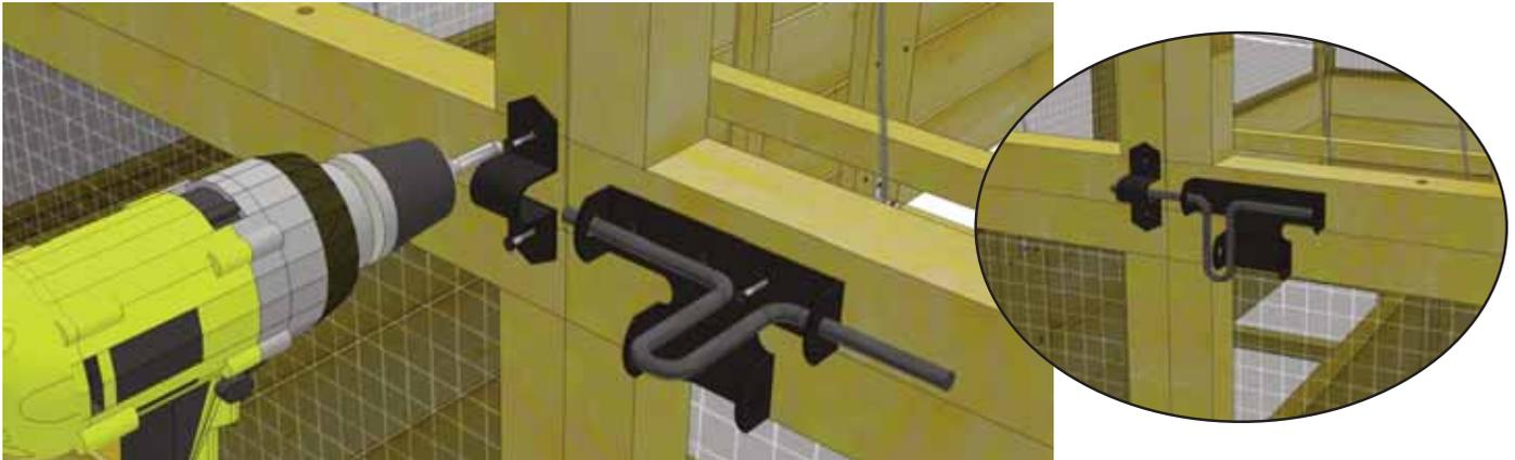
**10.** Attach Black Barrel Bolt to door and panel frame using **6 - 3/4" black screws**. Note how female part of Barrel Bolt is positioned higher than male. Do a dry run first to position Barrel Bolt correctly, then attach. Pre-drill with 1/8" drill bit to prevent wood from splitting.
