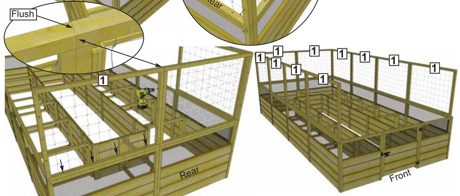
**4.** Position a second **Rear Panel (1) - 46" wide x 33 5/8" high** on top of the rear raised bed frame. Hold both rear deer fence frames together and starting at the top, screw together with **4 - 2 1/2" screws** as shown above. Screw bottom of frame down to raised bed frame with **4 - 2 1/2" screws**. Complete remaining side and rear panels attachments following **Steps 2 and 3**.
