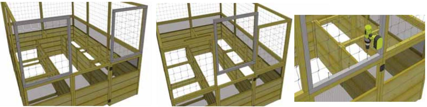
**5.** Locate all three **Front Deer Fence Panels (2)** - 30 5/8" wide x 33 1/2" high. Designate one to be a door panel and leave to the side. Attach both outside panels as per **Steps 1 - 3** except use only **3 - 2 1/2" screws** to attach bottom frame. Position and install designated door panel between front panels and screw only from bottom frame into top of raised bed door frame with **3 - 2 1/2" screws** as shown above.
