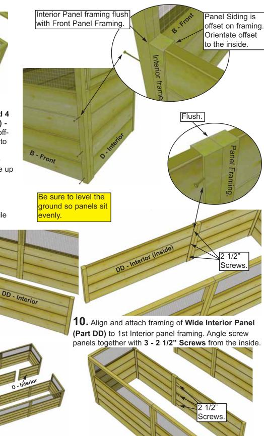
**11.** Align and attach framing of **(Part D)** and **(Part DD)** Panels as per **Steps 9 & 10**. Angle screw panels together with **3 - 2 1/2" Screws** from the inside.
