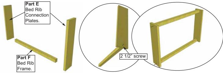
14. To complete rib assembly, locate all 18 Bed Rib Connection Plates (Part E) - 1" x 5 1/2" x 20".
