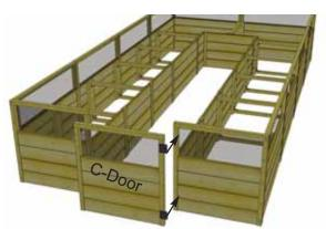
**20.** Locate **Door Panel (Part C) - 30 5/8" w x 33 1/2" h)** and position on flat surface screen down. Attach both hinges to door panel with **3 - 3/4" Black Headed Screws** per hinge. Space hinges evenly on door frame. Pre-drill shallow hole first to prevent wood from splitting.
