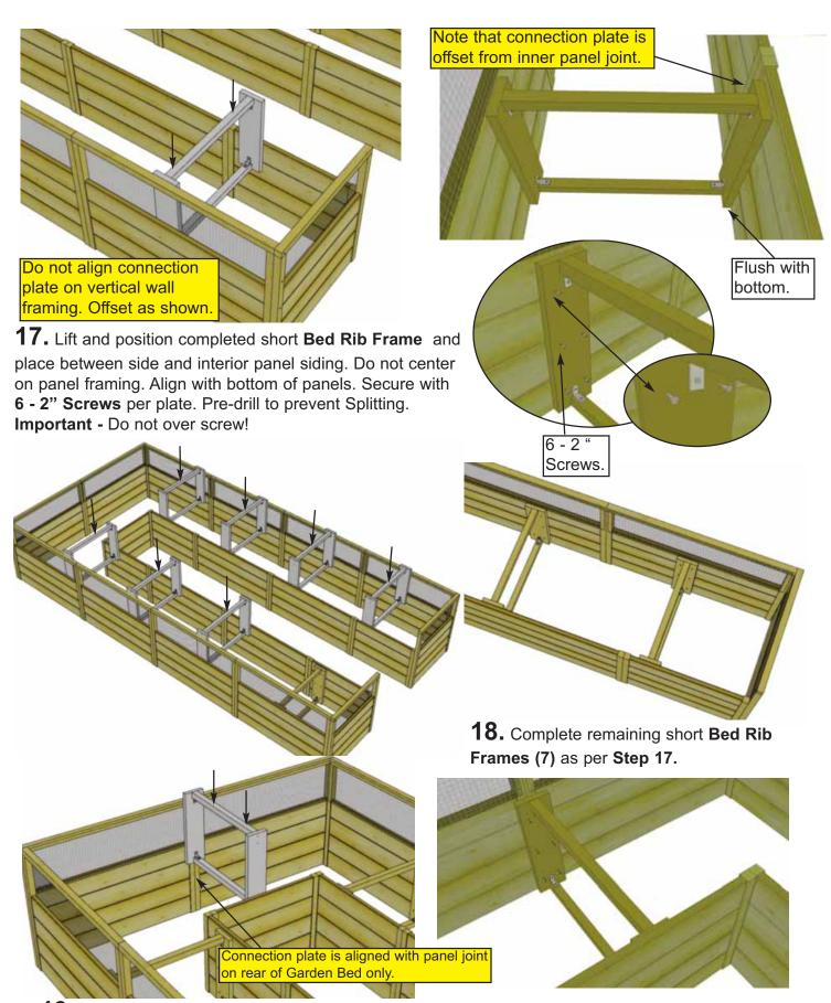
**19.** Lift and center completed longer **Bed Rib Frame** on rear and end interior panels. Align with bottom of panels. Secure with **6 - 2" Screws** per plate. **Important -** Do not over screw!
