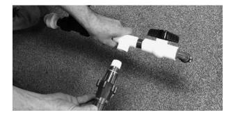
3. Attach Regulator with Hose Connector back on to main unit.
