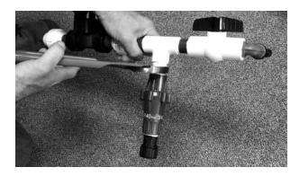
4. Tighten snug with wrench. Hook up main water supply to Regulator.
