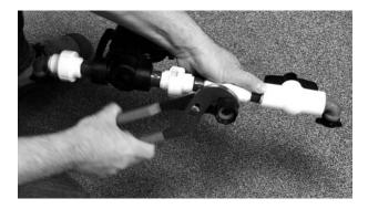
1. Remove Hose Connector on Main Irrigation Unit with wrench.
