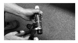
2. Attach Hose Connector snug to Pressure Regulator bottom.
