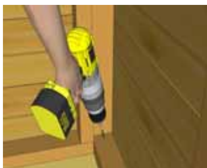
Angle screws into perimeter Floor Joists.
