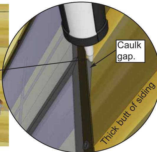
**83.** Once Insert is attached, caulk the "triangular gap" between the Insert's outside flange and the siding. Also put a bead of caulking horizontally at top of window where the flange and siding meet. This additional caulking will also will reduce the chances of moisture entering into your shed.
