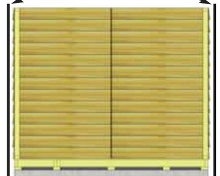
**23.** Prior to fastening walls and installing rafters, take time to confirm your walls are level, square and plumb. Measure diagonal at top and bottom of walls corner-to-corner. This should be approximately 125 1/4", but more importantly if measurements are not within 1/4", your walls are not square. Adjusting now will make it easier to install roof section.
