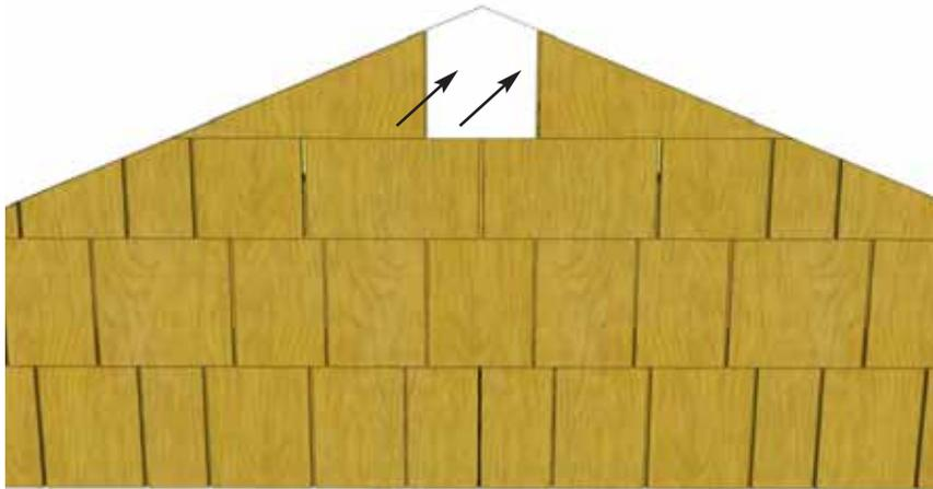
**31.** From the outside, slide in a Rear Gable Wall Filler Shingle to cover gable seam. Nail down above the exposure line with **2 - 1 1/2" Shingle Nails**. Complete by attaching the short 7 1/2" top Filler Shingle with **2 - 1 1/2" Shingle Nails**.
