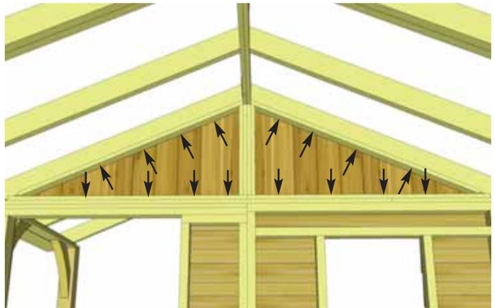
**46.** With both **Ridge Boards** connected, completely secure **Rafters** to **Gable** framing of **both rear and middle Gable Walls**. Use **8 - 2" screws** per gable.
