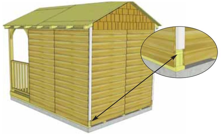
**63.** Attach **Rear Filler Trims** to rear walls, positioned flush with siding and bottom skirting. Attach with **8 - 1 1/2" Finishing Nails**.
