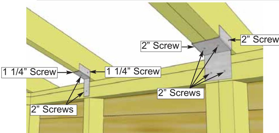
**50.** Attach all **Single** and **Double Rafter Brackets** where rafters meet **Top Wall Plates** inside of shed. Attach with **2 - 1 1/4" screws** and **2 - 2" screws** per **Single Bracket** and **6 - 2" screws** per **Double Bracket**.
