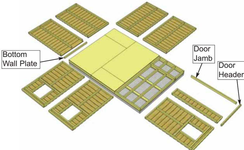
**12.** Lay out all the wall panels and become familiar with their location. On Standard Kits, there are **3 Window Wall Panels**, **4 Solid Wall Panels**, and **1 Narrow Porch Wall Panel**. Make sure to position panels right side up so water is directed away from and not into shed. Look at window wall panels to determine proper wall orientation.
