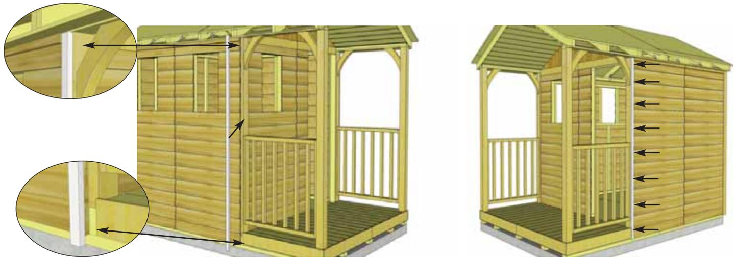
**65.** Position **Narrow Filler Trims** in gap between shed and porch. Attach with **8 - 1 1/2" Finishing Nails** per piece.
