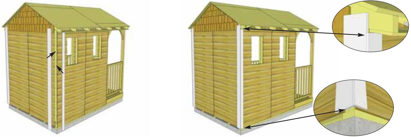
**64.** Position **Corner Trim** in rear corner and **Wide Corner Trim** over **Filler Trim**. Prior to attaching, do a dry run with Narrow Trim butted up tight underneath the Soffit. Position Wide Trim evenly with Narrow Trim at bottom. Narrow Trim will cap Wide Trim. Attach with **8 - 1 1/2" Finishing Nails** per piece. Repeat for other opposite rear corner.
