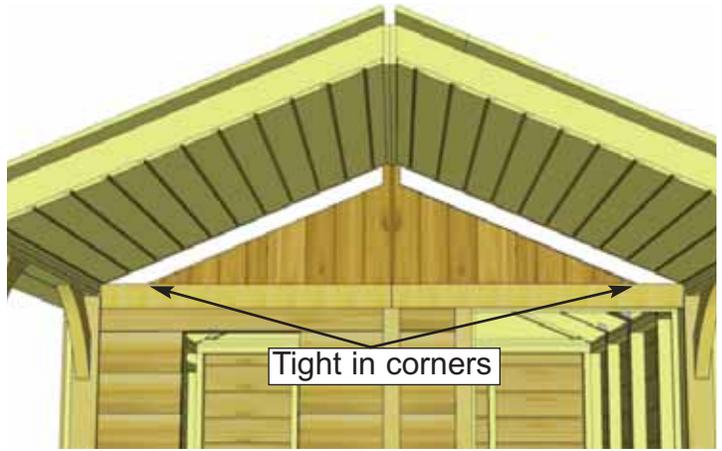
**69.** Position **Porch Roof Seam Trim** so the sharp angle of each piece is tight into the corner between Porch Ceiling and Horizontal Above Door Trim. Attach with **4 - 1 1/2" Finishing Nails** per piece.
