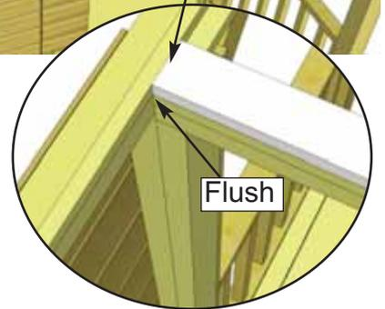
**27.** Position the **Front Top Plates** on top of Door Header and front wall panel. There are 2 plates (72" and 19" long). Front top plates are straight cut on the ends. Once again, the plate will be flush with inside of top wall framing. Attach with **6 - 2" screws** (4 screws in long and 2 in short plate).
