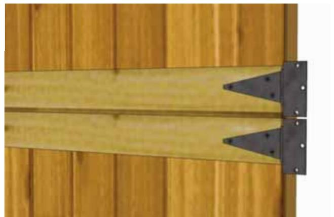
**85.** Attach Door hinges to Top and Bottom **Dutch Door** sections. Top Door has trim overhanging door at bottom while bottom door has trim recessed slightly. Hinges should be centered on door trim with barrel nudged to end of trim. Use **2" & 3/4" screws** as above.
