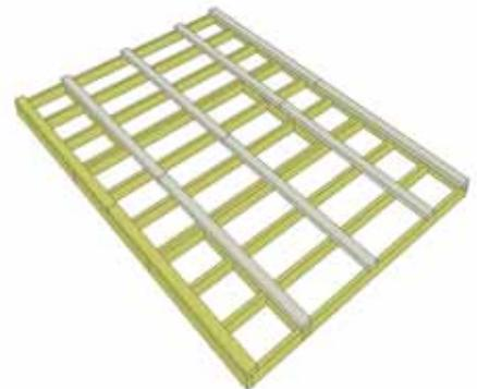
**7.** Attach **Floor Runners** to completed floor frame. There are 2 floor runners per 136 1/2" side and 5 completed runners in total. Use **6 - 2 1/2" screws** per completed Runner. Make sure Runners are flush with edge of floor framing, but not overhanging.
