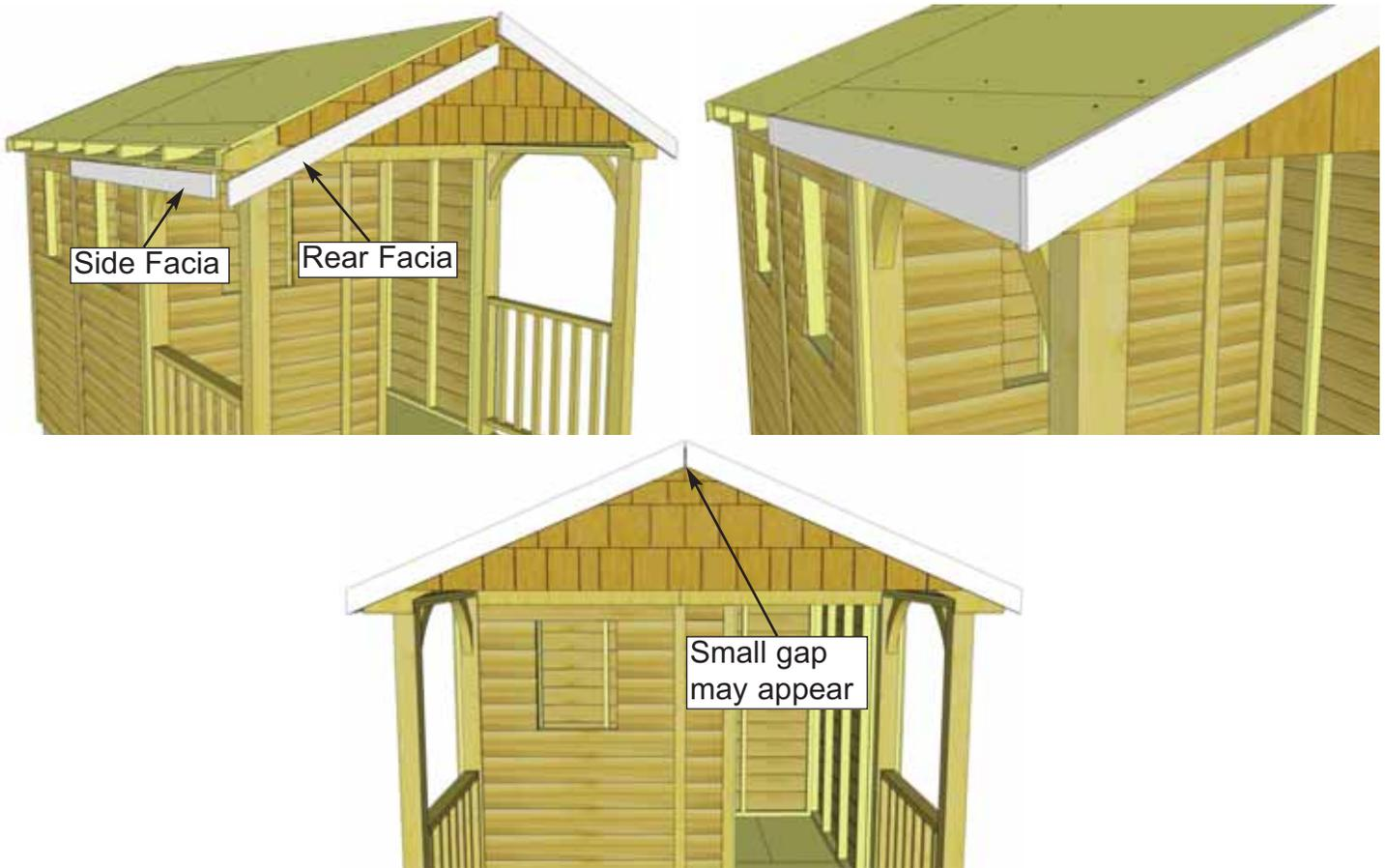
**76.** Position **Front Facia** - angle cut ends tight underneath roof shingles and tight against Nailing Strips. Temporarily position **Side Facia** for a dry run to help you correctly position Front Facia before attaching.
