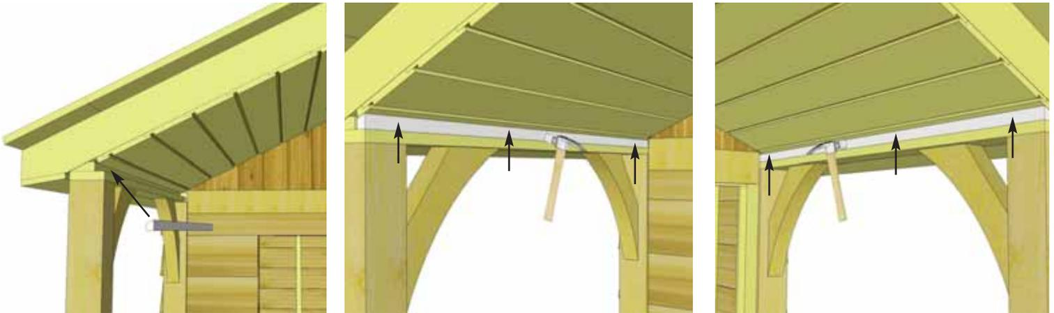
**58.** Insert **Porch Ceiling Support Strips** - Angle Edge Cut into the gap between the top of the Porch Rail Section and the Porch Ceiling Panel. Gently tap into place with a hammer. Once in place, attach each piece with **3 - 1 1/2" Finishing Nails** up through the Porch Rail Section into the Support Strips.
