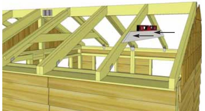
**49.** **Roof Gussets** are positioned on middle **Rafters**. Prior to attaching, make sure walls are properly aligned. Have two helpers push walls at the top from the outside of shed until inside to inside measurement between front and rear plates is 91". Use a level to square **Gusset**. Attach Gusset with 4 - 2" screws. First **Gusset** will sit below Rafter Nailing Cleat, second flush with Rafter.
