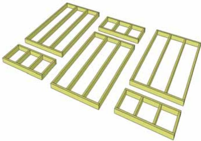
**3.** Lay out **Floor Joist Frames** as illustrated. There are 3 larger and 3 smaller Frame Sections. The Footprint for the floor when attached together will be 136 1/2" Deep x 96" Wide.
