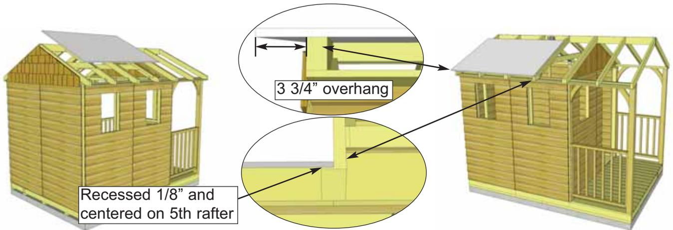
**51.** Identify all Roof Panels. Locate one **Large Plywood Roof Panel**. Position on rear side of shed. Recess plywood back 1/8" from end of rafter. Plywood will overhang rear of shed by 3 3/4". On opposite side plywood will be centered on 5th rafter, supported by Rafter Nailing Cleat.
