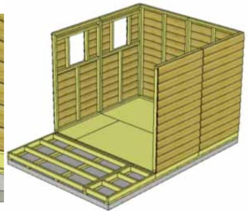
**16.** Be sure to correctly position wall panels so siding overhangs your floor and wall framing is flush with floor framing. Continue to attach walls together as per **Step 15**.
