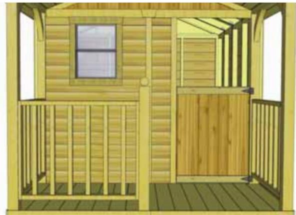
**86.** Place **Bottom Dutch Door** panel into position. Gap 3/8" on bottom, evenly space on sides, and attach hinge to doorway seam trim with **3 - 2" Black Headed Screws**. Use shim to help keep the door evenly spaced on bottom. One of the **Shim Shingles** can be used.
