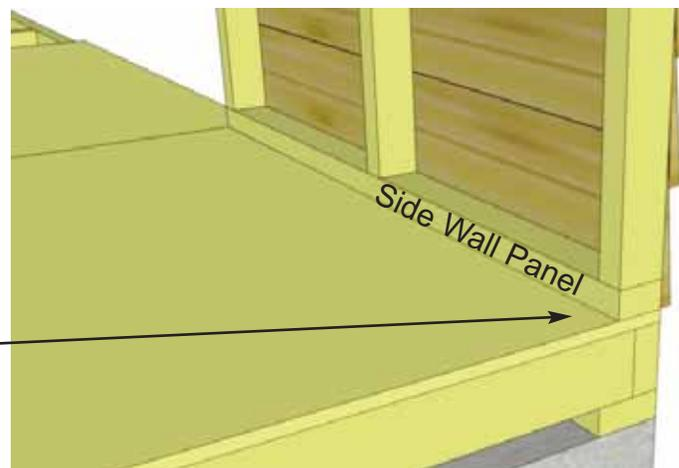
Outside 2x3 Plate of wall panel is flush with outside of floor frame when properly aligned. Floor plywood may be slightly recessed.
