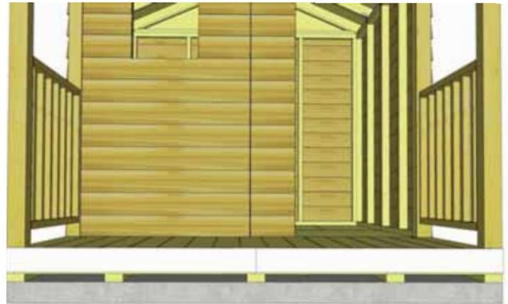
**59.** Attach **Front Bottom Skirting** around the base of the shed. Skirting will hide floor framing. Start with Front Skirting positioned flush with the top of the deck boards and the side of the floor frame. Attach with **6 - 1 1/2" Finishing Nails** per piece.
