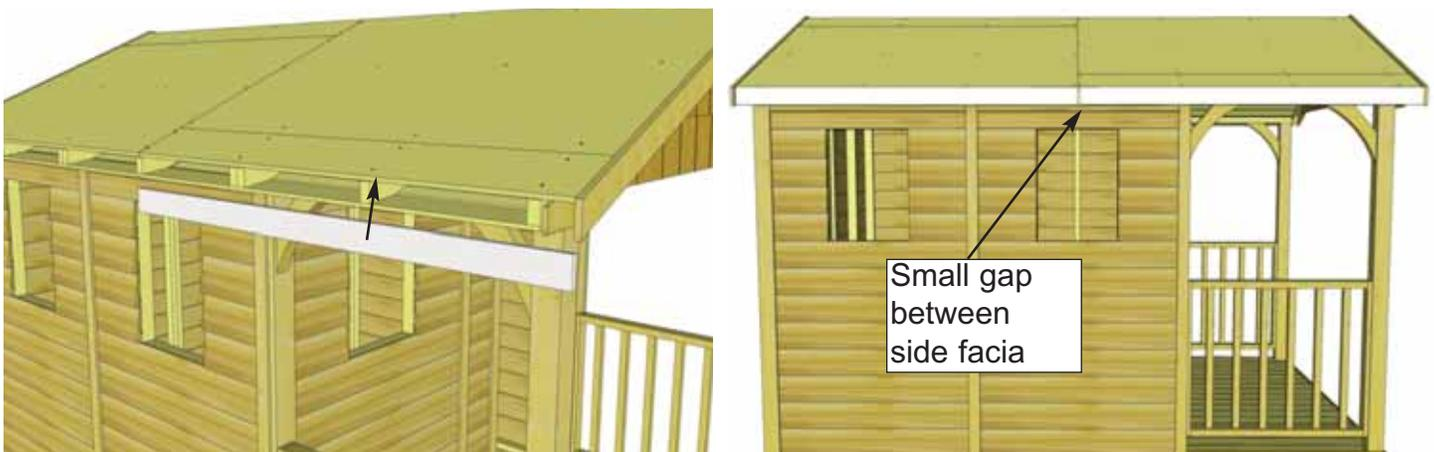
**77** Attach **Side Facia** to rafter ends. There are 2 Facia pieces per side. A small gap may appear between Facias, which will be covered in **Step 79**. Secure with **8 - 1 1/2" Finishing Nails** per piece.
