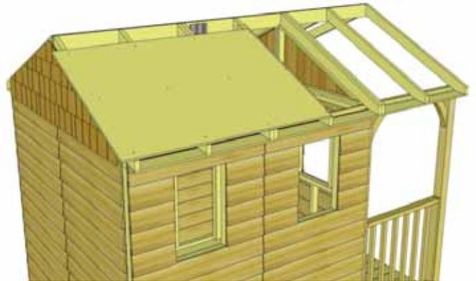
**52.** With Roof Plywood correctly positioned on rafters, attach with **12 - 1 1/4" screws**. On 5th rafter, be sure to angle screw to hit the meat of the rafter.
