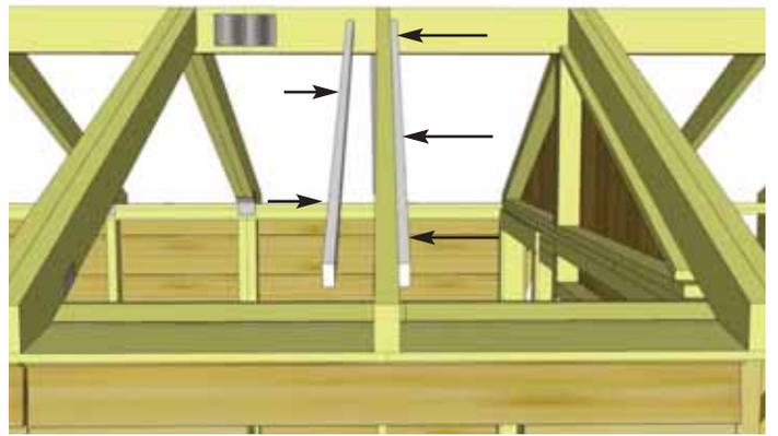
**48.** Position **Rafter Nailing Cleats** on center Rafter. Top of Rafter Nailing Cleat should be flush with top of Rafter to support plywood roof. Position **Rafter Nailing Cleat** to be 4 1/2" from each end of rafter as shown above. Pre-drill pilot holes in **Rafter Nailing Cleat** and then attach to rafter with **3 - 1 1/4" screws**. Repeat for each side of the rafter and then on opposite side of the roof.
