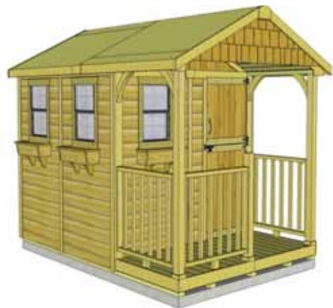
**92.** Assemble **Flower Box Kits** with Assembly Instructions included on Page 51. Position completed Flower Box below bottom of window trim and secure with **2 - 2 1/2" screws**. Screw from inside of box into the center wall stud. Attach second screw 2" underneath first screw and once again into the wall stud. Install Flower Box Kits underneath each window/double-window..
