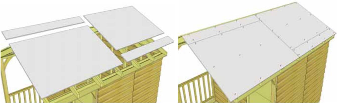
**55.** Repeat **Steps 51 - 54** to complete opposite side of roof with 4 remaining roof panels (2 large and 2 small).
