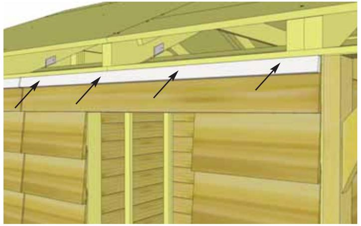
**62.** Trim out side walls by attaching **Top Wall Trim**. Position with thick end of Bevel downwards at top of wall, tight against Soffits. Attach with **4 - 1 1/2" Finishing Nails** per piece. Complete both sides
