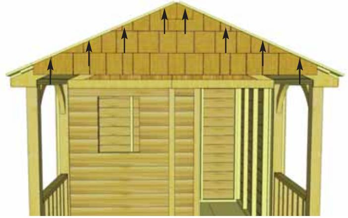
**74.** Position the **Gusset Gable** onto the front of the shed. Push Gable plywood up tight under roof plywood and against Roof Nailing Strip. Screw through the shingles of the Gusset Gable horizontally into the Roof Nailing Strip with **8 - 2 1/2" screws**.
