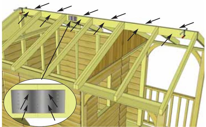
**45.** At the peak, align **Ridge Boards** so they are flush together and secure them with **12 - 1 1/4" screws**. To completely secure **Ridge Boards**, place **4 - 1 1/4" screws** into any of the remaining **Metal Ridge Board Connector** holes. Complete both sides. **Important:** If there is a gap between **Ridge Boards**, try pushing side walls closer together from outside. Walls should be 91" apart at top from inside of wall plate to wall plate.
