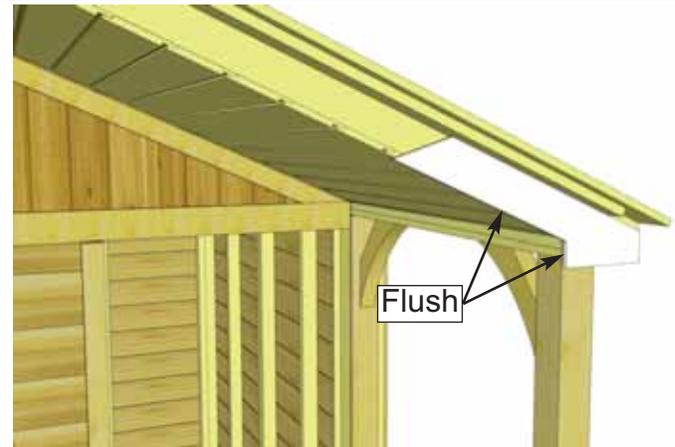
**73.** Position **Front Post Detail Covers** onto bottom corner of rafters, tight underneath Facia Nailing Strips. Covers should be approximately flush with the bottom of the Porch Roof, the inside of the 4x4 Porch Post, and the Rafter ends. Attach with **4 - 1 1/2" Finishing Nails** per piece.
