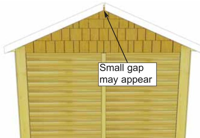
**75.** Position **Rear Facia** - angle cut ends tight underneath roof shingles and tight against Nailing Strips. Temporarily position **Side Facia** for a dry run to help you correctly position Rear Facia before attaching.
