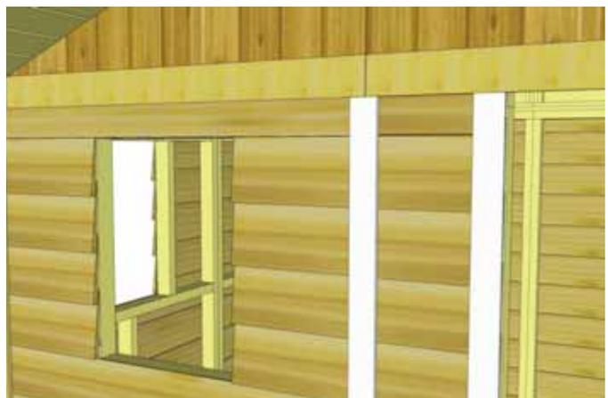
**68.** Attach both **Porch & Door Trims** to front walls. Secure with **6 - 1 1/2" Finishing Nails**.
