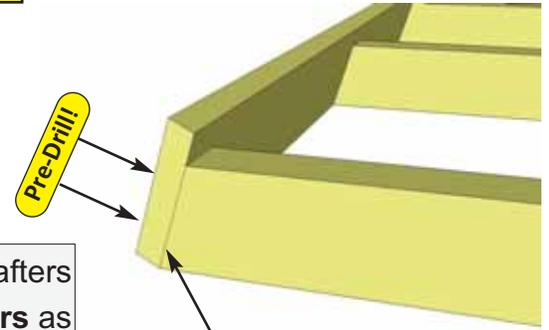
**37.** Attach completed **Ridge Board** to ends of both outside **Rafters** with **2 - 2" screws** per end. Measure and position interior **Rafters** as illustrated below. When positioned correctly, attach **Ridge Board** to remaining rafters with **2 - 2" screws** per **Rafter** end.
