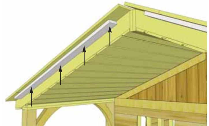
**72.** Attach remaining two **Roof Nailing Strips** to the underside of the roof plywood on front of shed. These strips will be pushed tight against the rafters unlike the Rear Nailing Strips. Fasten with **4 - 1 1/4" Screws** per piece.
