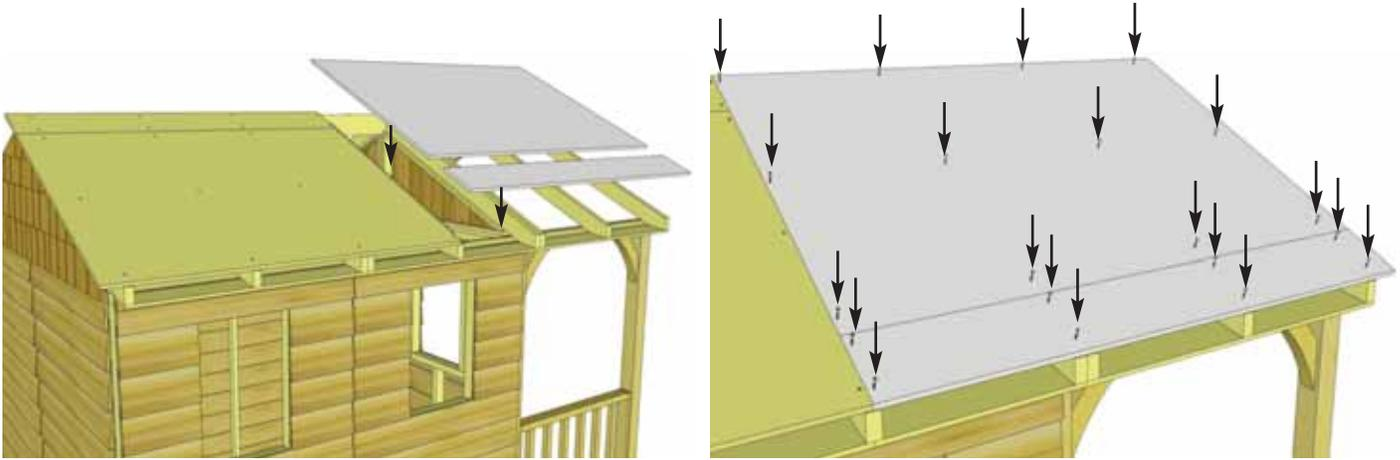
**54.** Locate one **Small Plywood Roof Panel** and one Large Roof Plywood Panel. Repeat **Steps 51 - 53** to complete 2nd half of roof but alternate which size of panel is near ridge board as shown above.
