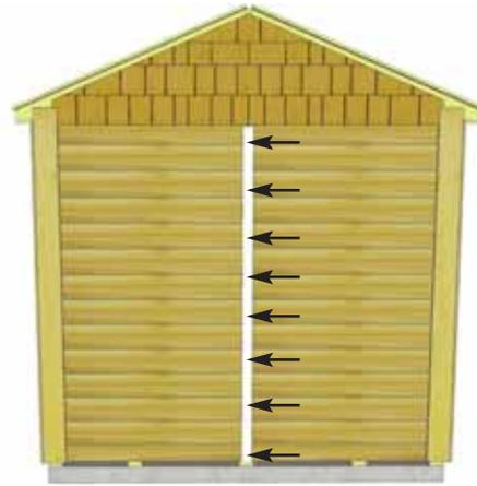
**67.** Attach **Rear Wall Seam Trim** where back wall panels meet. Secure with **8 - 1 1/2" Finishing Nails**.
