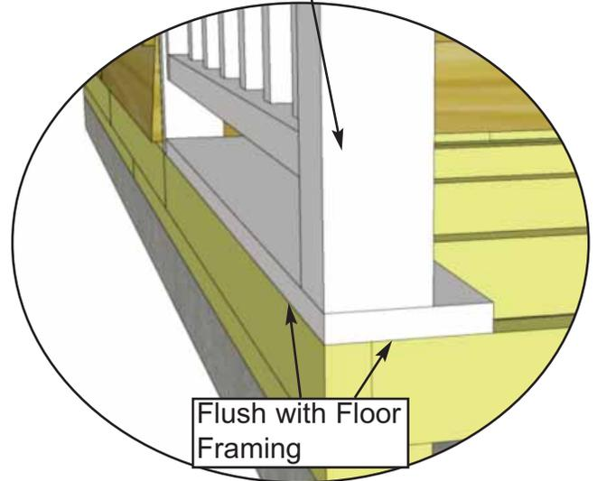
**21.** With the Porch Rail Sections complete, attach to the deck area as shown. Outer Deck Board will be positioned flush with the Floor Frame in the front corner. Fasten to Floor Joists with **4 - 2" Screws**. Pre-drill pilot holes before fastening screws. Complete other side the same.
