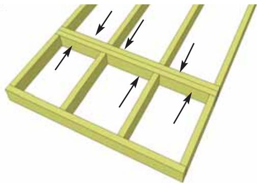
**4.** Attach each large and small floor joist frames together with **6 - 2 1/2" screws** per section.
