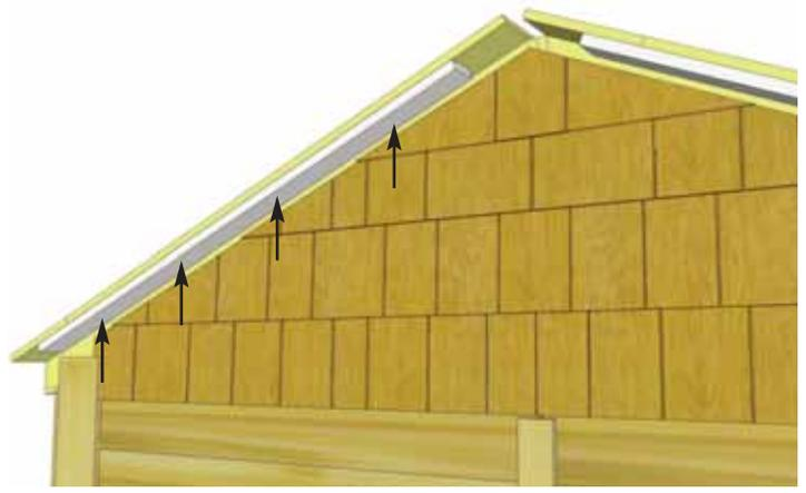
**71.** Attach two **Roof Nailing Strips** to the underside of the roof plywood on rear of shed. Align strips flush with plywood ends. Fasten with **4 - 1 1/4" Screws** per piece.
