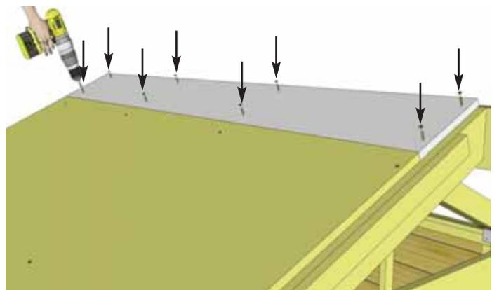
**53.** Locate one **Small Plywood Roof Panel** and position above the previous piece. Position tight against Large Roof Panel and attach with **8 - 1 1/4" screws**.
