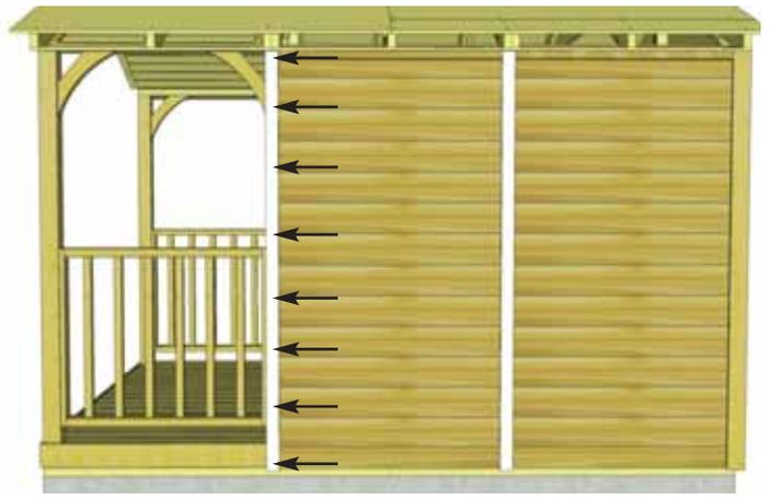
**66.** Attach four remaining **Narrow Trims** to both sides of the shed. Use **8 - 1 1/2" Finishing Nails** per piece.
