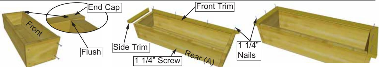
**2.** Position Front Frame Piece flush with End Cap. Attach both ends with 2 - 1 1/4" screws. Pilot hole Rear Box Frame near bottom center and secure to Base edge with 1 - 1 1/4" screw. Evenly position Front Trim (mitre cut on end and dado cut on inside bottom) tight against front frame and nail down with 4 - 1 1/4" nails. Position Side Trims as per Front and secure with 3 - 1 1/4" nails per side.
