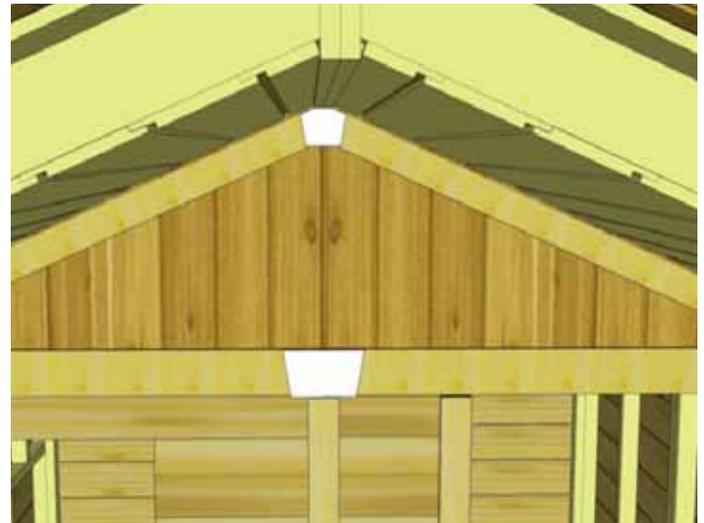
**70.** Position **Small Porch Detail Plate** and one **Facia Detail Plate** to cover trim seams. Attach with **4 - 1 1/2" Finishing Nails** per piece.
