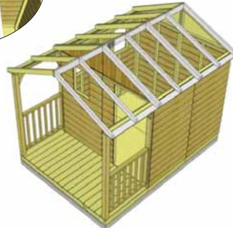
**43.** Place 2nd completed **Rafter** Section on gable wall framing. Position as per **Steps 39 - 42**.
