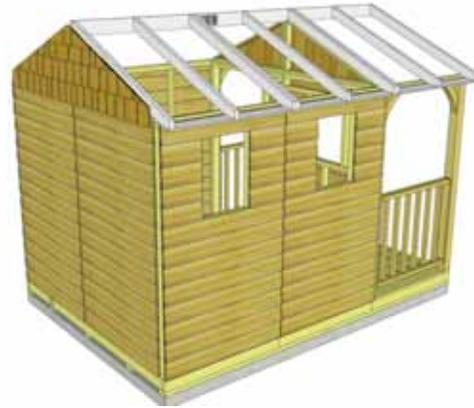
**42.** When **Rafter** Section is aligned correctly, tack **Rafter** Section temporarily down from **Middle Gable Wall** framing into **Rafter** with **2 - 2" screws**.
