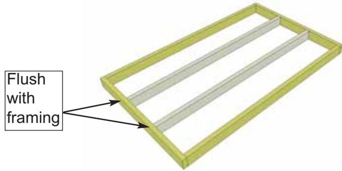
**1.** Lay out **Large Floor Joist Frame** and **2 Floor Joists** as illustrated above. Position Joists equally in Floor Joist Frame. Use **Small Floor Joist Frame** as a template to determine joist position. Position Joist so flush with framing.
