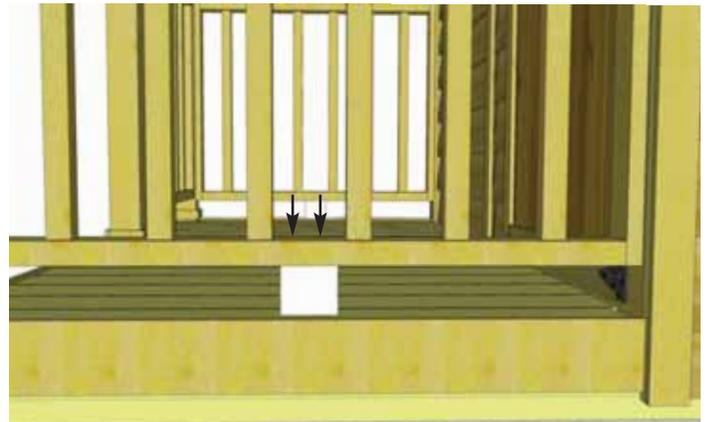
**91.** Place **Handrail Support Blocks** beneath Handrails, centered side-to-side and front-to-back. Attach each block with **2 - 2 1/2" screws** through the Handrail bottom.
