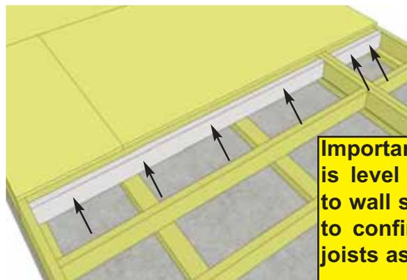
**Important:** Make sure floor is level before moving on to wall section. Use a level to confirm and shim floor joists as required.
