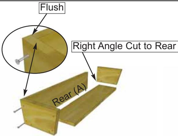
**1.** On a table position Rear Box and End Cap Frames together so flush at top. Fasten together with 2 - 1 1/4" screws. Place Base Frame tight against Rear and End Cap and flush at bottom. Secure with 2 - 1 1/4" screws. Complete attachment of remaining End Cap Frame. Slide Front Frame between End Caps.
