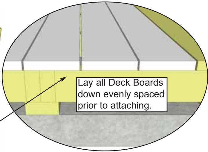
**22.** Attach remaining 15 **Deck Boards** using **4 - 2" Screws** per piece. Equally space all deck boards before attaching. Ensure screws enter the floor joists beneath deck boards. Pre-drill for screws at the ends of the deck boards.
