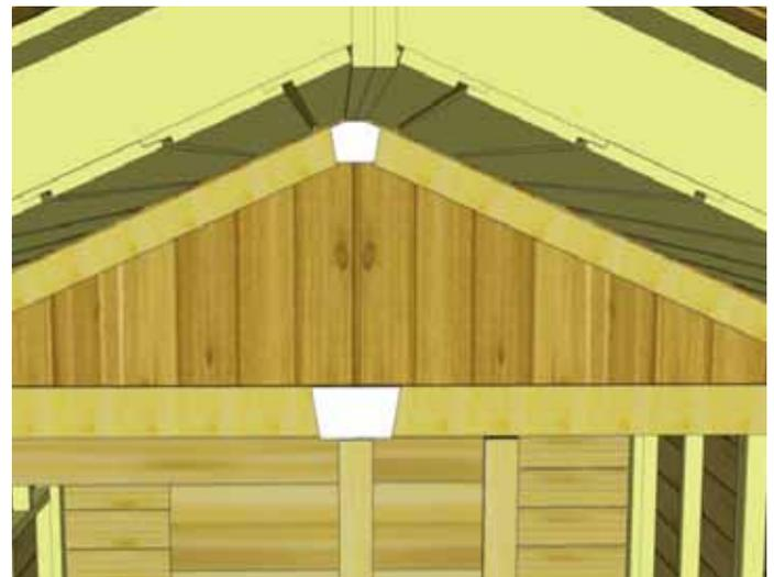
**81.** Position **Small Porch Detail Plate** and one **Facia Detail Plate** to cover trim seams. Attach with **4 - 1 1/2" Finishing Nails** per piece.
