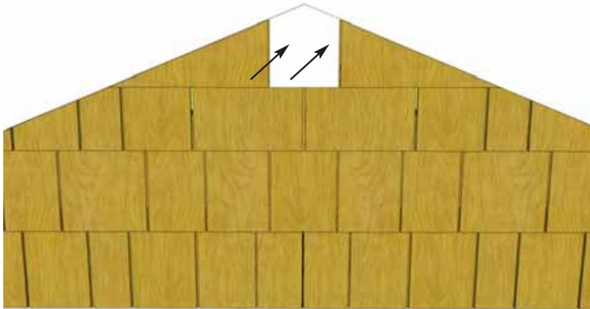
**31.** From the outside, slide in a Rear Gable Wall Filler Shingle to cover gable seam. Nail down above the exposure line with **2 - 1 1/2" Shingle Nails**.
