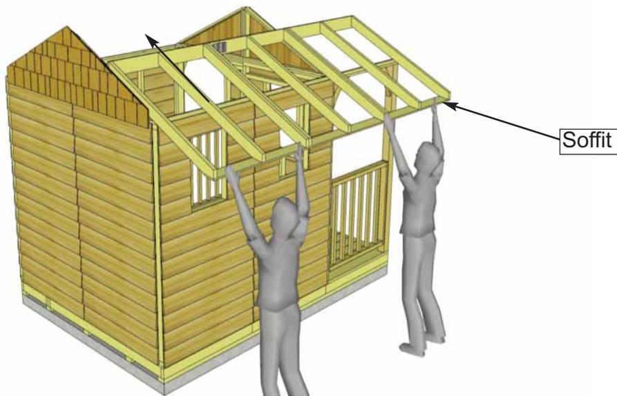
**39.** Carefully lift 1 completed **Rafter** Section up (make sure **Soffit** is facing down) and place on gable framing.
