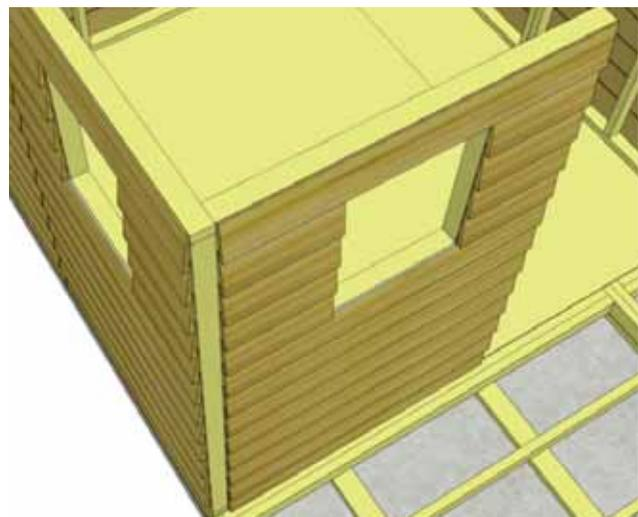
**17.** When attaching front corner wall panel, make sure panel is nested inside the side panel. Line up wall framing and secure at top, middle and bottom of wall studs.
