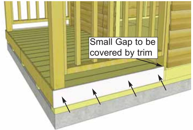
**71.** Position **Porch Side Bottom Skirting** on the side of the shed. The piece on the porch section will overlap the Front Skirting. When aligned there will be a gap on the shed side of the porch, this will be covered by trim pieces in **Step 77**. Attach with **4 - 1 1/2" Finishing Nails** per piece.
