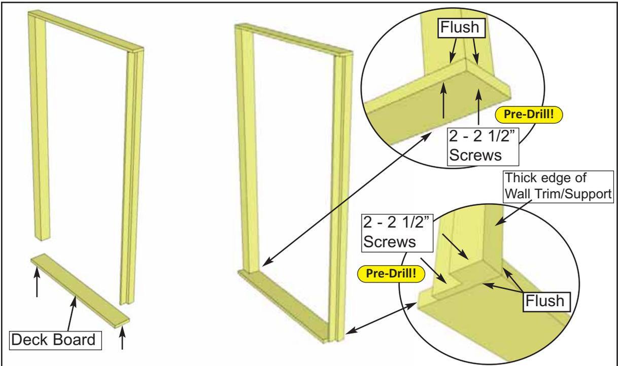
**C.** Attach **Outer Deck Board** (1" x 5 1/2" x 44") to the Wall Trim/Support with **2 - 2 1/2" Screws** fastened horizontally as shown above. Ensure Deck Board is flush with the thick edge of the Wall Trim/Support. Attach Outer Deck Board to the Long Porch Post with **2 - 2 1/2" Screws** fastened vertically as shown above. Ensure Deck Board is flush with corner of Long Porch Post.
