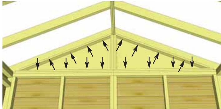
**46.** With both **Ridge Boards** connected, completely secure **Rafters** to Rear **Gable** framing of **both rear and middle Gable Walls**. Use **8 - 2" screws**.
