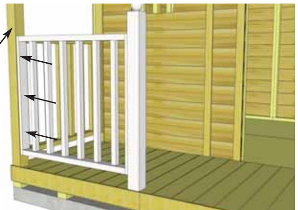
**91.** To complete porch, attach **Short Deck Post** and **Handrail Section** together with **3 - 2" Screws**. Measure **3 1/2"** from bottom of post to align rail. Place Post/Handrail section on deck. Attach rail to Porch Post with **3 - 2" Screws**.
