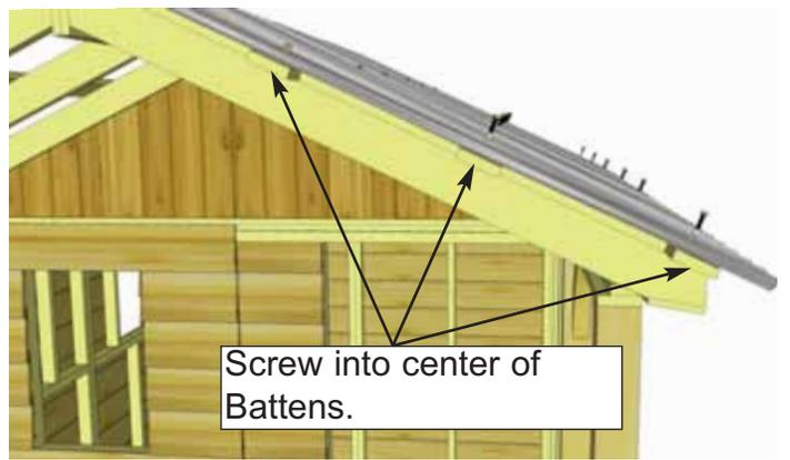
**63.** Using **12 - 2" Metal Screws** and 1/4" Nut Driver, secure **Metal Roof Panels** down to lower 2 rows of **Battens**. Leave the top row unsecured for now to secure Ridge Cap later in **Step 66**. Tighten screws in middle row that were partially secured in **Step 61**. Do not overtighten!
