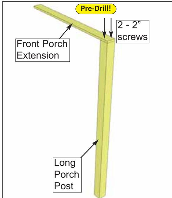
**A.** Attach **Front Porch Extension** (3/4" x 3 1/2" x 45 1/2") to **Long Porch Post** (3 1/2" x 3 1/2" x 73 7/8") with **2 - 2" screws**. Make sure support is flush with post.
