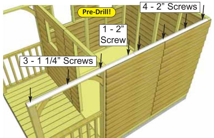
**26.** Attach the 4 **Side Top Plates**. The side top plates are angle cut down the length. Once again, position top plate on wall plate so it is flush with inside of wall plate. Side plate should also be flush with rear wall plate. Secure with:
