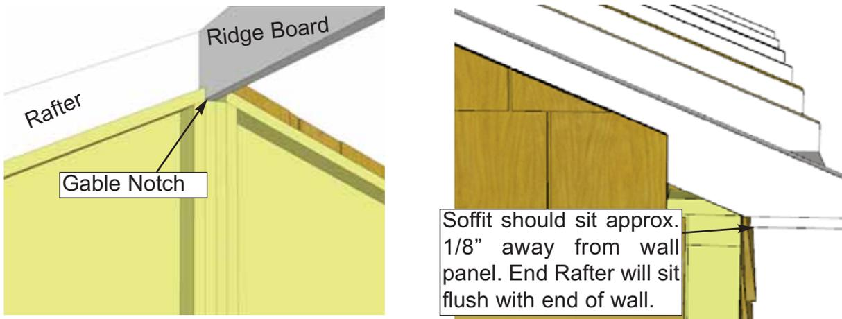
**40.** Slide **Rafter** Section up on gable framing until bottom of **Ridge Board** slips into gable notch. **Soffit** will sit approximately 1/8" away from wall panel.
