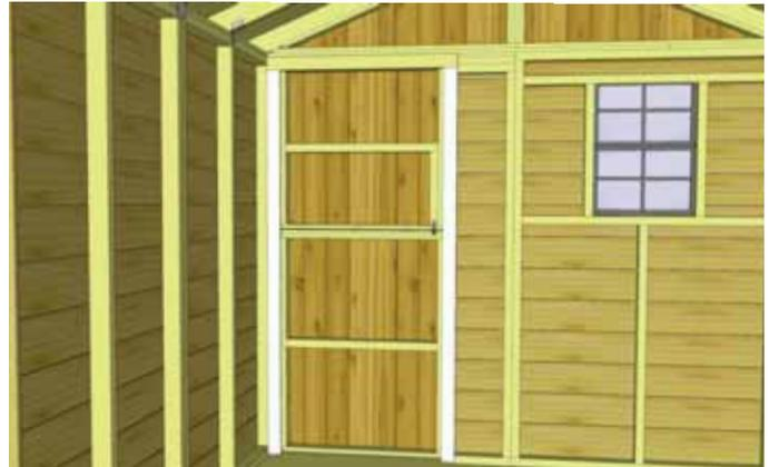
**100.** Attach **Horizontal Door Stop** and **Vertical Door Stops** to door jamb and wall framing. Use **4 - 2" screws** to secure **Horizontal Stop**, and **6 - 2" screws** per **Vertical Stop**. Door Stops should overhang the door by approximately 1/2". Start with the Horizontal Stop first.
