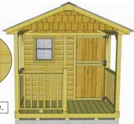
**98.** Place the **Top Dutch Door** panel into place and gap top and bottom trims on the outside about 1/8" apart/ On the inside, horizontal door frames should be about 1/4" apart. Use a shim once agin to help you. Attach hinges to trim with **2" Black Headed Screws** provided.
