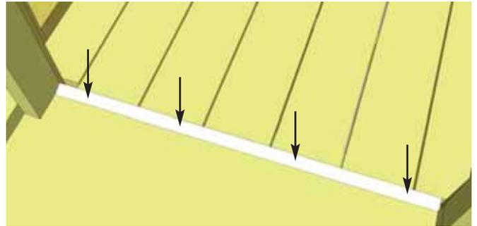
**29.** At the doorway of your shed there will be a small gap between the deck boards and floor plywood. Fill this gap with the **Doorway Floor Transition Strip** - angle edge cut and attach with **4 - 1 1/2" Finishing Nails**.
