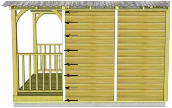
**77.** Attach four remaining **Narrow Trims** to both sides of the shed. Use **8 - 1 1/2" Finishing Nails** per piece.
