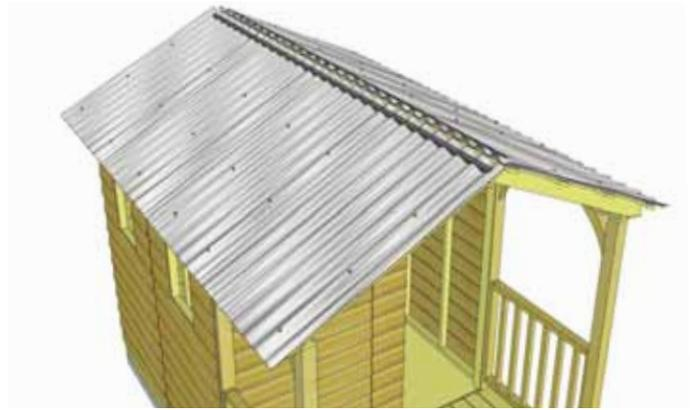
**65.** Locate remaining **Foam Enclosures**. Place **Foam Enclosures** at the top of roof panels. **Foam Enclosures** prevent moisture from coming in through the top of your shed.
