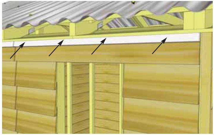
**73.** Trim out side walls by attaching **Top Wall Trim**. Position with thick end of Bevel downwards at top of wall, tight against Soffits. Attach with **4 - 1 1/2" Finishing Nails** per piece. Complete both sides
