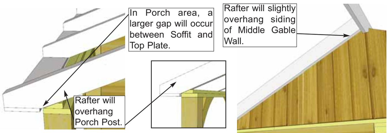
**41.** To confirm **Rafter** Section alignment - in the front, **Rafter** will overhang **Porch Post** by slightly". **Rafter** will also overhang the siding of Middle Gable Wall.
