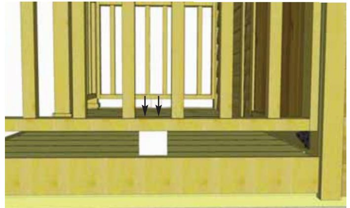
**102.** Place **Handrail Support Blocks** beneath Handrails, centered side-to-side and front-to-back. Attach each block with **2 - 2 1/2" screws** through the Handrail bottom.
