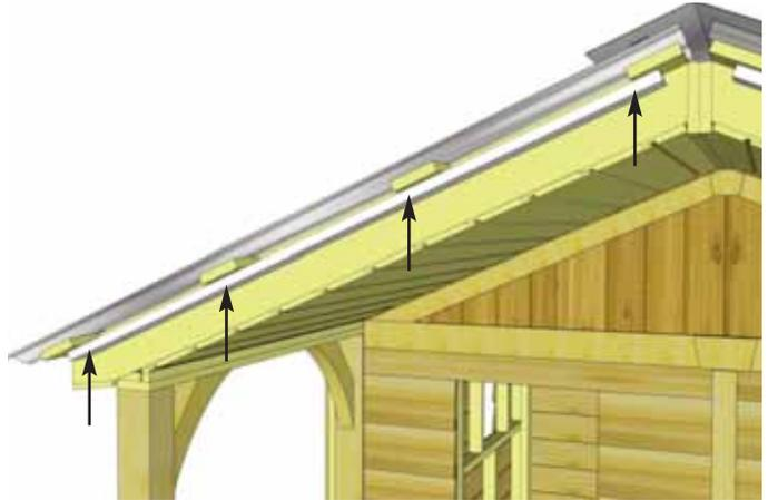
**83.** Attach remaining two **Roof Nailing Strips** to the underside of the roof plywood on front of shed. These strips will be pushed tight against the rafters unlike the Rear Nailing Strips. Fasten with **4 - 1 1/4" Screws** per piece.
