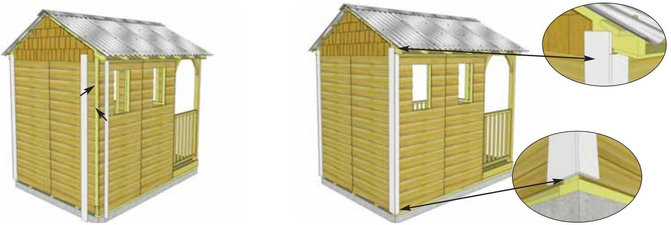
**75.** Position **Corner Trim** in rear corner and **Wide Corner Trim** over **Filler Trim**. Prior to attaching, do a dry run with Narrow Trim butted up tight underneath the Soffit. Position Wide Trim evenly with Narrow Trim at bottom. Narrow Trim will cap Wide Trim. Attach with **8 - 1 1/2" Finishing Nails** per piece. Repeat for other opposite rear corner.
