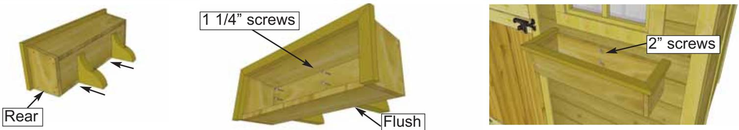
**3.** On a flat surface, flip Flower Box on it's rear face. Evenly space Brackets and secure through Base Frame and into the Brackets with 2 - 1 1/4" screws per Bracket. Position completed Flower Box beneath window trim and screw from inside of box into the center wall stud with 2 - 2" screws. (2" screws supplied with Base Kit.)
