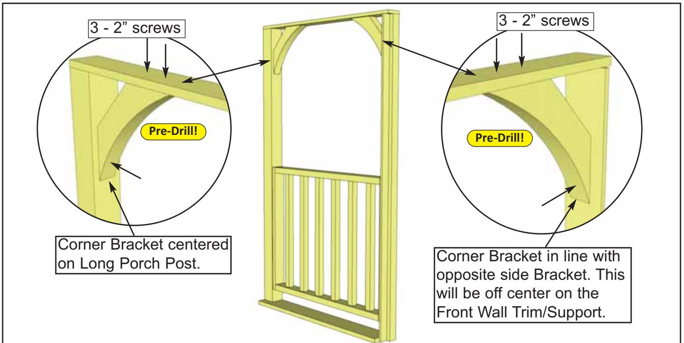
**E.** Position **Corner Bracket** centered on the Long Porch Post as shown. Position opposite side Corner Bracket in line with first. Attach each Corner Bracket with **3 - 2" Screws**. Fasten two screws down through Front Porch Extensions into Bracket, and the third screw horizontally through the bottom of the Corner Bracket. Drill Pilot holes before screwing to prevent splitting.
