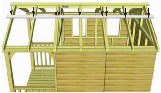
**54.** Locate **2 Outside Roof Battens** and **1 Inside Roof Batten**. Place outside Battens flush with Batten Spacers and overhanging outside Rafter by  $3 \frac{3}{4}$ ". Secure row of Battens to Rafters with **9 - 1 1/4"** screws (3 screws per Batten).
