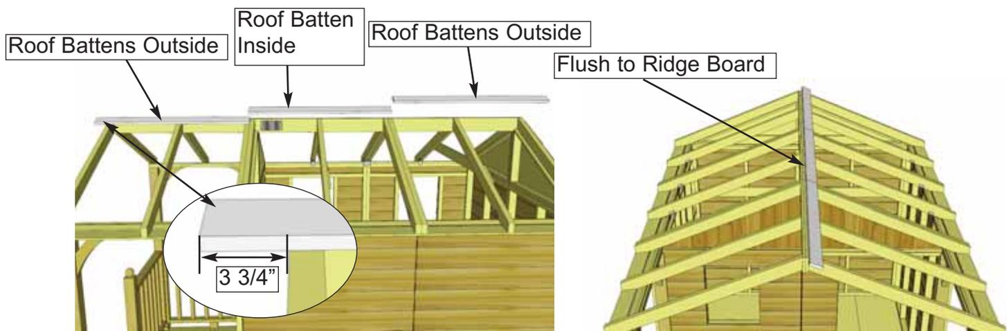
**51.** Locate 2 **Roof Battens Outside** and 1 **Roof Batten Inside** and place on roof Rafters. Place at top of Rafter section where Rafters and Ridge boards meet. Battens should be positioned with each end touching a doubled Rafter. Battens will overhang outside Rafters by 3 3/4".
