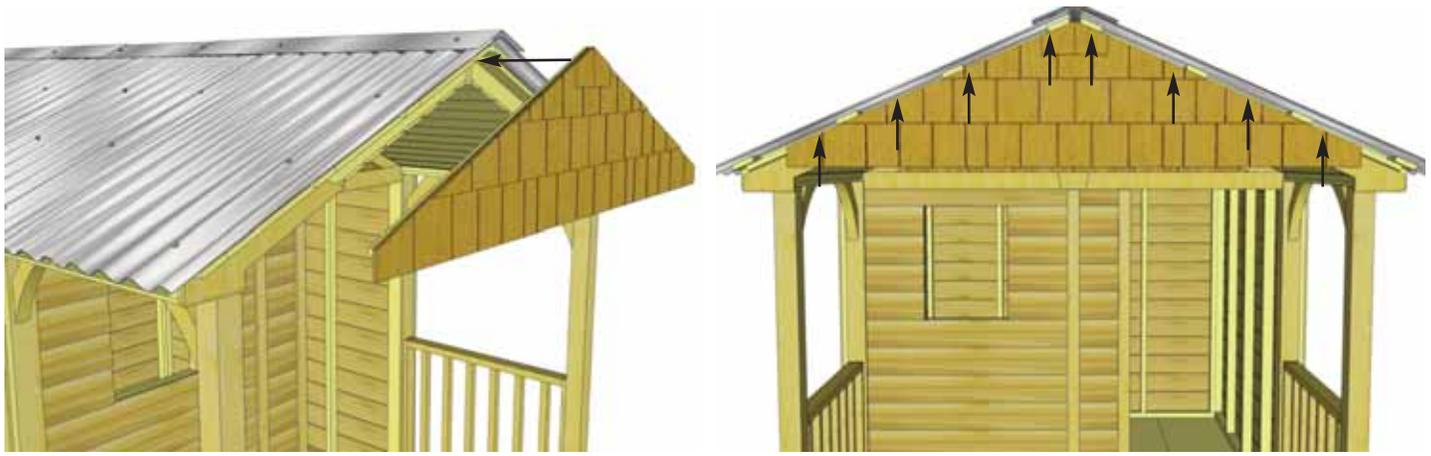
**85.** Position the **Gusset Gable** onto the front of the shed. Push Gable plywood up tight under roof plywood and against Roof Nailing Strip. Screw through the shingles of the Gusset Gable horizontally into the Roof Nailing Strip with **8 - 2 1/2" screws**.
