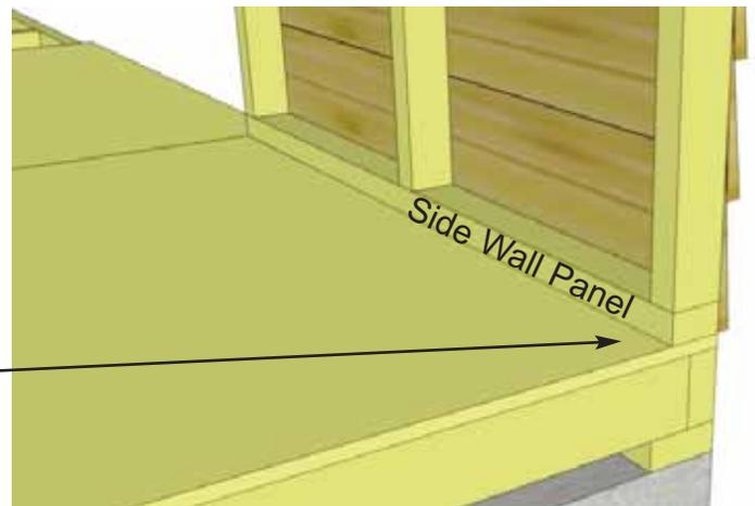
Outside 2x3 Plate of wall panel is flush with outside of floor frame when properly aligned. Floor plywood may be slightly recessed.
