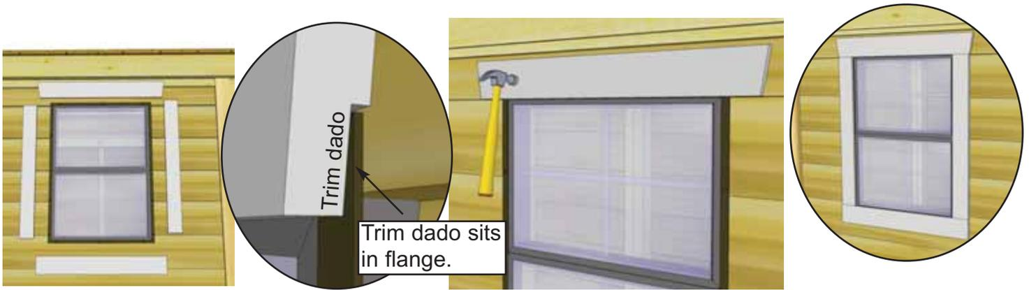
**95.** Position **Window Trim** around window doing a dry run first and attach with **4 - 1 1/2" Finishing Nails** per piece. Window trim has a small dado on reverse face. Outside flange of window will roughly sit in the dado to give a better fit.
