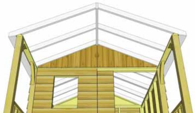
**44.** When both **Rafter** Sections are correctly aligned, **Ridge Boards** will sit in both the rear and middle gable notches. Front **Rafters** will overhang **Porch Posts**.
