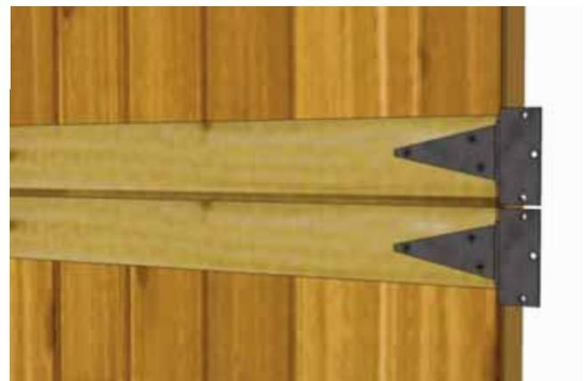
**96.** Attach Door hinges to Top and Bottom **Dutch Door** sections. Top Door has trim overhanging door at bottom while bottom door has trim recessed slightly. Hinges should be centered on door trim with barrel nudged to end of trim. Use **2" & 3/4" screws** as above.
