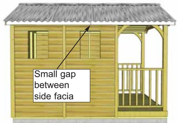
**88.** Attach **Side Facia** to rafter ends. There are 2 Facia pieces per side. A small gap may appear between Facias, which will be covered in **Step 79**. Secure with **8 - 1 1/2" Finishing Nails** per piece.
