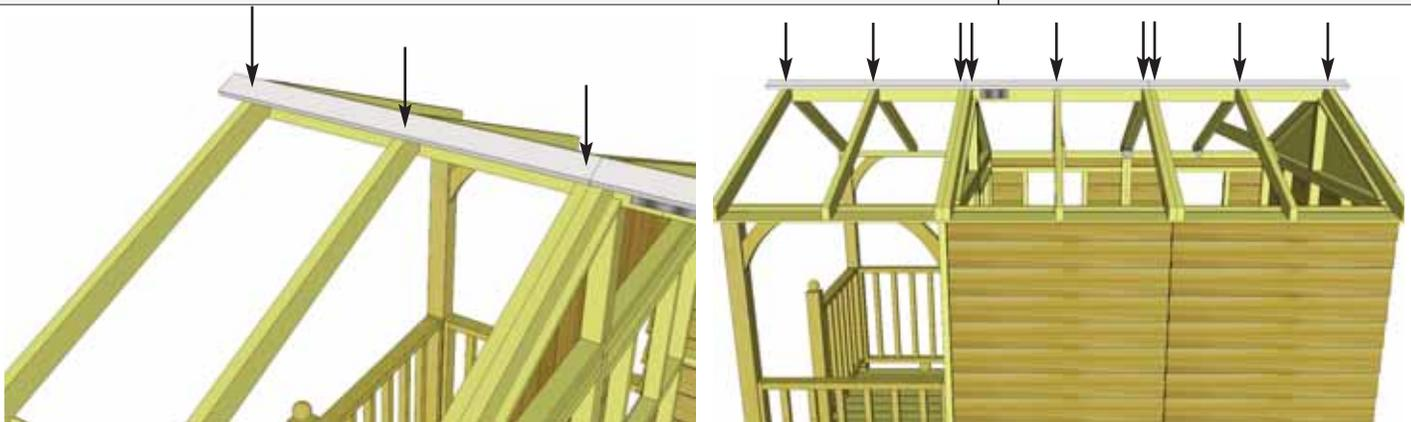
**52.** Attach each **Batten** to Rafters with 3 - 1 1/4" screws per Rafter section. **Important:** pre-drill pilot holes with 1/8" drill bit first to prevent splitting.
