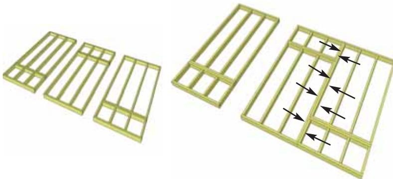
**5.** Complete all large and small frame attachments. Screw each completed section together with **8 - 2 1/2" screws**.
