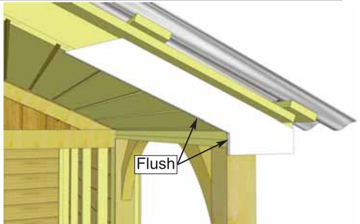
**84.** Position **Front Post Detail Covers** onto bottom corner of rafters, tight underneath Fascia Nailing Strips. Covers should be approximately flush with the bottom of the Porch Roof, the inside of the 4x4 Porch Post, and the Rafter ends. Attach with **4 - 1 1/2" Finishing Nails** per piece.
