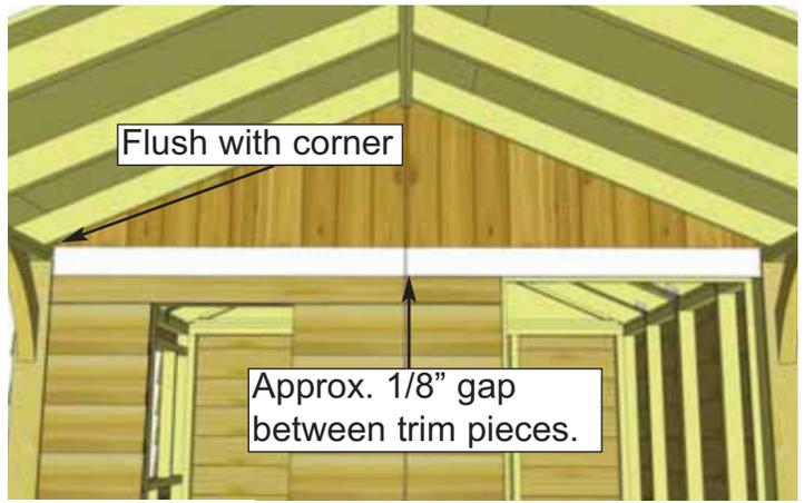
**67.** Attach **Horizontal Above Door Trim** with right side piece aligned flush with the top corner of doorway. Leave 1/8" gap between trim pieces, gap will be covered by a detail plate in **Step 81**. Attach with **4 - 1 1/2" Finishing Nails** per piece.
