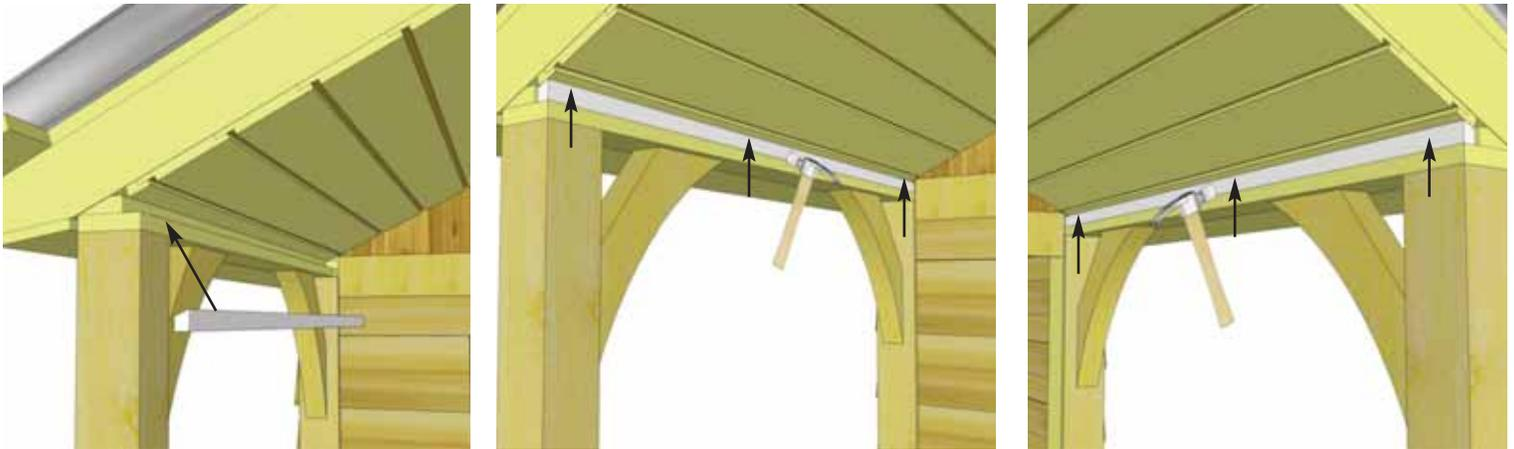
**69.** Insert **Porch Ceiling Support Strips** - Angle Edge Cut into the gap between the top of the Porch Rail Section and the Porch Ceiling Panel. Gently tap into place with a hammer. Once in place, attach each piece with **3 - 1 1/2" Finishing Nails** up through the Porch Rail Section into the Support Strips.
