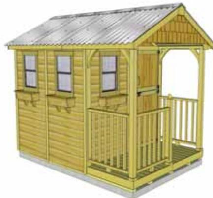
**103.** Assemble **Flower Box Kits** with Assembly Instructions included on Page 55. Position completed Flower Box below bottom of window trim and secure with **2 - 2 1/2" screws**. Screw from inside of box into the center wall stud. Attach second screw 2" underneath first screw and once again into the wall stud. Install Flower Box Kits underneath each window/double-window..
