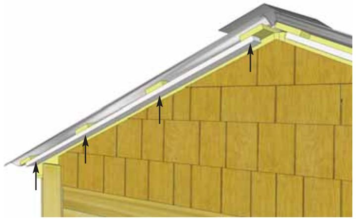
**82.** Attach two **Roof Nailing Strips** to the underside of the roof plywood on rear of shed. Align strips flush with plywood ends. Fasten with **4 - 1 1/4" Screws** per piece.
