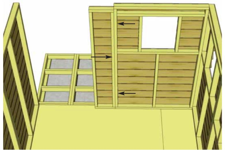
**18.** To complete walls, attach the **Narrow Porch Wall** to front wall panel. **Note:** the narrow wall is only 73" high. Attach wall stud to adjoining wall with **3 - 2 1/2"** screws.
