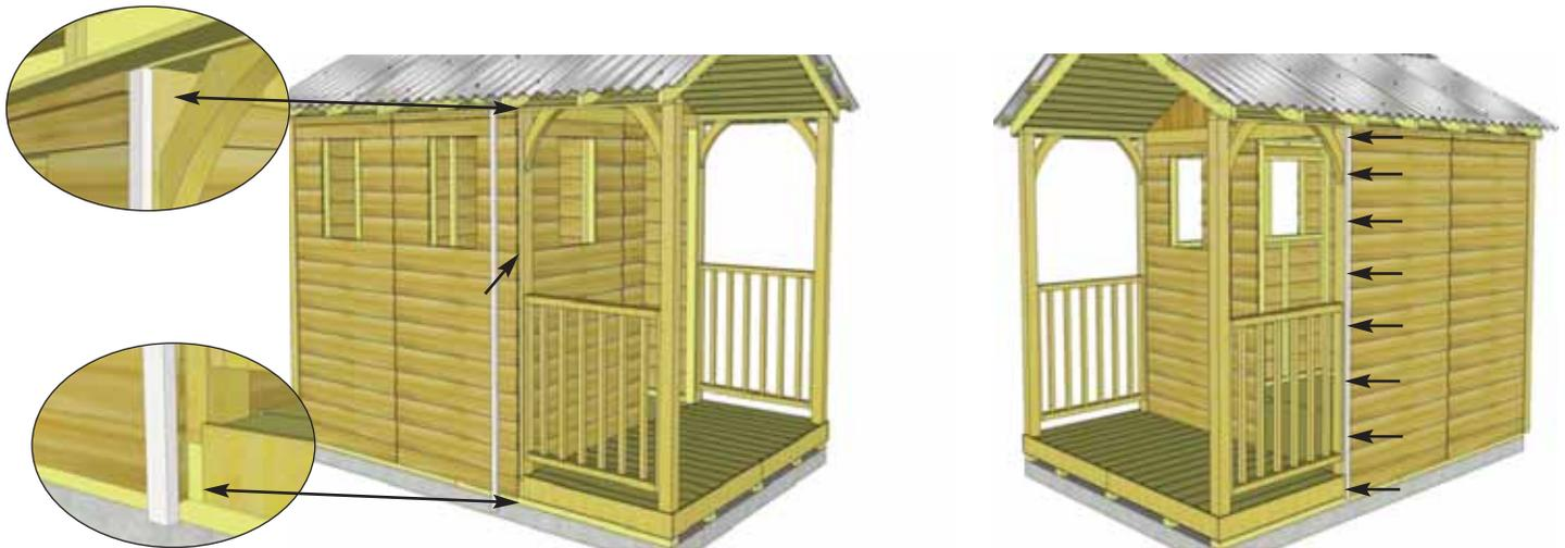
**76.** Position **Narrow Filler Trims** in gap between shed and porch. Attach with **8 - 1 1/2" Finishing Nails** per piece.
