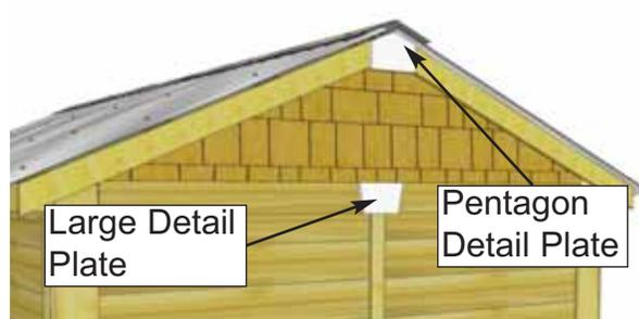
**90.** Attach two **Facia Detail Plates** and both **Pentagon Detail Plates** to cover seams where Facia pieces come together. Secure with **4 - 1 1/2" Finishing Nails** per piece.
