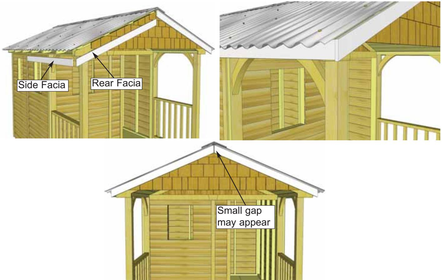
**87.** Position **Front Facia** - angle cut ends tight underneath roof shingles and tight against Nailing Strips. Temporarily position **Side Facia** for a dry run to help you correctly position Front Facia before attaching.
