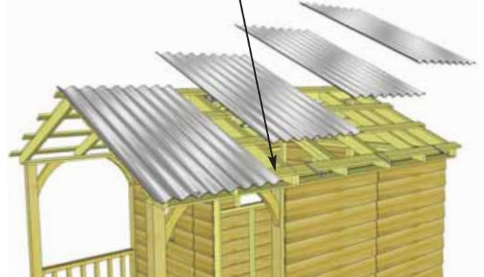
**58.** Locate 4 **Metal Roof Panels** and 4 **Metal Roof Hangars**. To temporarily hold the **Metal Roof Panels** in place, hook a **Metal Roof Hangar** onto the lowest Batten, approximately where the center of the panels will be. Place first **Metal Roof Panel** on Battens and into Hangar. Do not fasten panels down until **Step 62**. Place remaining 3 panels and hangars on the same way. Metal Roof Panels will overlap each other.
