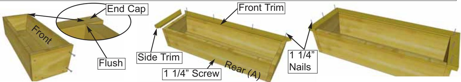
**2.** Position Front Frame Piece flush with End Cap. Attach both ends with 2 - 1 1/4" screws. Pilot hole Rear Box Frame near bottom center and secure to Base edge with 1 - 1 1/4" screw. Evenly position Front Trim (mitre cut on end and dado cut on inside bottom) tight against front frame and nail down with 4 - 1 1/4" nails. Position Side Trims as per Front and secure with 3 - 1 1/4" nails per side.
