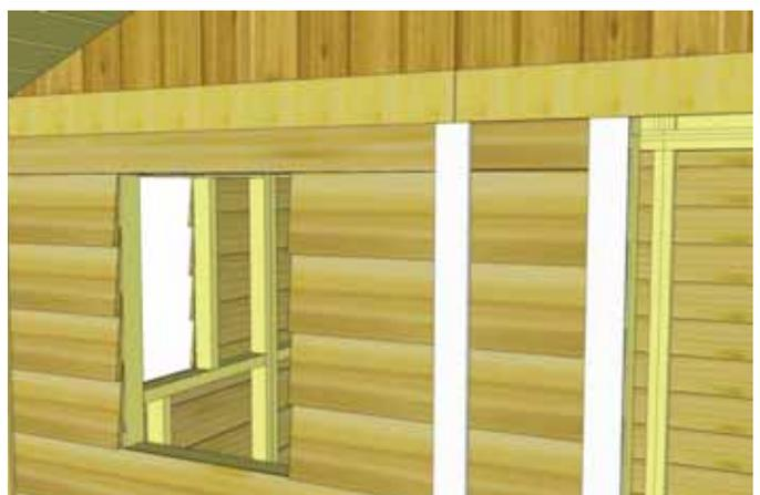
**79.** Attach both **Porch & Door Trims** to front walls. Secure with **6 - 1 1/2" Finishing Nails**.
