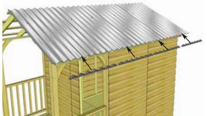
**62.** Before fully fastening **Metal Roof Panels** down, remove the **Metal Roof Hangars** and insert **Foam Enclosures** between **Metal Roof Panels** and **Battens** at the bottom of the roof. Enclosures will prevent moisture and unwanted bugs, etc from entering your shed through here.
