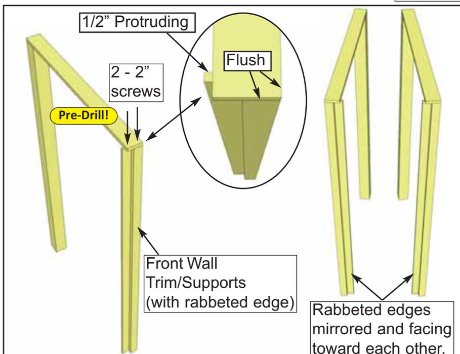
**B.** Attach **Front Wall Trim/Supports** ( 1" x 4" x 74 7/8") to Front Extension using **2 - 2" screws**. Make sure Front Extension is Flush to back and thick side of Wall Trim/Supports, and 1/2" protruding on thin side of Wall Trim/Supports
