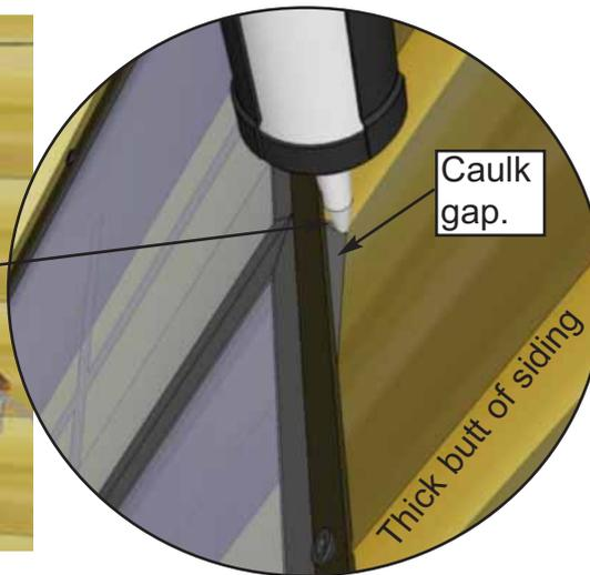
**94.** Once Insert is attached, caulk the "triangular gap" between the Insert's outside flange and the siding. Also put a bead of caulking horizontally at top of window where the flange and siding meet. This additional caulking will also will reduce the chances of moisture entering into your shed.
