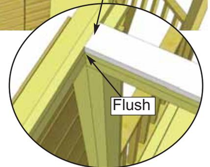
**27.** Position the **Front Top Plates** on top of Door Header and front wall panel. There are 2 plates (72" and 19" long). Front top plates are straight cut on the ends. Once again, the plate will be flush with inside of top wall framing. Attach with **6 - 2" screws** (4 screws in long and 2 in short plate).
