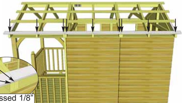
**56.** Locate another pair of **Batten Spacers** and position flush with third row of Battens. Attach Batten Spacers to outside Rafter with **2 - 1 1/4"** screws per **Spacer**. Locate 2 more **Outside Roof Battens** and 1 more **Inside Roof Batten**. Position Battens flush to **Batten Spacers**, **Battens** should be recessed  $\frac{1}{8}$ " from end of Rafters. Attach each **Battens** to Rafters with **3 - 1 1/4"** screws (9 total).
