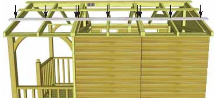
**55.** Locate another pair of **Batten Spacers** and position flush with second row of Battens. Attach Batten Spacers to outside Rafter with **2 - 1 1/4"** screws per **Spacer**. Locate 2 more **Outside Roof Battens** and 1 **Inside Roof Batten**, position Battens flush to **Batten Spacers**. Attach each **Batten** to Rafters with **3 - 1 1/4"** screws (9 total).
