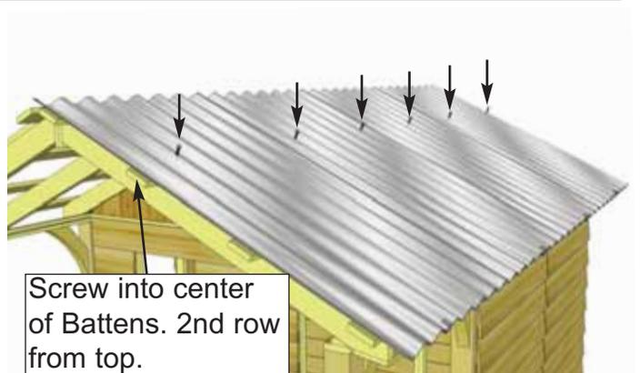
**61.** Using **6 - 2" Metal Screws** and **1/4" Nut Driver** (included), partially secure **Metal Roof Panels** to 2nd row of **Battens** from top. Only fasten screws halfway so that **Metal Roof Hangars** can be removed in **Step 62.** Metal screw is self-tapping, screw into center of Battens
