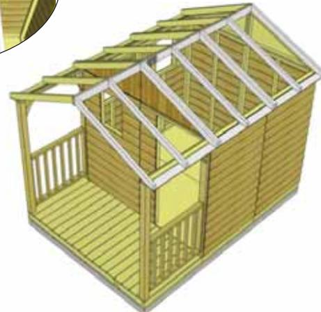
**43.** Place 2nd completed **Rafter** Section on gable wall framing. Position as per **Steps 39 - 42**.
