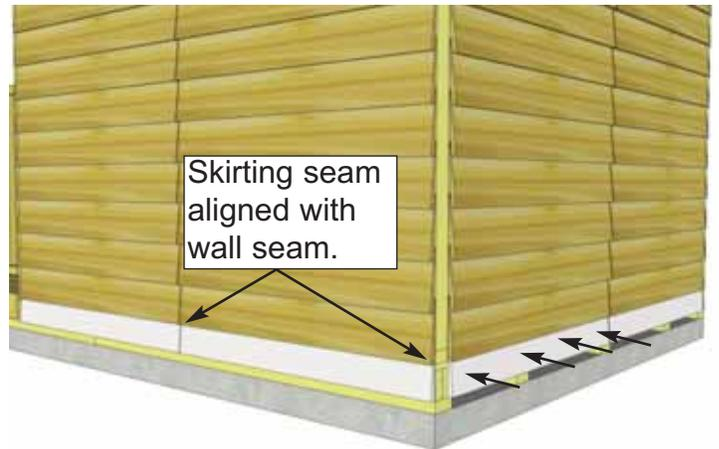
**72.** Position **Rear Bottom Skirting - Bevel** around the base of the shed. Bevel is thicker at butt and thinner at top of board. Skirting will hide floor framing. Gaps on side will be covered by Narrow & Wide Trim pieces later. Start on side walls first and attach with **4 - 1 1/2" Finishing Nails** per piece.
