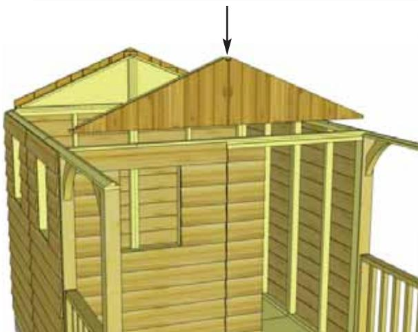
**34.** Position the **Middle Gable Wall** on top of front top plate. Middle gable has cedar siding on the front that is cut flush with gable framing. Once again, the framing of the gable should be flush with outside of plate and be centered sideways on the plate. When in correct position, attach with **2 - 2" screws** temporarily as per **Step 30**.
