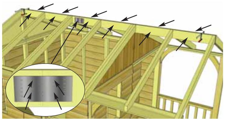
**45.** At the peak, align **Ridge Boards** so they are flush together and secure them with **12 - 1 1/4" screws**. To completely secure **Ridge Boards**, place **4 - 1 1/4" screws** into any of the remaining **Metal Ridge Board Connector** holes. Complete both sides. **Important:** If there is a gap between **Ridge Boards**, try pushing side walls closer together from outside. Walls should be 91" apart at top from inside of wall plate to wall plate.
