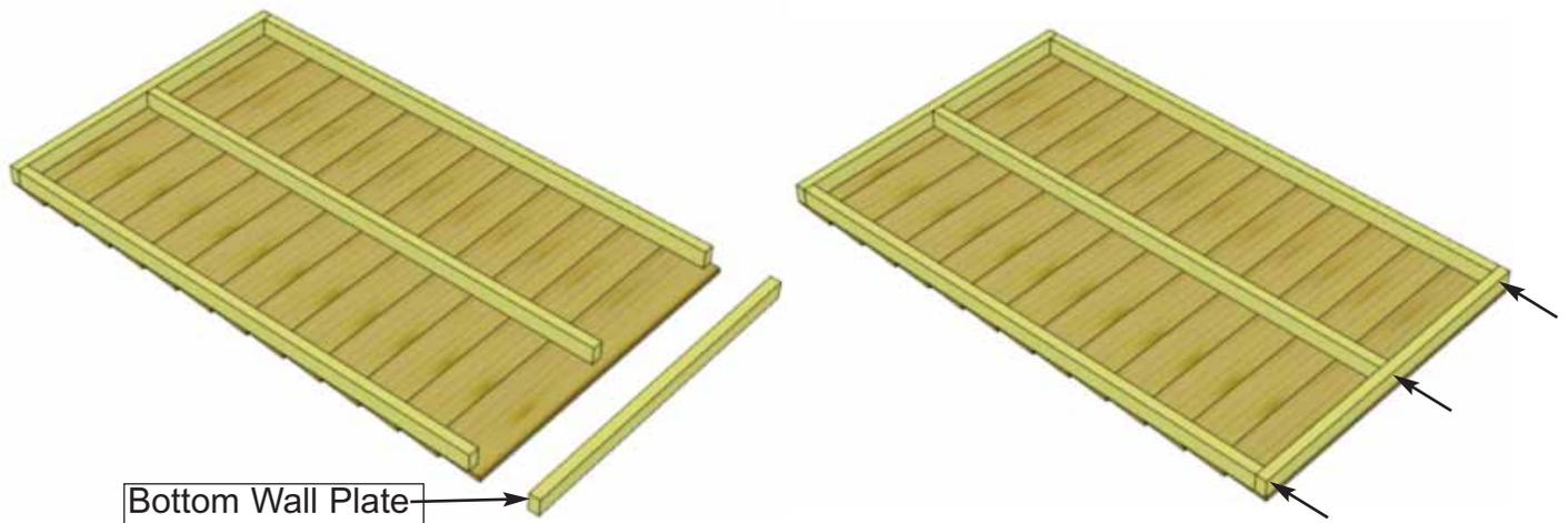
**13.** Starting with All **Solid Wall Panels**, carefully lay panel face down. Position and attach **Bottom Wall Plates** to bottom of wall studs of each wall panel with **3 - 2 1/2" screws**. Position so Wall Plates are flush with framing.
