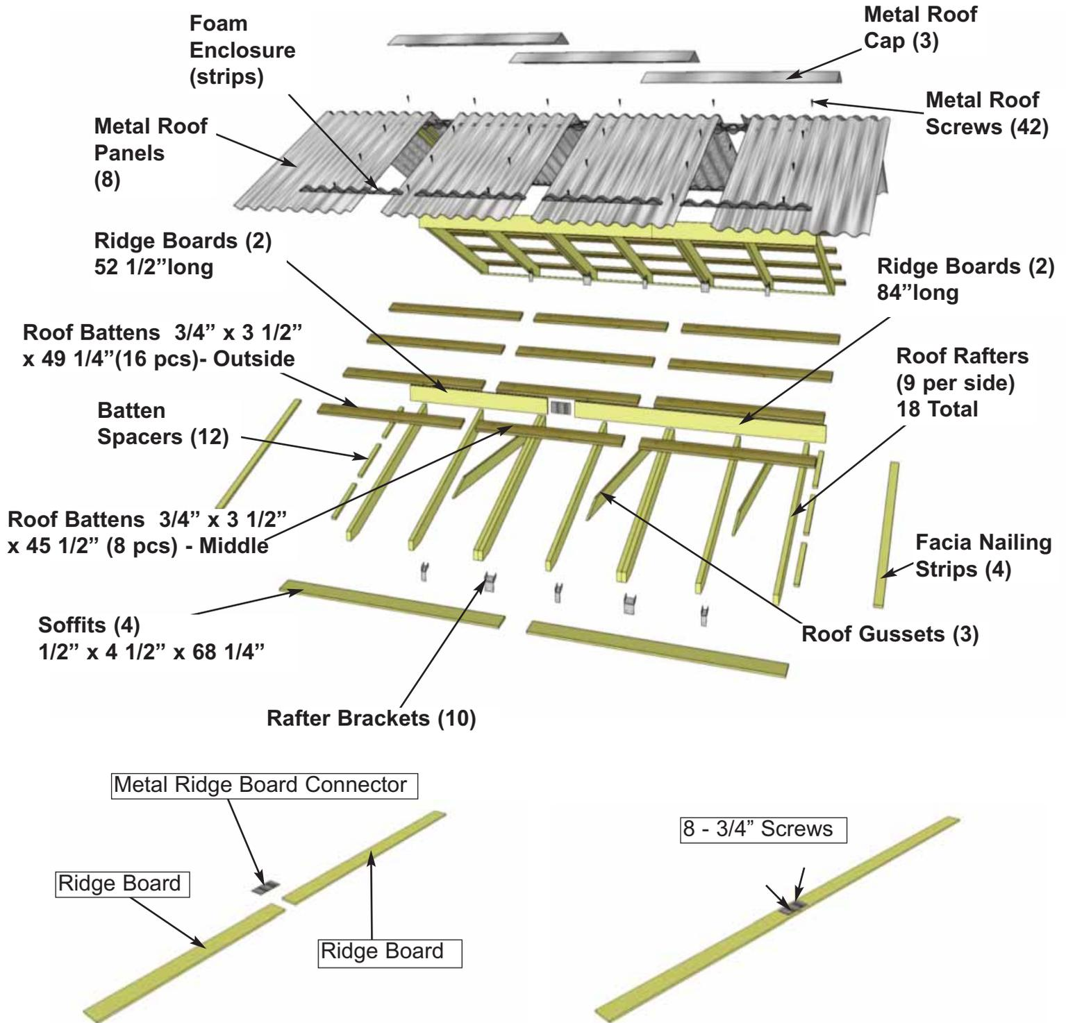
**35.** Locate **Ridge Boards Long & Ridge Boards Short** and attach together with **Metal Ridge Board Connector** using **8 - 3/4" silver screws**. Position **Metal Ridge Board Connector** evenly on **Ridge Boards**. Total length when connected is 136 1/2". Complete two sets.
