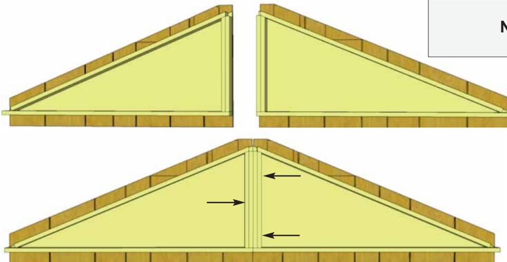
**30.** Locate both Rear Gable Wall pieces. Rear Gables have shingles that overhang the top and bottom of the gable frame. Screw together with **3 - 2 1/2" screws**.
