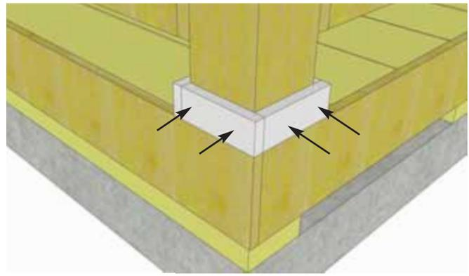
**101.** Attach **Post Base Trims** to bottom of porch posts. Attach with **2 - 1 1/2" Finishing Nails**.
