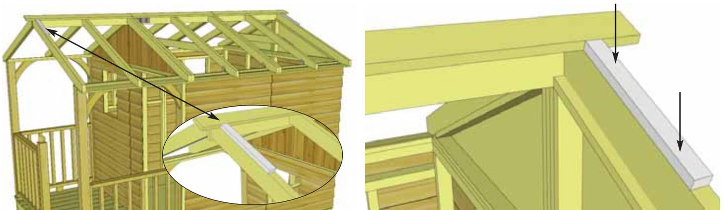
**53.** Place **Batten Spacer** flush with first set of Battens on outside Rafter. Batten Spacer allows you to line up next row of Battens. Attach each with **Batten Spacer** with 2 - 1 1/4" screws.
