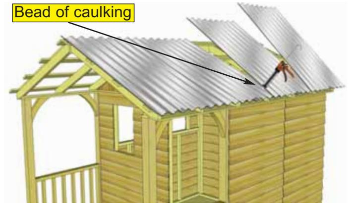
**60.** Once the Metal Roof Panels are spaced correctly from side-to-side and top-to-bottom, lift 3 panels up and run a bead of caulking down the overlapping seams of each panel to seal the joints. Place panels down one by one once seam is caulked. You will likely need assistance from a helper for this step. Caulk each seam.
