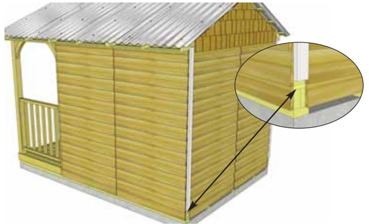
**74.** Attach **Rear Filler Trims** to rear walls, positioned flush with siding and bottom skirting. Attach with **8 - 1 1/2" Finishing Nails**.
