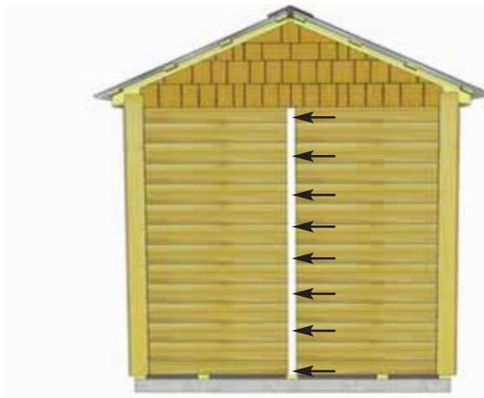
**78.** Attach **Rear Wall Seam Trim** where back wall panels meet. Secure with **8 - 1 1/2" Finishing Nails**.
