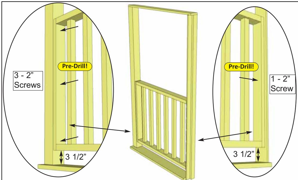
**D.** Attach a **Hand Rail Section** to the Long Porch Post. Hand Rail should start 3 1/2" from bottom of Post and be centered side-to-side. Use **3 - 2" Screws** to attach. Attach Hand Rail to Wall Trim/Support with **1 - 2" Screw** for now, more screws will be added when it is attached to the wall in **Step 28**.
