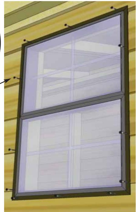
**93.** To reduce possible water from penetrating into the window cavity, caulk gap on both sides of window opening prior to installing **Window Insert**. Position insert in cavity and screw with **6 - 1 1/4" Screws**. On sides, make sure to screw insert into the thick butt of the siding only.
