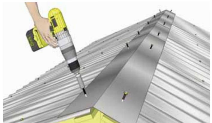
**66.** Place 3 **Metal Ridge Caps** onto apex of roof. Evenly space from front to back of your shed, Metal Ridge Caps will overlap each other. Overhang the cap approximately 1" - 2" past each end. When **Metal Ridge Caps** are correctly positioned, secure with **12 - 2" Metal Ridge Screws** (6 per side). Screw into center of final **Batten**. Do not overtighten!
