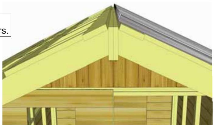
**59.** Overhang the **Metal Roof Panels** past the **Battens** on front and rear of shed by approximately 1". Adjust panels side-to-side to achieve desired width. Overall width past the **Battens** can vary from 1" - 3" depending on your preference. The overhang over the side of the shed will be set by the **Metal Roof Hangars**, but should be approximately 4" on side of shed.
