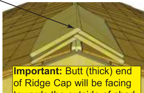
Alternate Ridge Cap seams (offsetting angle cut at peak)
