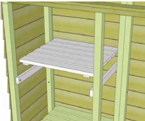
15. Complete positioning and attachment of second shelf as per Step 13 - 14.
