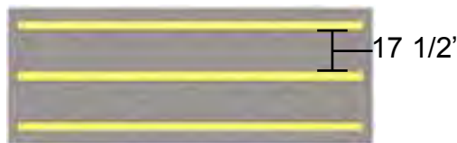
Gravel Foundation with treated stringers
