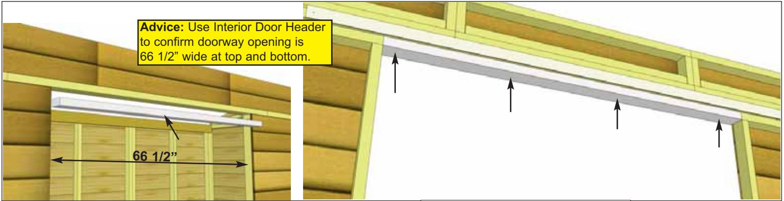
**23.** Attach **2E - Interior Door Header** as shown above. Align with top framing of front walls. Attach with **4 - 2 1/2" Screws**.
