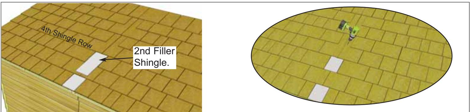
**39.** Slide 2nd **Filler Shingle** up and underneath fourth shingle row. Follow **Steps 37 - 38** to align and attach. Repeat for other roof seam.
