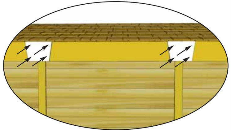
**65.** Attach **4U - Trim Detail Plates** to cover seams. Four Plates will cover seams where Front and Rear Facia pieces meet, attach these with **4 - 1 1/2" Finishing Nails** per piece. One more Trim Plate will cover the seam of the Track Overlay, attach with **3 - 1 1/2" Finishing Nails** along the top of the Plate so nails are secured to 2x4 backing.
