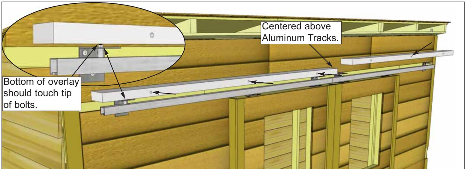
**54.** Install both **4KA - Track Overlay - Top** pieces above the aluminum tracks. Position pieces horizontally as shown above. Attach with **3 - 4" Screws** per piece through the pre-drilled holes.
