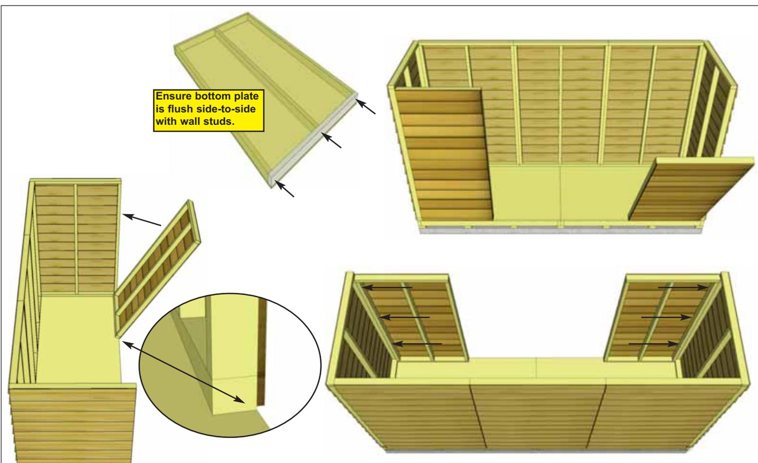
**13.** Carefully lay **2BA - Front Wall Panels** face down. Position and attach **2BB - Bottom Wall Plates** to bottom of wall studs of each wall panel with **3 - 2 1/2" Screws** as per **Step 7**. Complete other remaining Front Wall.
