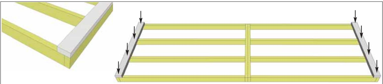
**3.** Position **1C - Floor Runners - Short** on each side of the completed floor frame. Runners should be flush with corners but not overhanging. Attach with **4 - 2 1/2" Screws** per Runner.
