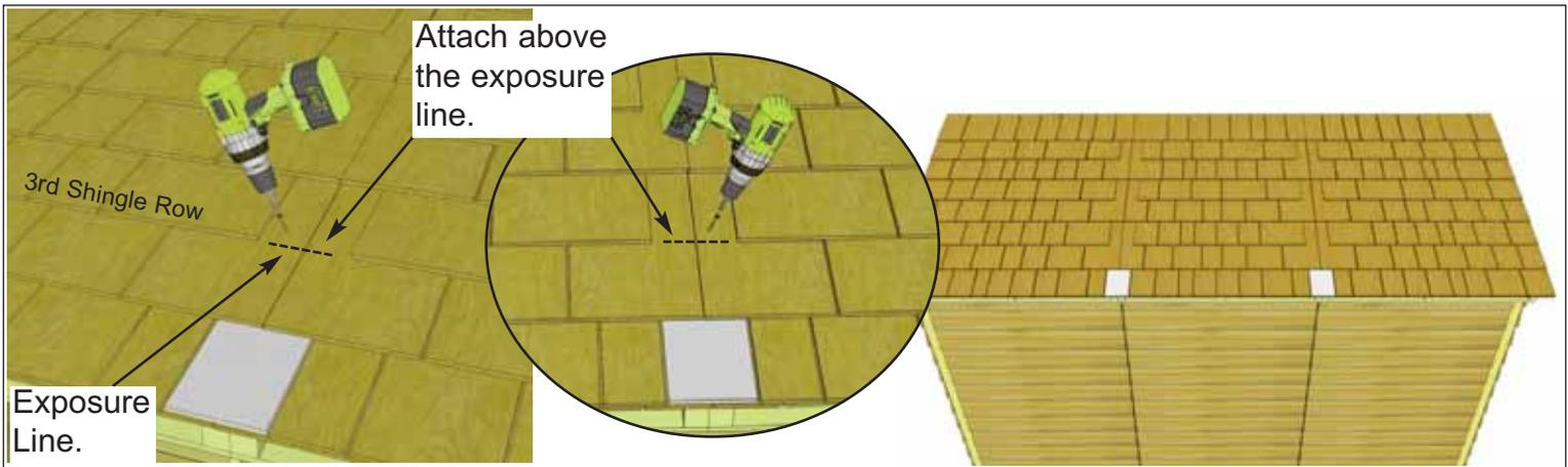
**38.** Screw first filler shingle down to rafters using **1 - 2 1/2" Screw** per panel (2 in total). Screw on slight angle and make sure to screw into rafter. Screw slightly above 3rd row of shingles (exposure line). This way, the screw will get covered up when you install your 2nd Filler Shingle and will prevent leaking. Do both roof seams the same.
