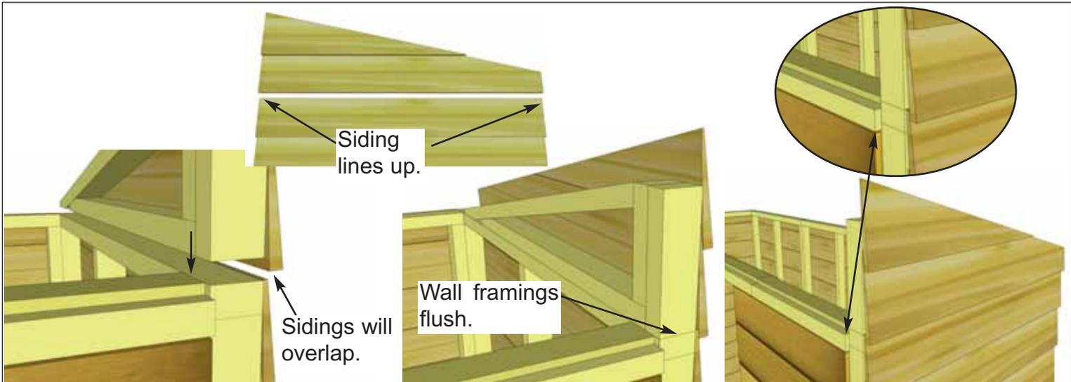
**17.** Align wall framing of Angled Wall Extender and Side Wall so they are flush at the front. The siding for both walls should also align evenly from front to back.
