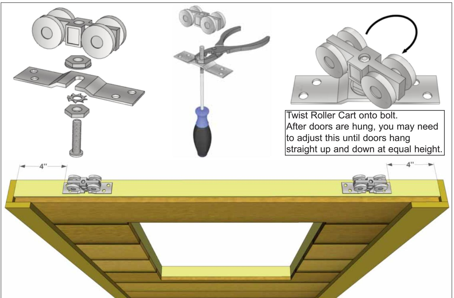
**50.** Locate all four **Y35 - Roller Assemblies**. Before attaching to top of doors, assemble the units as shown above. Attach two Roller Assemblies to each door with **4 - 1 1/4" Screws** per Assembly, center on the door framing **4"** from each end as shown above.
