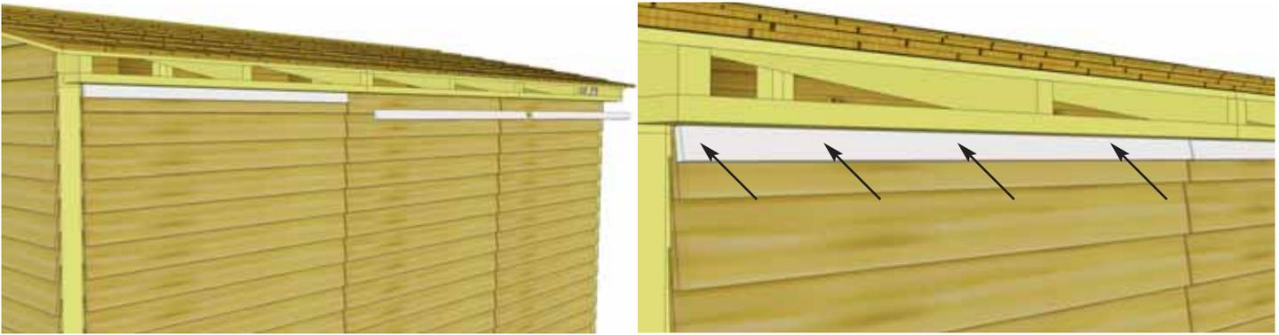
**46.** Trim out Rear Walls by attaching **Top Wall Trim**. Position with thick end of Bevel downward at top wall, tight against Soffits. Attach with **4 - 1 1/2" Finishing Nails** per piece.
