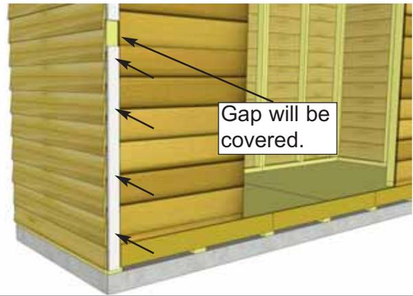
**47.** Position and attach **4C - Front Corner Filler Trim** with **4 - 1 1/2" Finishing Nails** per piece. Filler trims won't be visible because they serve as nailing strips for the Corner Trims which will be attached later.
