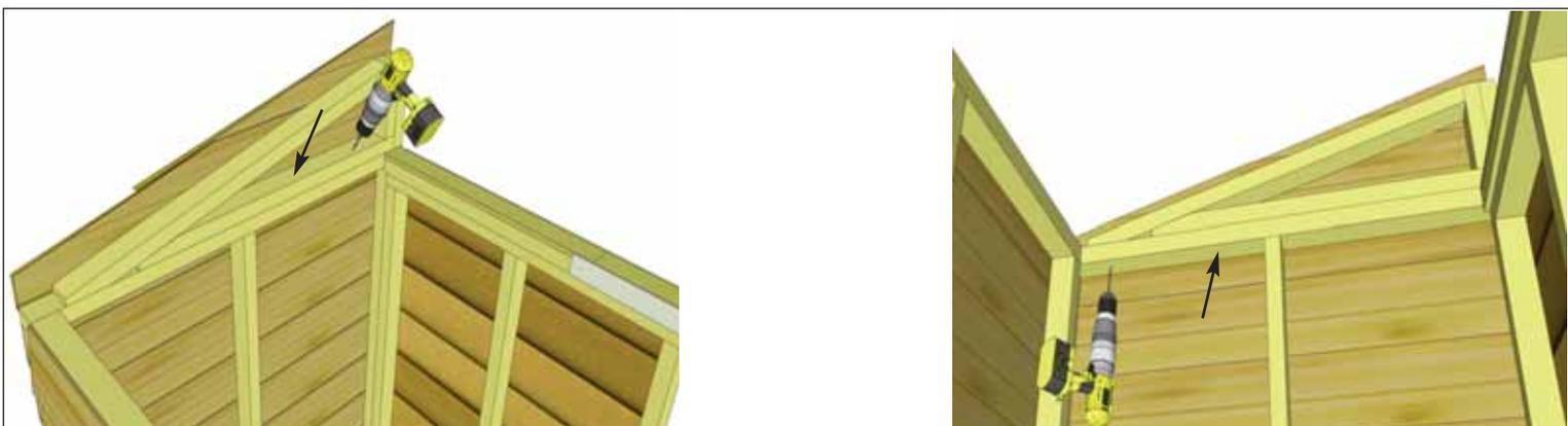
**18.** With Angled Wall Extender and Side Wall aligned correctly, secure together from the inside with **4 - 2 1/2" Screws**.
