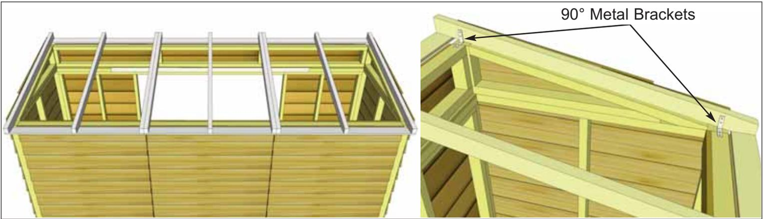
**29.** With Rafter Section correctly aligned, secure rafters to walls using **2 - 90° Metal Brackets** per side. Attach each brackets with **4 - 1 1/4" Screws**. Screw into Wall Extender framing at the front and Wall Panel top framing at the rear. Complete both sides.
