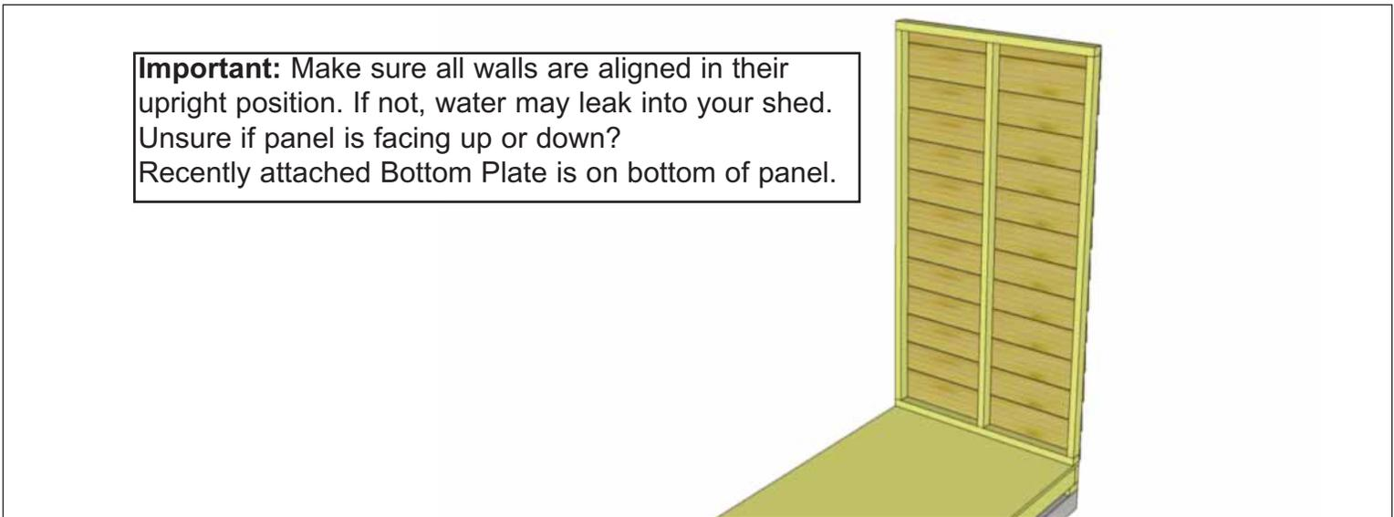
**8.** Starting on one side, position a Solid Wall Panel on top of plywood floor. The Wall Panel bottom framing will sit flush with the outside of the floor frame. Wall siding will overhang the floor.
