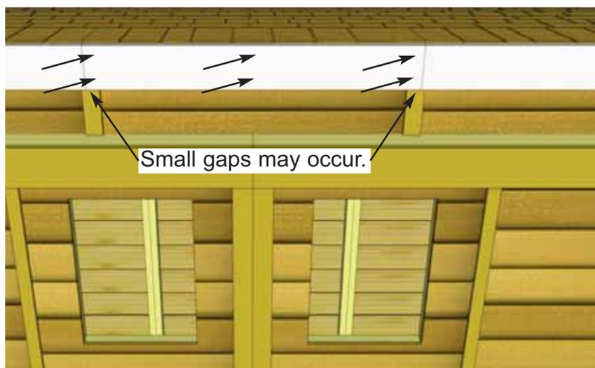
**63.** Attach **4T - Front Facia - Center** to rafter ends as shown above. Small gaps may occur between the Center and Left/Right Facia, but these will be covered by Facia Detail Plates in **Step 65**. Attach with **2 - 1 1/2" Finishing Nails** per rafter end.
