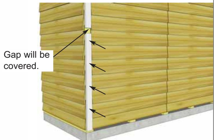
**48.** Position and attach **4D - Rear Corner Filler Trim** with **4 - 1 1/2" Finishing Nails** per piece as per **Step 47**.
