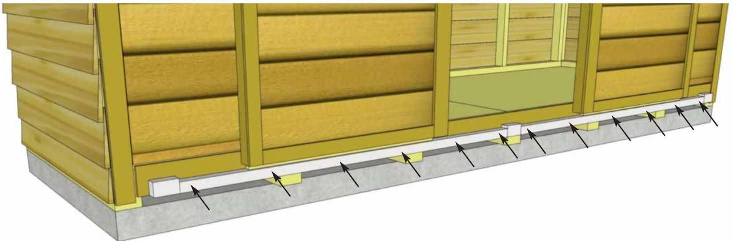
**51.** Locate **4G - Door Tracks** and **4IA - Door Stops**. Start with Middle Door Stop centered on middle Floor Runner and build out from there. Door Tracks rest on Long Floor Runners. Bottom of Door Stops and Door Tracks should be flush with each other. Secure Door Tracks to shed with **6 - 3" screws** per piece. Secure Door Stops with **2 - 3" screws** per piece.
