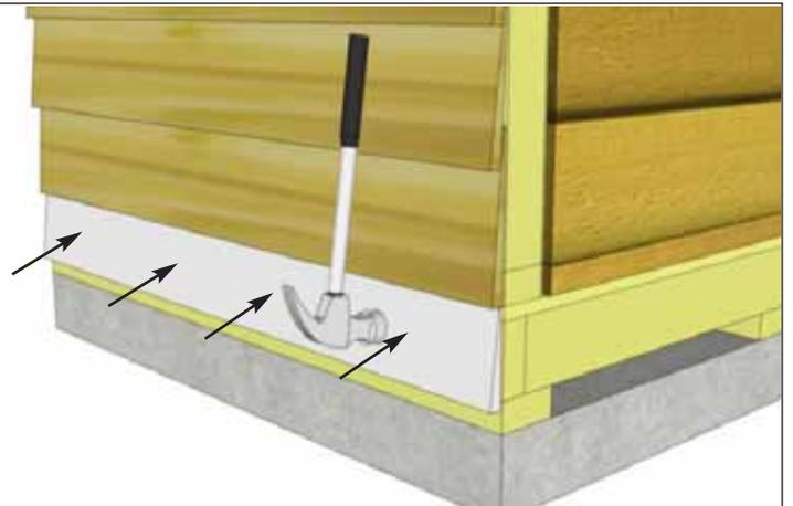
**43.** Attach **4A - Side/Rear Bottom Skirting** around the base of the shed. Skirting will hide floor framing. Start with side skirting pieces first and attach with **4 - 1 1/2" Finishing Nails** per piece.
