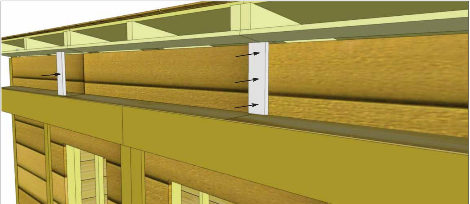
**60.** Attach **4Q - Front Middle Trims** above doors where front wall extenders come together above track. Attach with **3 - 1 1/2" Finishing Nails** per piece, aligning tight underneath soffit and centered on seam.
