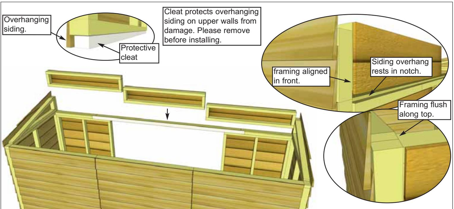
**20.** Place **2H - Extender Walls** on top of Door Header so that framing is aligned with Angle Wall Extender framing in front as shown above. With framing aligned, attach Extender Walls to Door Header and other extenders with **4 - 2 1/2" Screws** each as shown below.
