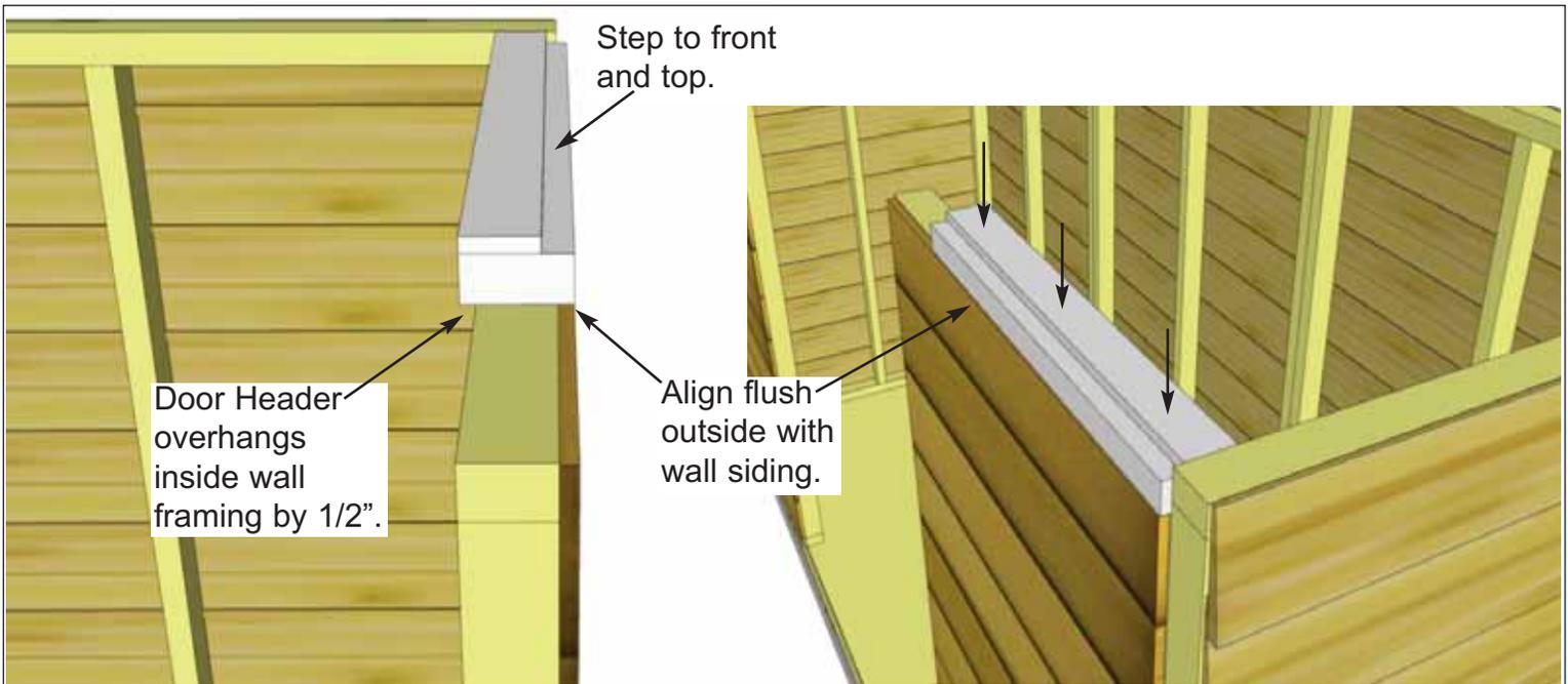
**14.** Position **2C - Door Header - Short** on top of wall stud so it is flush on the outside with the wall siding. Attach by screwing down into top wall framing with **3 - 3" Screws**.
