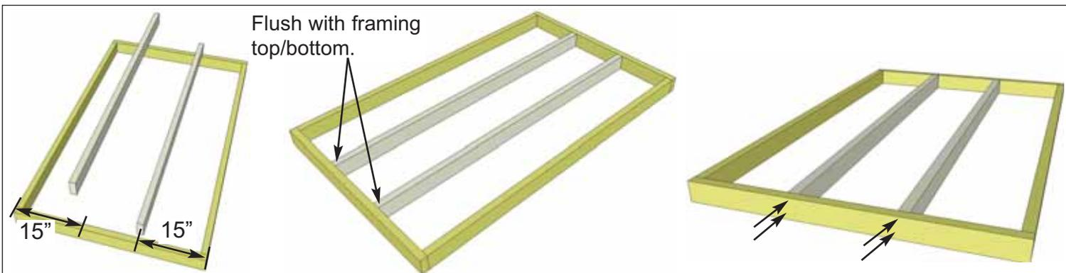
**1.** Lay out **1A - Floor Frame** and two **1B - Floor Joists** as illustrated above. Position the center of each Joist 15" from the outer edge of Floor Frame. When correctly positioned, attach each Joist with **4 - 2 1/2" Screws** (2 per end). **You can find the Square Drive Screw Bit in the Hardware Kit Bag.** Complete remaining Floor Frame the same.
