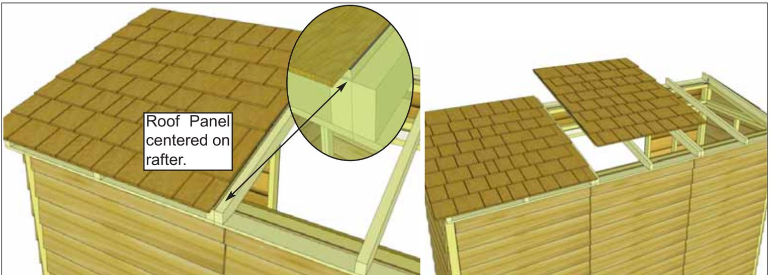
**33.** For correct Roof Panel position, align panel so plywood sits evenly on Center Rafters. Next, position **3H - Center Roof Panel** onto center rafters.
