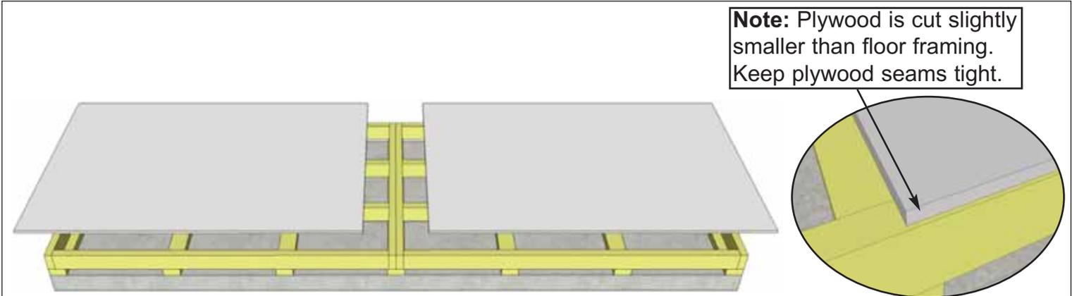
**5.** Position **1D - Plywood Floor** on top of completed floor frames. Plywood will sit slightly inset from outside of floor frame.
