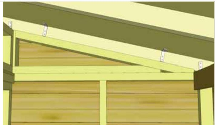
**41.** Secure roof panels to walls at both ends by positioning **2 - 90° Metal Brackets** on plywood and outside rafters and securing with **4 - 1 1/4" Screws** per Bracket. Complete both sides.
