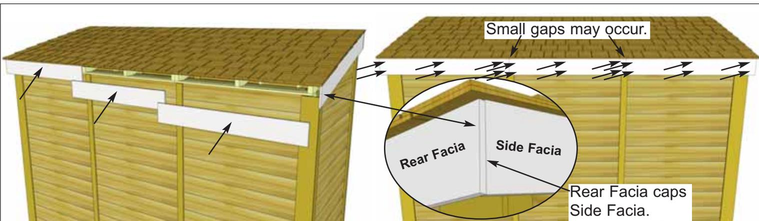
**64.** Attach **4S & 4T - Rear Facia** onto rafter ends as per **Steps 61 - 63**. Small gaps may occur between the Center and Left/Right Facia, these will be covered by Facia Detail Plates in **Step 65**. Rear Facia will cap the side Facia. Attach Rear Facia to rafter ends with **2 - 1 1/2" Finishing Nails** per rafter end.
