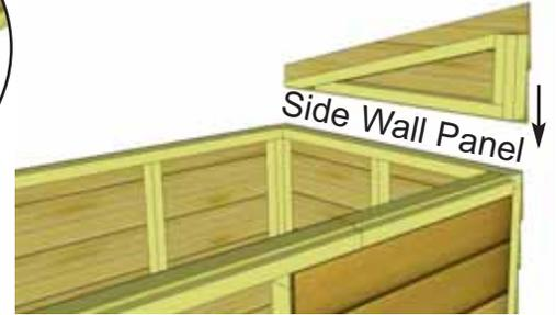
**16.** Position **2F - Top Triangular Siding Piece** onto **2G - Angle Wall Extender** and align as shown above. Attach with **3 - 1 1/2" Finishing Nails** to top frame of extender wall. There are left/right top siding pieces. Use rough surface side out. Place finished wall extender on side wall panel frame. Complete both sides now.
