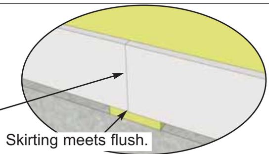
**45.** Attach **4B - Front Bottom Skirting** with **4 - 1 1/2" Finishing Nails** per piece as per **Steps 43 - 44.**
