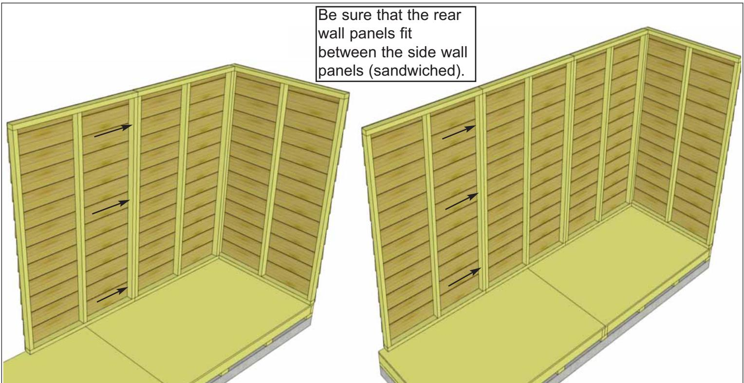
**11.** With the corner wall attachment complete, position a second rear wall panel in place so bottom 2x3 wall framing is sitting flush with outside floor joists. Wall siding should overhang floor by approximately 1/2". When positioned correctly, attach both side wall panel studs together as per **Step 10**.
