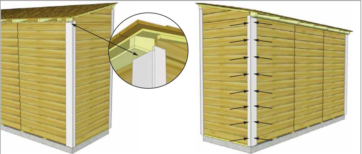
**58.** To complete trimming out rear corners, locate **4N & 4O - Rear Corner Trims**. Align and attach as per **Step 57**.
