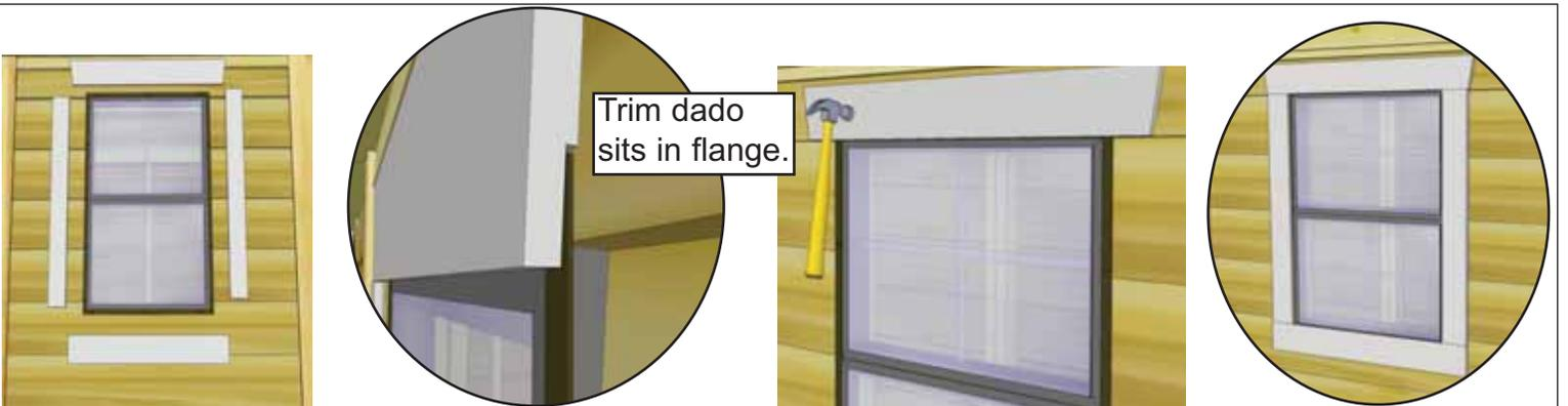
**68.** Position **4X - Window Trim** around window doing a dry run first and attach with **4 - 1 1/2" Finishing Nails** per piece. Window trim has a small dado on reverse face. Outside flange of window will roughly sit in the dado to give a better fit. Complete both windows the same.
