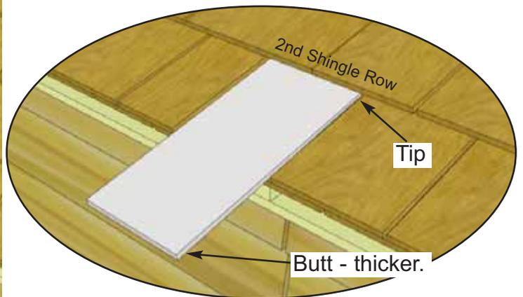
**37.** To cover roof seams, slide a **3I - Filler Shingle** up and underneath second shingle row. Push or bang filler carefully with a hammer until evenly spaced and butt is even with other 1st row of shingles. Do first filler shingle on both seams.
