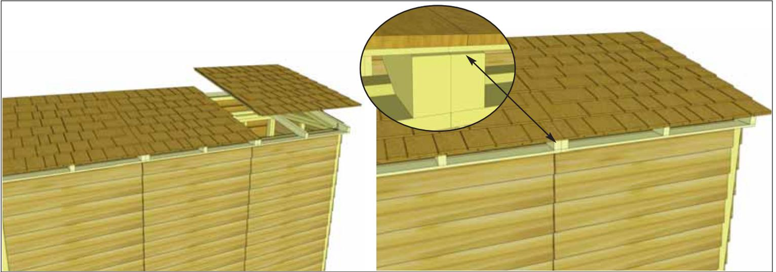
**35.** Position other side roof panel onto rafters as per **Steps 32 - 34.**
