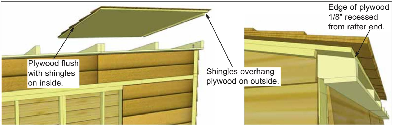
**32.** Correctly orientate **3G - Side Roof Panel**, with shingles overhanging plywood on the side of the shed and flush with plywood toward the center of the shed. Place on rafters with rear edge of plywood just about flush with rafter ends but just slightly recessed. Doing so allows rear fascia to sit better.
