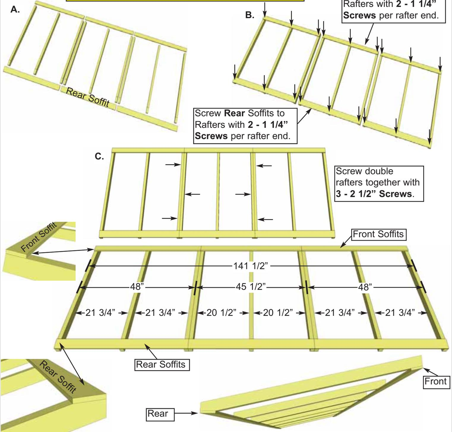
**25.** Locate **3A - Rafters**, **3B & 3C - Front Soffits** and **3D & 3E - Rear Soffits**. Lay out on level ground and assemble as shown above in Illustrations **A** through **C** below. Attach Soffit Boards flush to end of outside rafters. Attach Front Soffits with **2 - 1 1/4" Screws** per rafter end. Attach Rear Soffits with **2 - 1 1/4" Screws** per rafter end.
