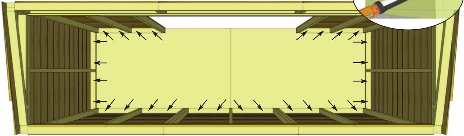
**24.** To complete Wall Section, attach bottom 2x3 wall plates to plywood floor with 2 - 2 1/2" Screws per wall section. Prior to securing, make sure wall panels are aligned correctly on the floor. Refer to **Step 9**. Wall siding should overhang floor while 2x3 wall plates should sit flush with floor.
