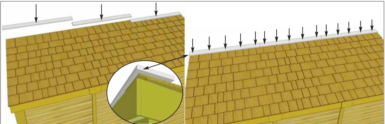
**66.** Position **4V - Roof Ridge Board** at the rear of roof to cap off shingles and facia. Ridge Boards should meet on seam of roof panels. When aligned correctly, attach with **5 - 1 1/2" Finishing Nails** per piece.
