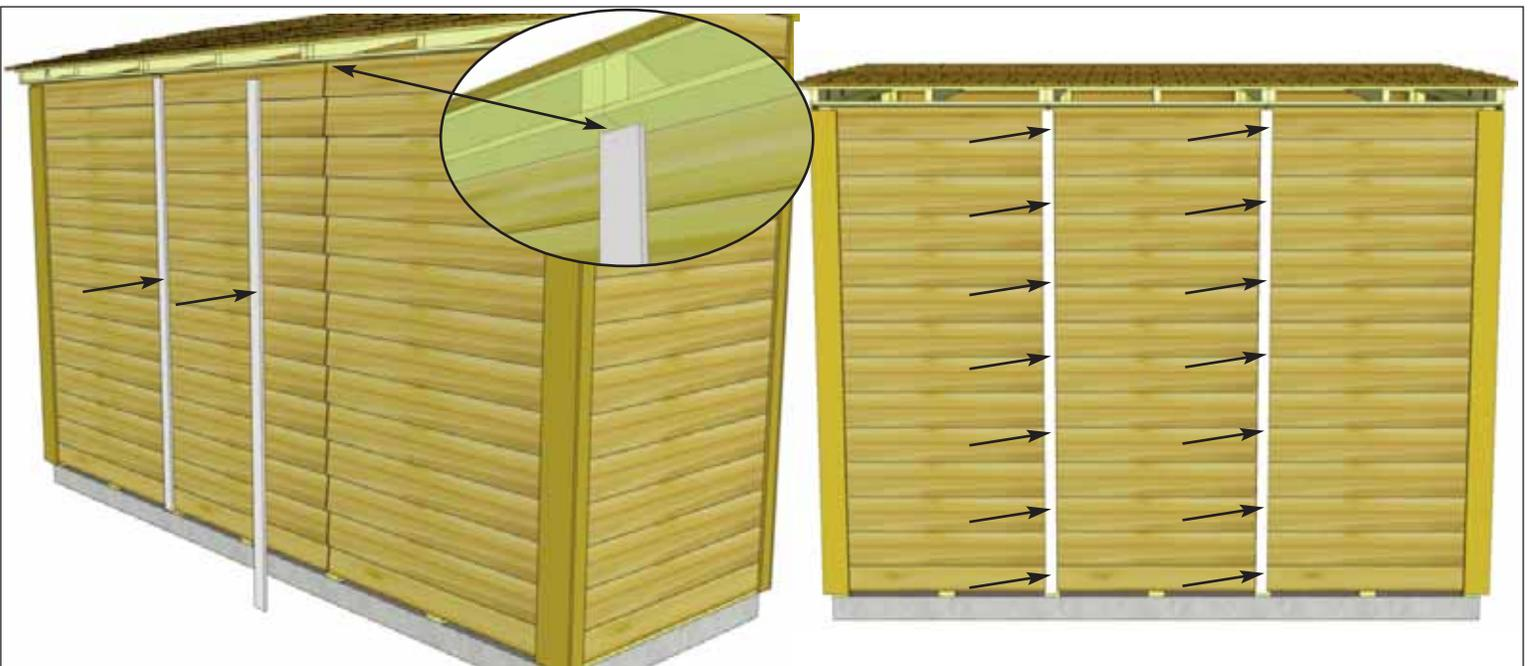
**59.** Attach **4P - Rear Middle Trims** where wall panels come together at rear seam. Attach with **8 - 1 1/2" Finishing Nails** aligning tight underneath soffit and center on seam.
