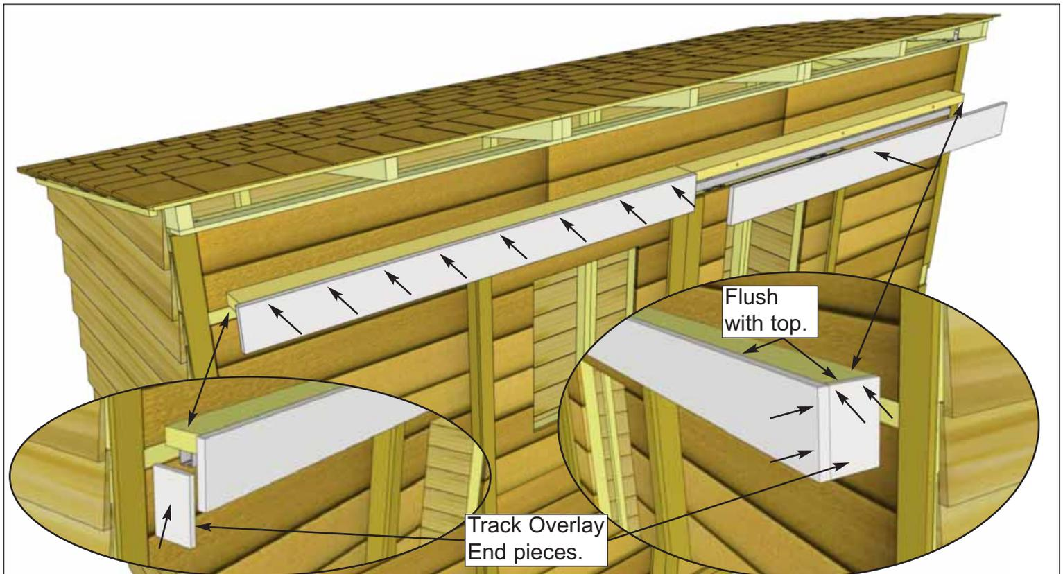
**55.** Position both of **4KB - Track Overlay - Front** onto the edge of the Overlay Top so they meet at the center. Ends of the Overlay Front will protrude 1/2" past the ends of the Overlay Top. Attach with **8 - 1 1/2" Finishing Nails** per piece. Next, attach **4KC - Track Overlay - Ends** as shown above with **4 - 1 1/2" Finishing Nails** per piece.
