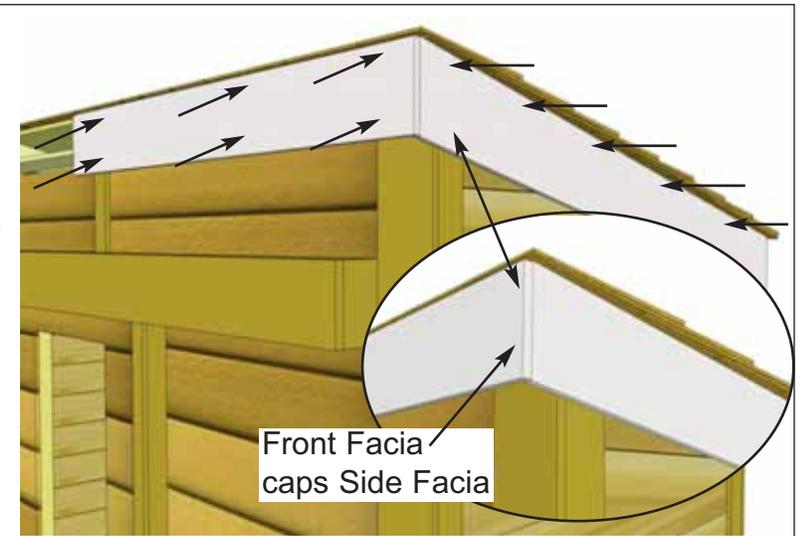
**61.** Locate one **4R - Side Facia** and one **4S - Front Facia** and align in front corner. Position facias underneath roof panel, doing a dry run first before securing. Front Facia goes against rafter ends and Side Facia goes against Facia Nailing Strip. Align so the Front Facia caps the Side Facia. Attach Front Facia with **2 - 1 1/2" Finishing Nails** per rafter end. Attach Side Facia to the Facia Nailing Strip with **5 - 1 1/2" Finishing Nails**.
