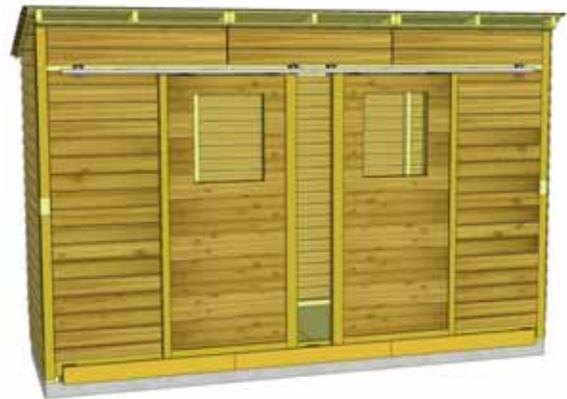
**52.** Locate **4HA - Door Track Covers**. Lineup so Track Covers are flush with Door Stops. This creates an enclosure so doors can not slide out of the track. Secure each piece of Track Cover with **4 - 2 1/2" screws**.
