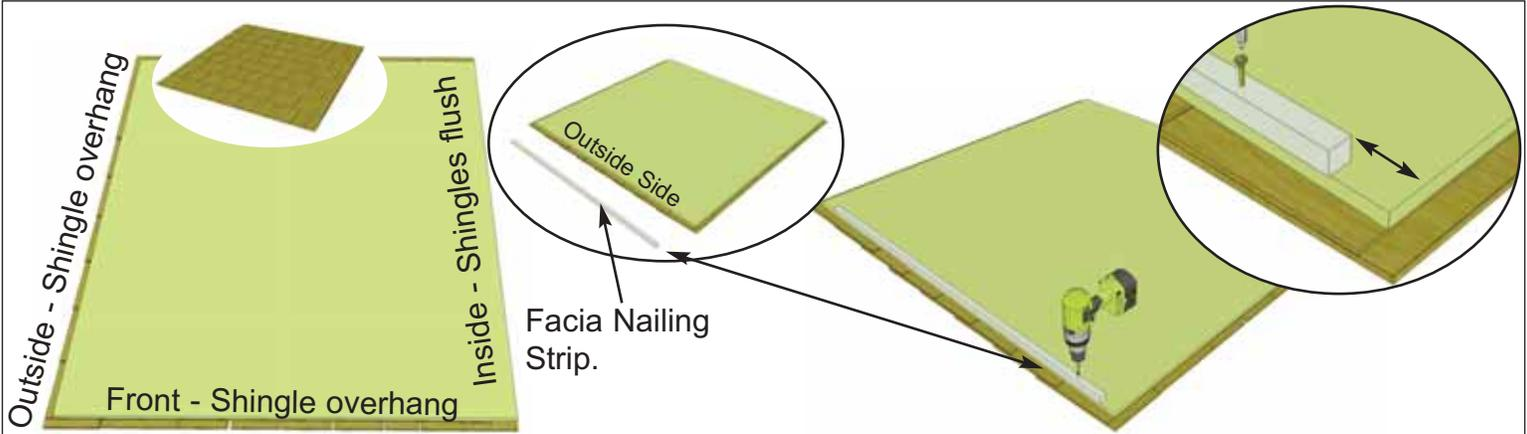
**31.** Carefully flip Roof Panels over so plywood sheathing is facing up. Center **3F - Facia Nailing Strips** onto outside of each panel flush with plywood. Attach with **4 - 1 1/4" Screws** evenly spaced. The Facia Nailing Strip provides for a greater nailing surface later when you attach side facia.
