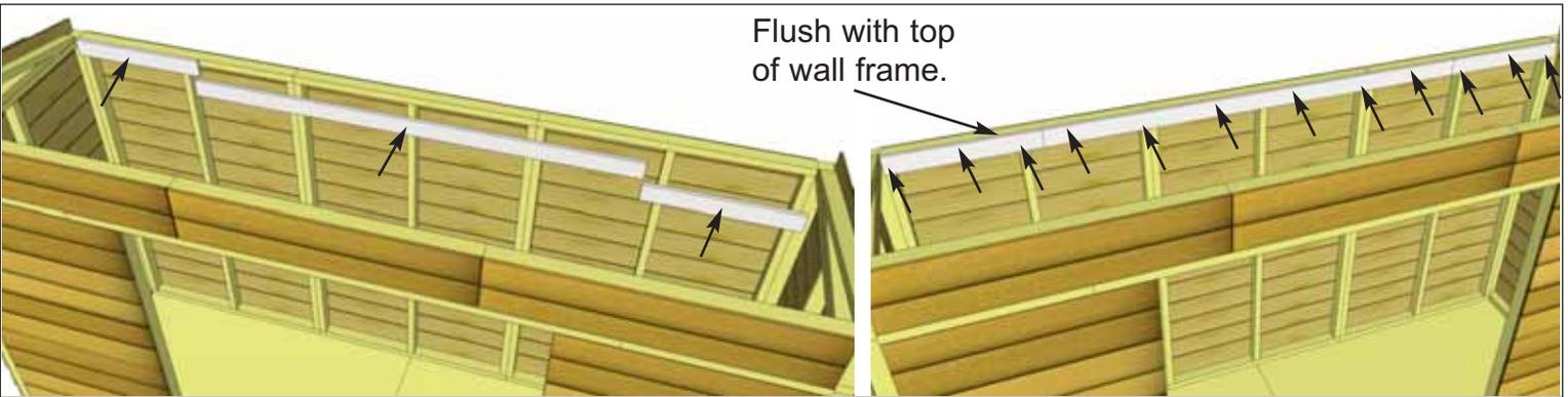
**22.** Align **2J & 2K - Horizontal Wall Cleats** flush with top of Rear Wall framing. Attach with **3 - 1 1/4" Screws** per short cleat and **6 - 1 1/4" Screws** on the long cleat.
