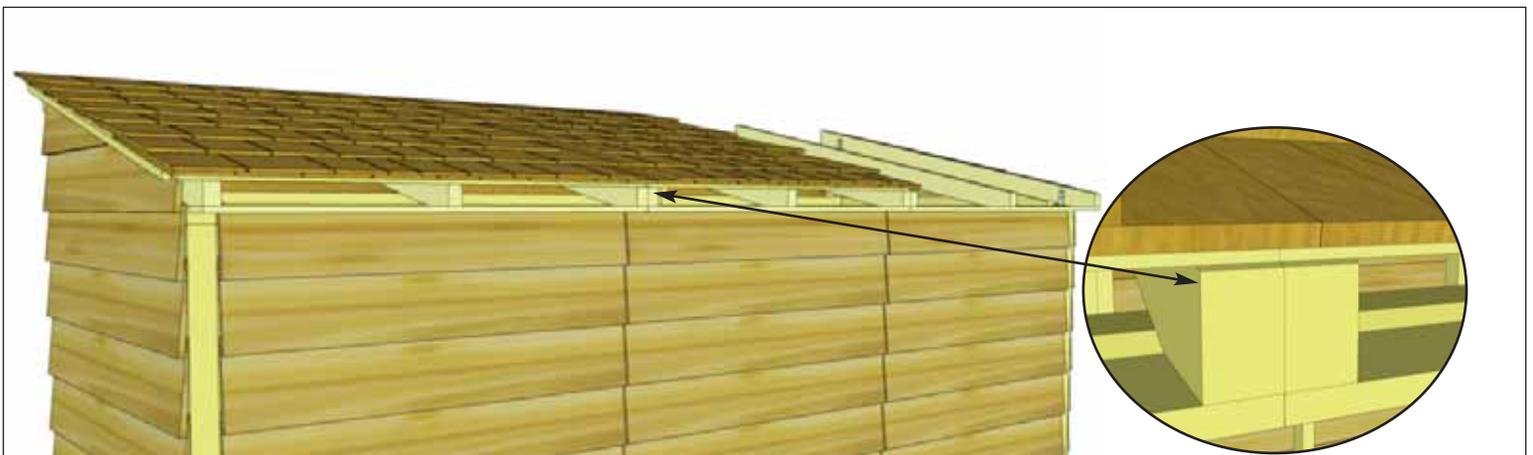
**34.** Align plywood of center roof panel so it is tight against the plywood of the side roof panel. Spacing should be even front and back.
