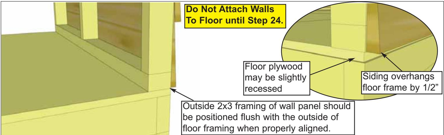
**9.** The side wall panels will sit even with the floor frame and the rear panels will be sandwiched between the side wall panels. The floor plywood may be slightly recessed.
