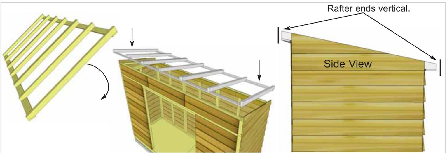
**26.** Carefully flip completed Rafter Section over so Front Soffit is facing the front and place on GardenSaver walls. **Note:** Double check that your Rafter Section is positioned correctly by ensuring the ends of the Rafters are sloped vertically as shown above.
