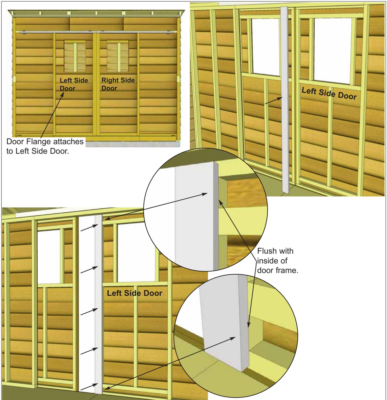
**53.** Position **4J - Interior Door Flange** on the rear of the left side door (when viewed from the front of the shed). Ensure flange is flush with the inside of the door frame and attach with **5 - 1 1/4" Screws**.
