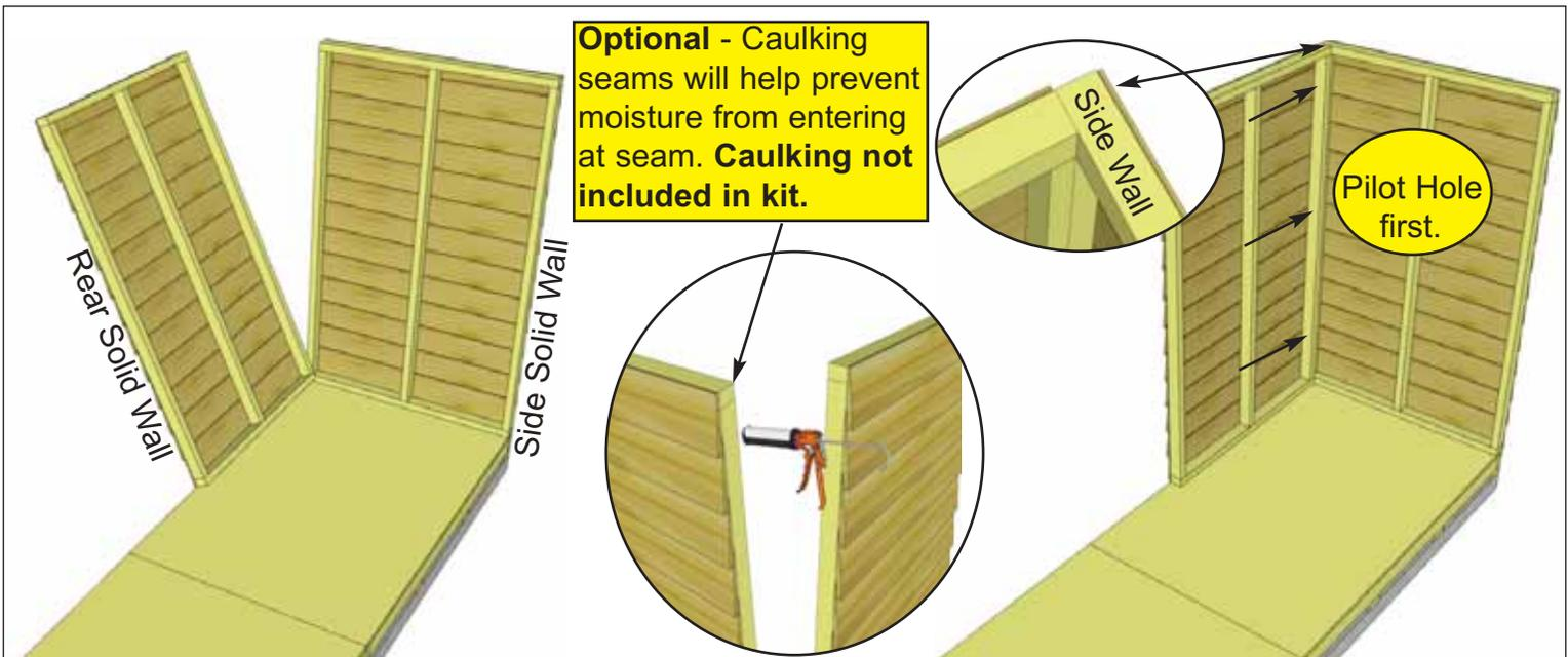
**10.** Position rear solid wall into place on plywood floor. Butt both vertical wall studs of side and rear walls together and attach with **3 - 2 1/2" Screws**. Screw at the bottom, middle and top of stud to secure properly.
