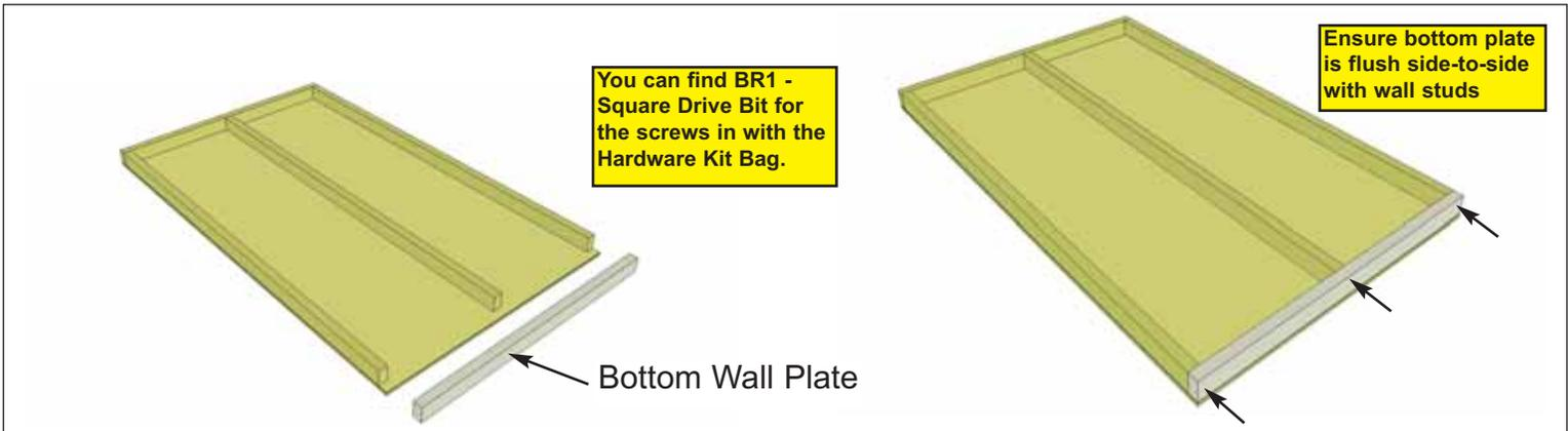
**7.** Carefully lay **2AA - Side/Rear Wall Panels** face down. Position and attach **2AB - Bottom Wall Plates** to bottom of wall studs of each wall panel with **3 - 2 1/2" Screws**. Position so plates are flush with framing. Complete 4 remaining solid walls.
