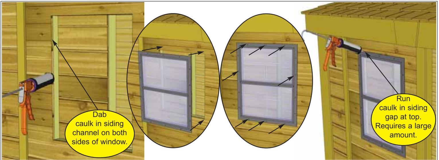
**67.** Locate **4V - Window Inserts**. Before installing, dab caulk in siding channel on both sides of window opening. This will prevent water from getting in behind window. Position window in cavity and secure with **8 - 1 1/4" Screws**. Caulk gap between siding and window at top. This requires a large amount of caulking but is important to fill. Later, Window Trims will be installed to hide caulking. Complete second Window Insert the same.
