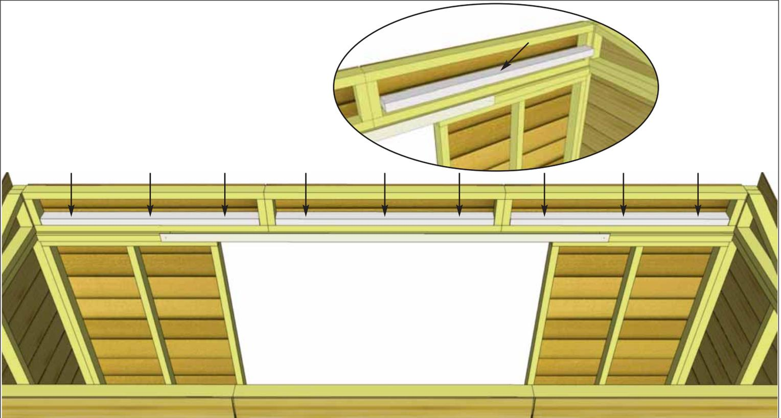
**21.** With Extender Walls attached, position **2I - Extender Wall Cleats** in the lower section of each Extender Wall. Attach with **3 - 2 1/2" Screws** per cleat.
