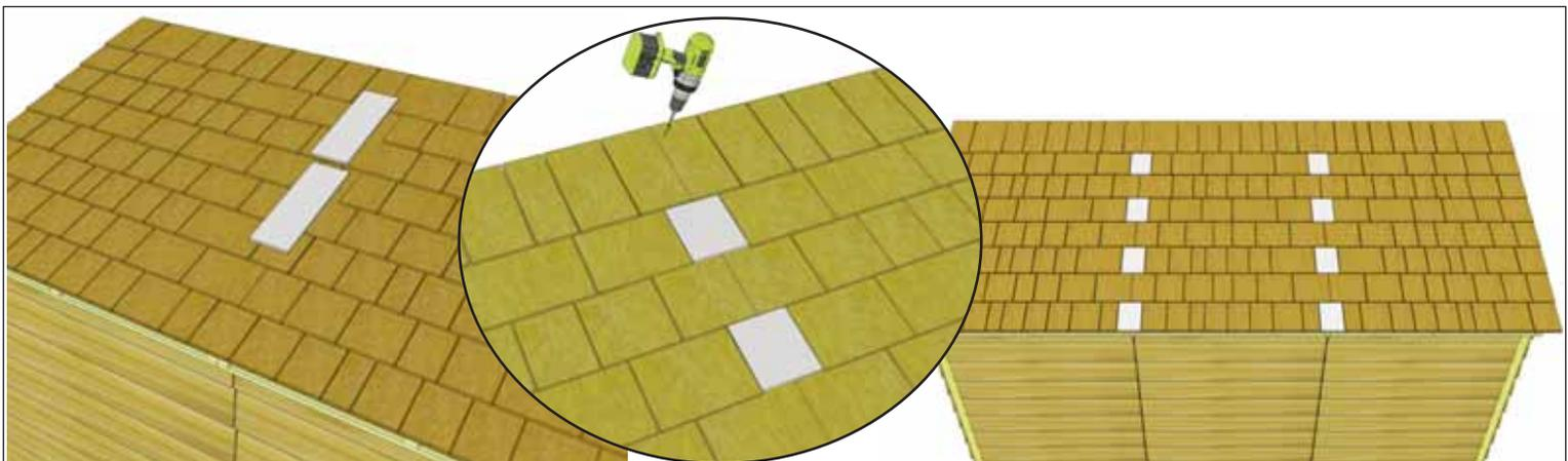
**40.** Slide 3rd and 4th **Filler Shingles** up and underneath appropriate shingle rows and follow **Steps 37 - 39** to align and attach. On last filler, screws will get covered by Roof Ridge Board (4 1/2" wide).
