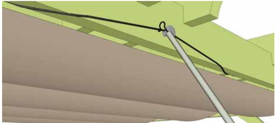
**14.** Extend and contract the canopy several times with pull handle. When extending or contracting the canopy, **pull** firmly in one continuous motion to prevent wings from binding.
