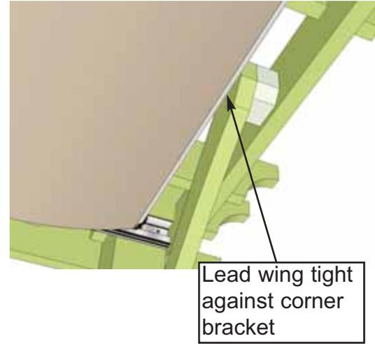
**13.** Pull canopy out using pull handle on lead rope. Fully extend canopy until canopy cannot extend further. Follow **Step 12** to position and attach wing anchor knob to outside girder.
