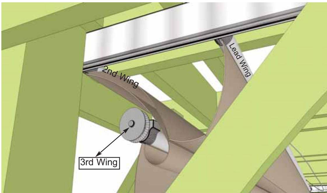
**9.** Continue to feed wings into the track until all wings are installed.
