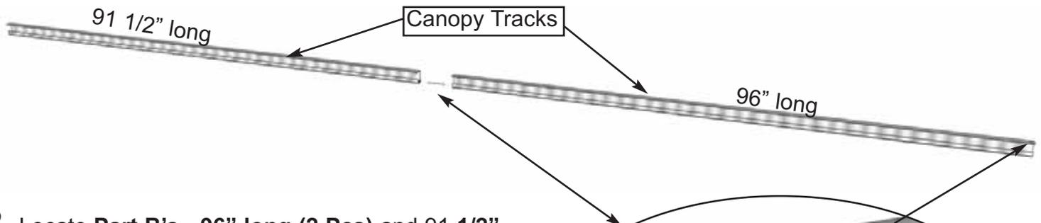
**2.** Locate **Part B's - 96" long (2 Pcs)** and **91 1/2" long Canopy Tracks (2 Pcs)** as well as **4" long x 1/4" diameter Plastic Track Connector (2 Pcs)**.
