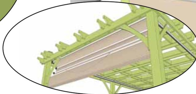
**8.** Push Lead Wing slightly ahead on track. Wings can roll out of track until **D - Aluminum Wing Stop (2 Pcs.)** are installed so be careful. Lift and feed 2nd Wing into track and push wing slightly forward.
