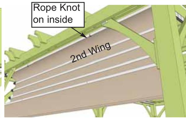
**7.** Before feeding **Part C - 133" long Aluminum Wings (8)** with **Canopy** into track, make sure canopy fabric is facing the correct direction. First, locate Lead and Anchor Wings in set. Both have a black pull rope attached. Make sure rope knots are facing to the inside and the pull rope is facing to the outside. Starting with the Lead Wing, feed the wing wheels onto the track as shown above. Wheels have springs and compress in and out slightly to fit.
