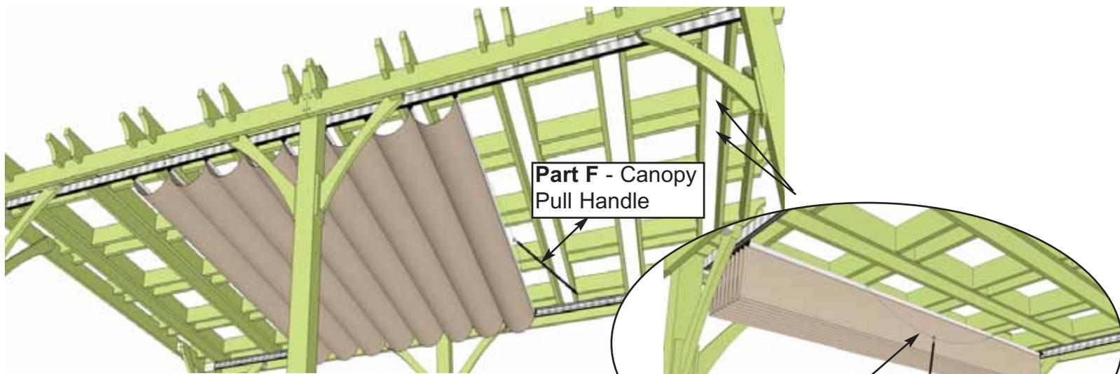
**11.** Using **Part F - Canopy Pull Handle**, pull canopy back and forth a few times to lubricate wheels and track. If wing binds, stop and pull forward until wings are straight and start again. When wings and canopy are tracking well, pull canopy to anchor side of pergola to install **Part D - Wing Anchor Knob**.
