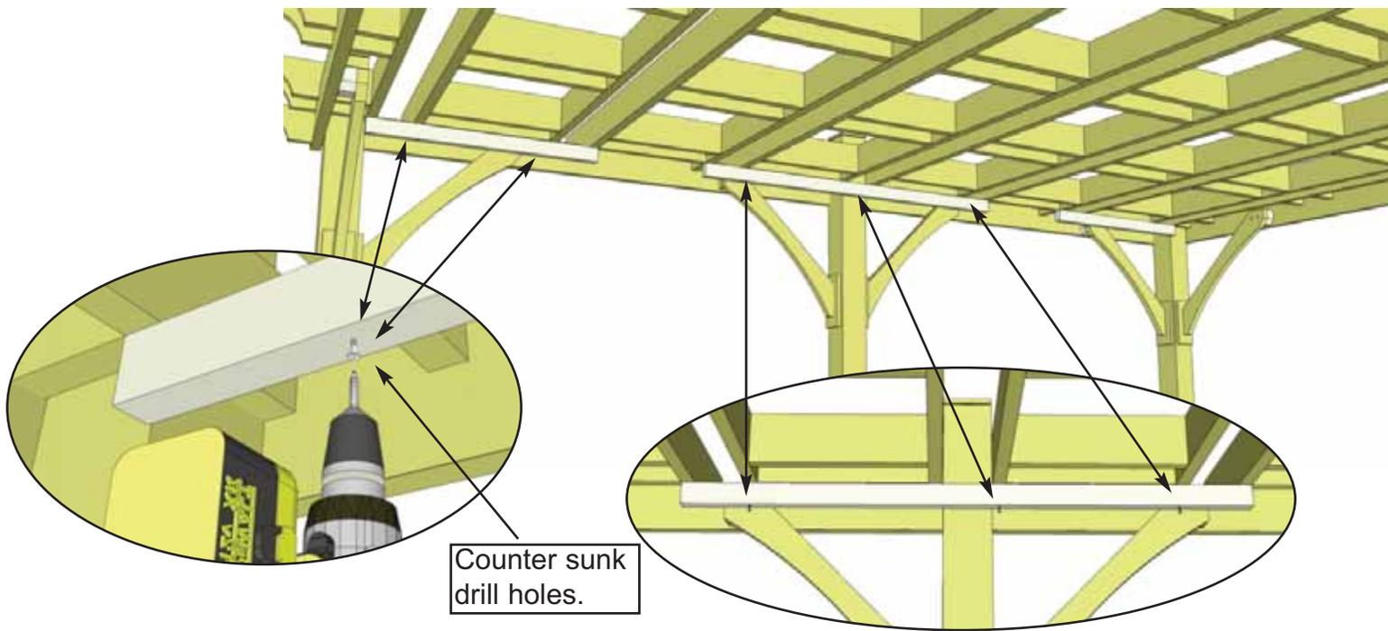
**1.** With a Step Ladder, install **Part A - Canopy Lowering Cleats - 3 pcs Total. (2 pcs. @ 1 1/2" x 3 1/2" x 37 1/4") & (1 pc. @ 1 1/2" x 3 1/2" x 66")**. Attach with **2-3 - 4" Torx Screws**. Cleats will lower the canopy on one side and drain water off the fabric so it doesn't collect excessively. Decide best side for water to drain for your situation. Position cleats underneath pergola joists or blocking as shown above and attach. Cleats are pre-drilled for Torx Screws.
