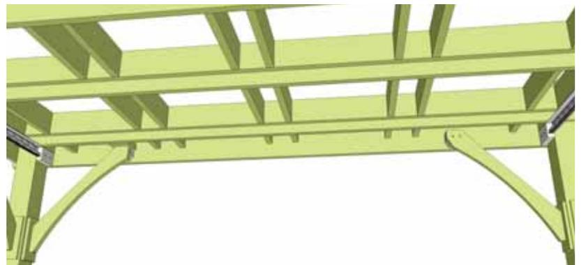
**10.** Install **Part D - 4 1/4" long Aluminum Wing Stops - 2 Pcs.** where track ends and gap exists. Use 2 - 1 1/4" brown screws per stop to install. When removing the wings and canopy in the future, simply remove wing stops and roll wing and canopy out carefully with a helper.
