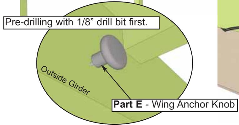
**12.** With canopy pull handle or hand, pull anchor rope up tight so anchor canopy wing is up against inside of pergola bracket. Center Anchor Knob from side-to-side and mark. Before attaching, make sure anchor rope will be snug when slipped over knob. Screw wing anchor knob into outside girder. Pre-drilling with 1/8\" drill bit first.
