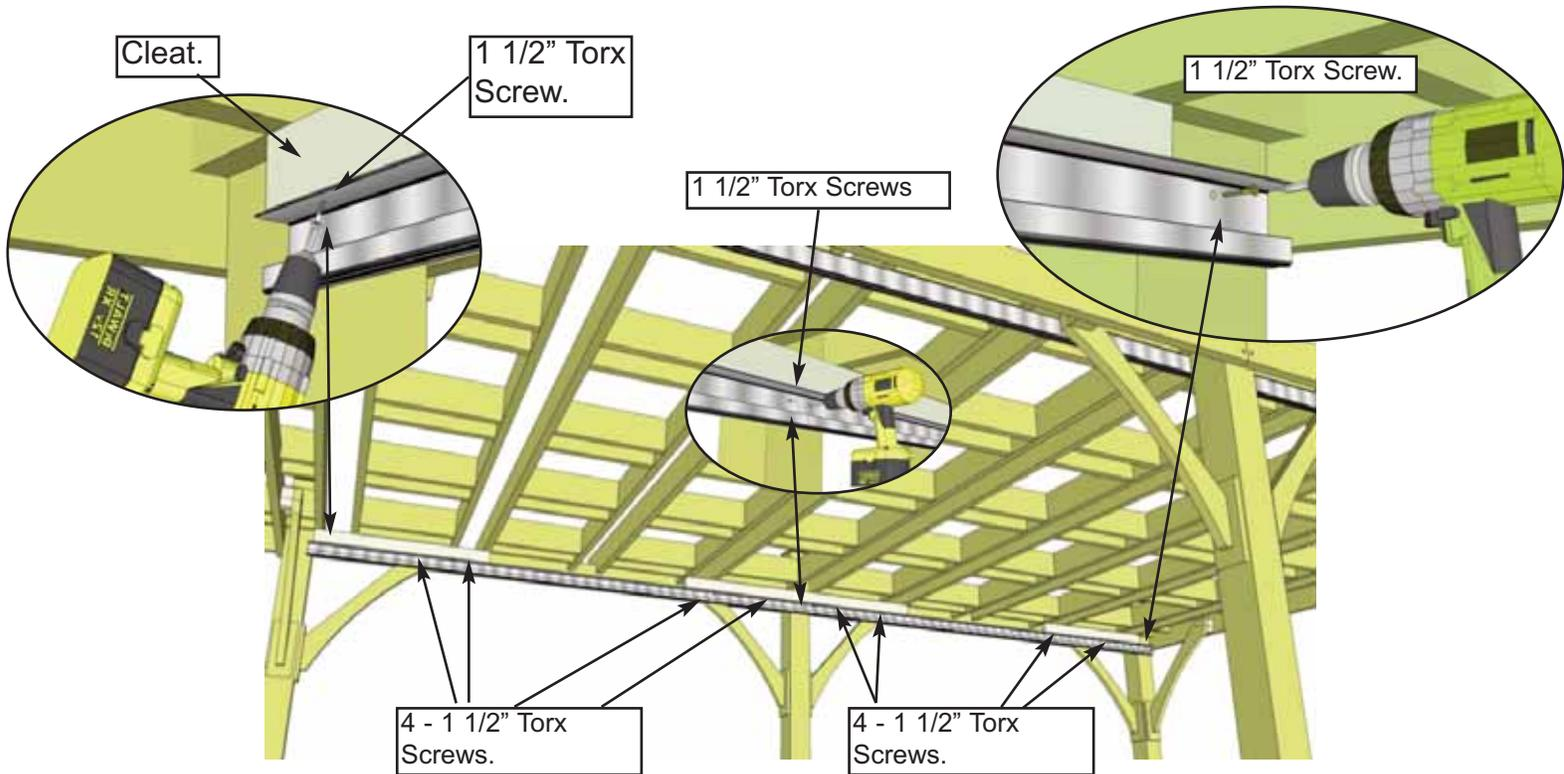
**5.** Align and attach second **Canopy Track** directly underneath lowering cleats as per **Step 4**. Position track flush against post as illustrated above. At mid post, screw track to post with 2 - 1 1/2" Torx Screws. Pre-drill first with 1/4" bit.
