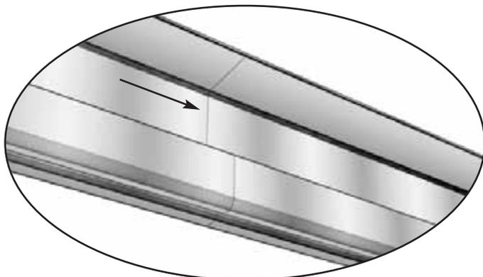
Plastic Connector helps align Track and is not structural. Carefully support connected track when lifting.
