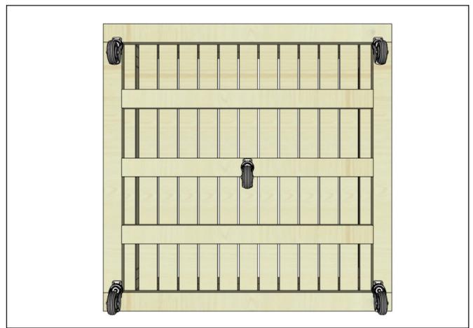
**6. Optional:** Locate Casters. Attach 5 Casters to underside of Floor Frame with **4 - 1 1/4" screws & 4 - washers** per caster. Hardware for Casters comes in the add on package with the casters. Place 1 Caster in each Corner and 1 Caster in the Center of floor frame.
