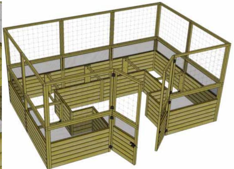
**6.** Locate all four **Black Plastic Hinges (3)** and attach to deer fence frame with **6 - 3/4" black screws** per hinge as shown above. Use 1/8" drill bit to pilot hole shallow holes before attaching to avoid splitting deer fence framing. Open and close door to check door aligned correctly. Adjust as required.
