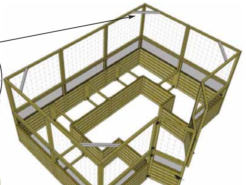
**7.** Attach **Corner Brackets with angle cut ends - (4)** on the inside frames at the top. Use **2 - 2 1/2" Screws** per bracket. Screw on an angle. Pre-drill ends with 1/8" drill bit to prevent wood splitting.
