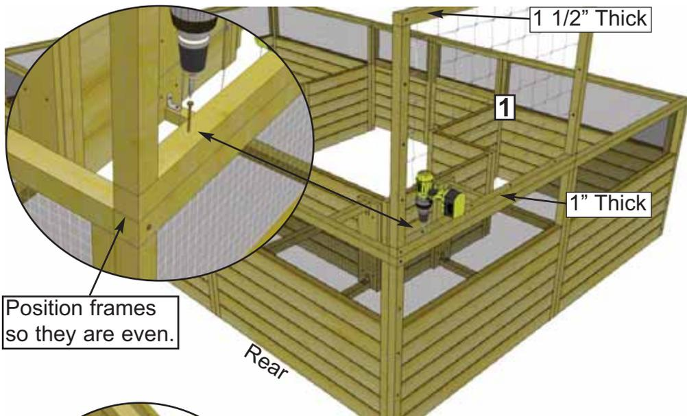
**2.** Starting on the side of the rear corner, position the frame of a **Side Panel (1) - 46" wide x 33 1/2" high** directly on top of the raised bed frame. Screw frames together with **4 - 2 1/2" Screws** as shown on the left. Install panels with the 1 1/2" thick side on top.
