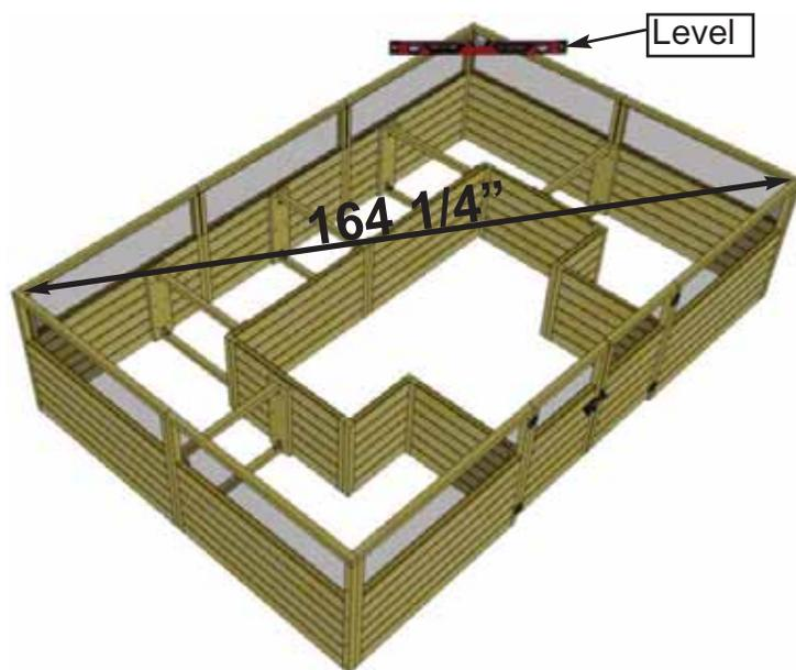
**1.** Prior to installing your Deer Fence Option Kit, confirm your 12x8 Raised Bed is level and square. Measure diagonally inside corner to corner (approximately 164 1/4") in both directions. Adjust as required. Use a level to determine if the tops of the bed frames are sloped and adjust if necessary.
