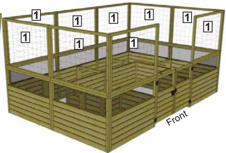
**4.** Position a second **Rear Panel (1) - 46" wide x 33 1/2" high** on top of the rear raised bed frame. Hold both rear deer fence frames together and starting at the top, screw together with **4 - 2 1/2" Screws** as shown above. Screw bottom of frame down to raised bed frame with **4 - 2 1/2" Screws**. Complete remaining side and rear panels attachments following **Steps 2 and 3**.
