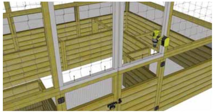
**5.** Locate both **Deer Fence Door Panels (2) - 22 3/4" wide x 33 1/2" high**. Position and install both Door Panels, screwing only from bottom frame into top of raised bed door frame with **3 - 2 1/2" screws** per panel as shown above.
