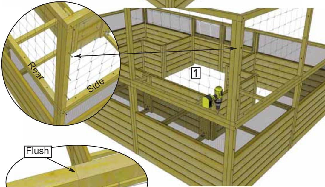
**3.** Position a **Rear Panel (1) - 46" wide x 33 1/2" high** directly on top of the side raised bed frame. Hold both deer fence frames together and starting at the top, screw together with **5 - 2 1/2" Screws** as shown on the left. Screw bottom of frame down to raised bed frame with **4 - 2 1/2" Screws**.
