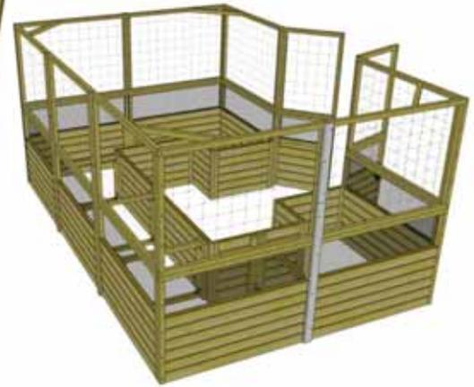
**9.** Position and attach short Vertical Panel Support using **3 - 2" Screws** as per Step 7. Complete remaining rear and side walls.
